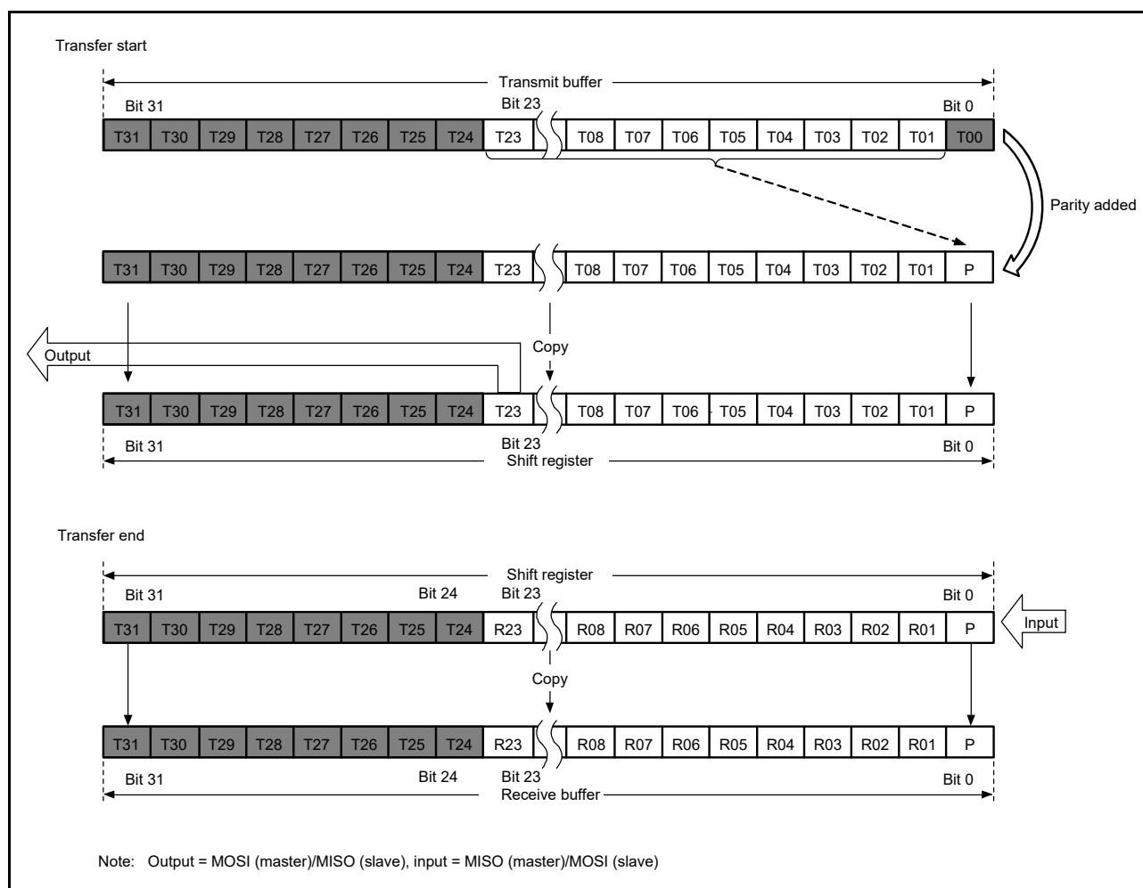
Figure 31.19 MSB-first transfer with 24-bit data and parity enabled
