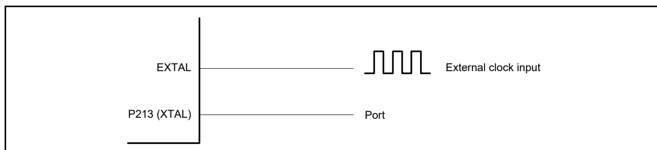
Figure 9.8 Equivalent circuit for external clock
