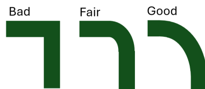
Figure 34. Example of RF trace routing
