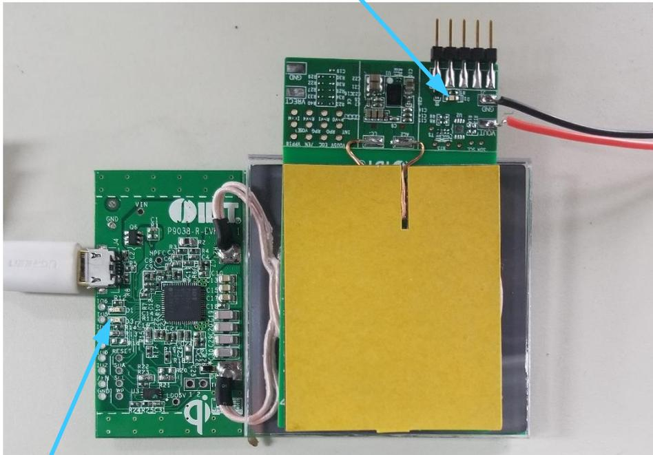
Solder wire leads to GND and VOUT test points to allow measuring VOUT or to apply load
