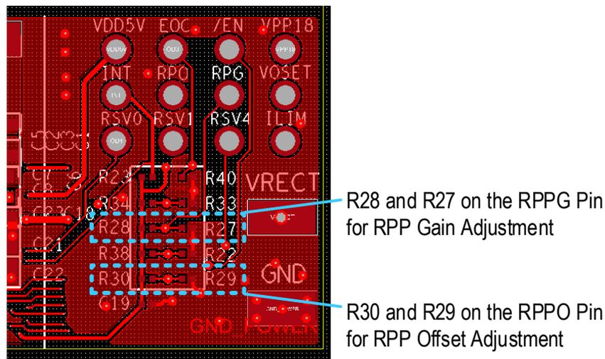
The P9225-R calculates the original received power by multiplying the voltage on the VRECT pin by the coil current, and then it performs initial calibrations to obtain the middle product  $P_{CAL}$ . Then the RPP value is computed using Equation 2:
