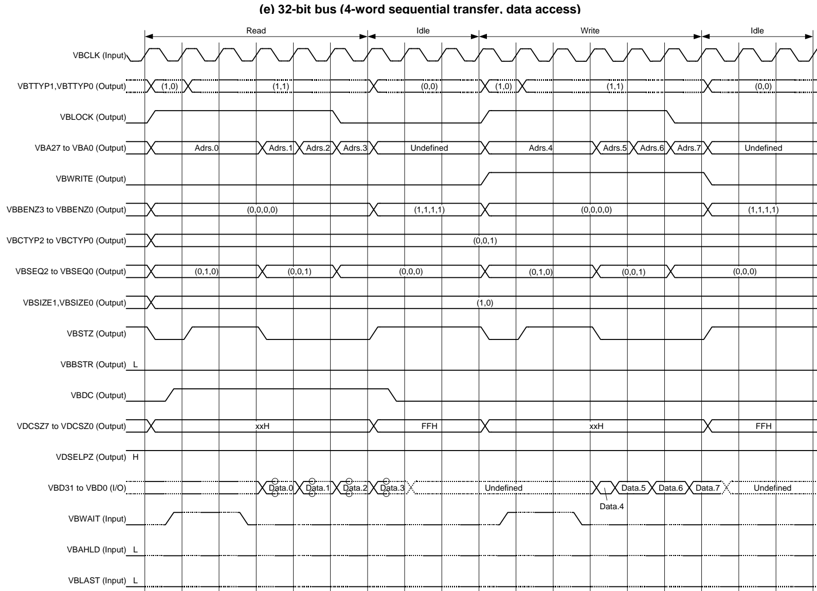
Figure 4-14. Read/Write Timing of Bus Slave Connected to VSB (5/12)
