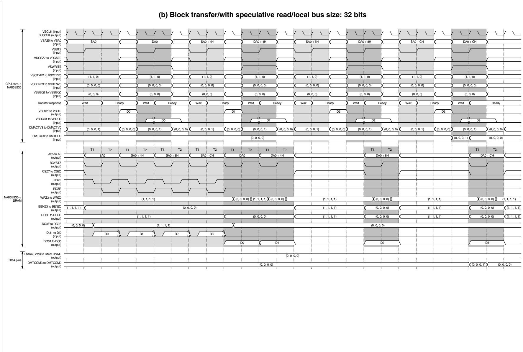
★ Figure 4-14. Example of DMA Transfer Timing (2-Cycle Transfer (Using DMAC with On-Chip CPU Core): SRAM → SRAM) (2/5)
