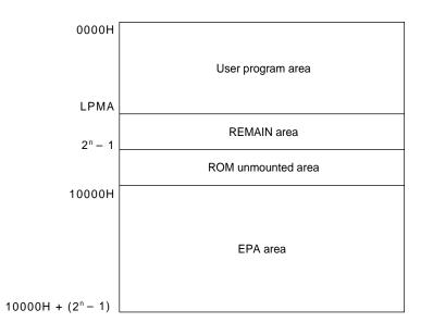
Figure 1-3. Address Space in a 17K Series Segment
