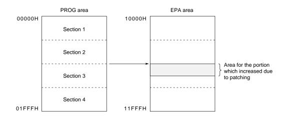
**Example 2.** Section 4 (allocated to the highest address in a segment) is patched, such that section 4 increases in size.
