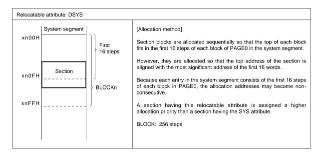
Figure 2-5. Relocatable Attribute (DSYS) and Allocation Method
