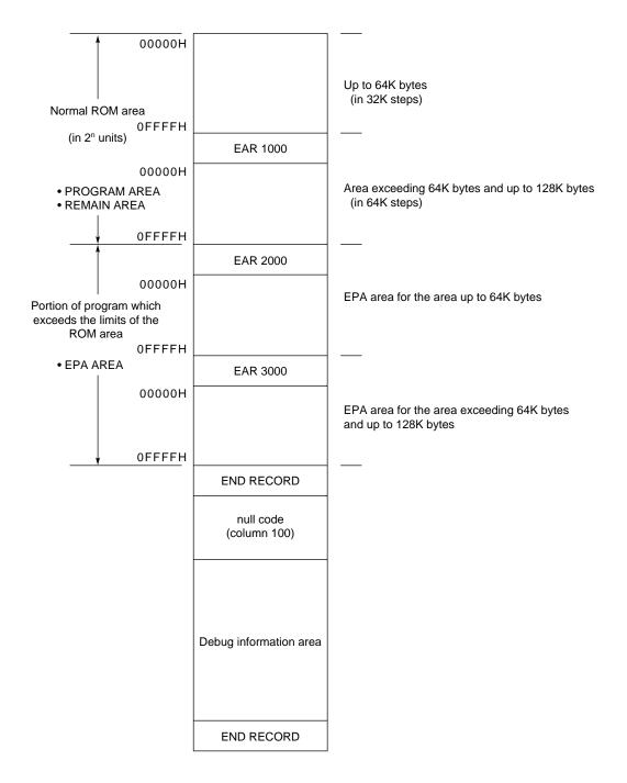
Figure 3-1. .ICE File Code Output Format
