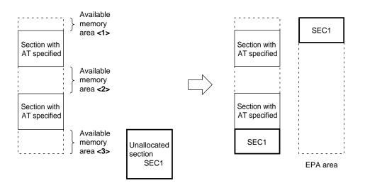
Figure 2-12. Allocating a Section to the EPA Area
