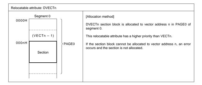
Figure 2-9. Relocatable Attribute (DVECTn) and Allocation Method
