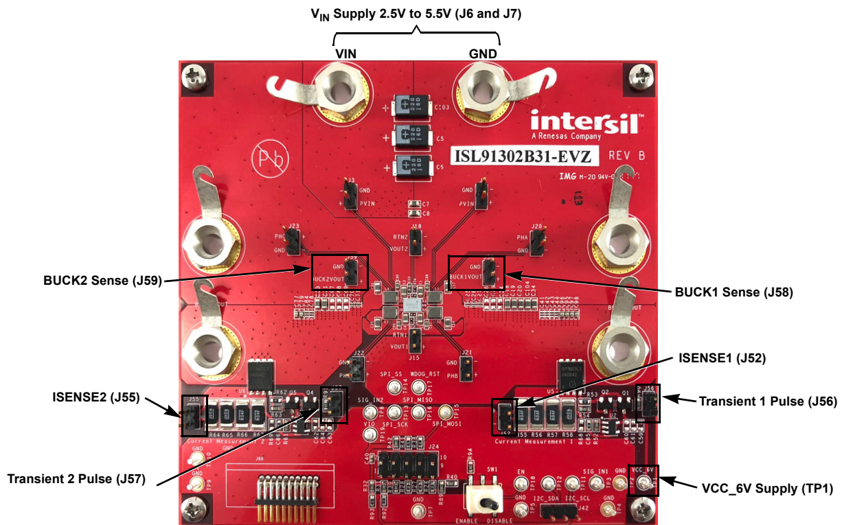
Figure 12. ISL91302B31-EVZ Load Transient Measurement Connections (Top View)
