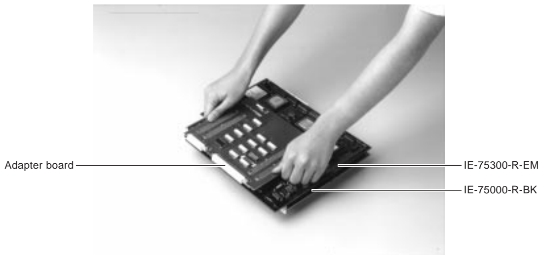
Figure 2-5. Connection of IE-75300-R-EM, IE-75000-R-BK, and Adapter Board
