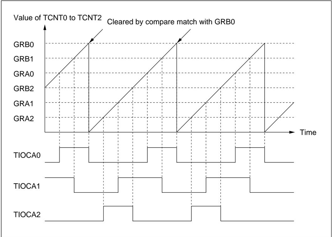
**Figure 10-27 Synchronization (Example)**
