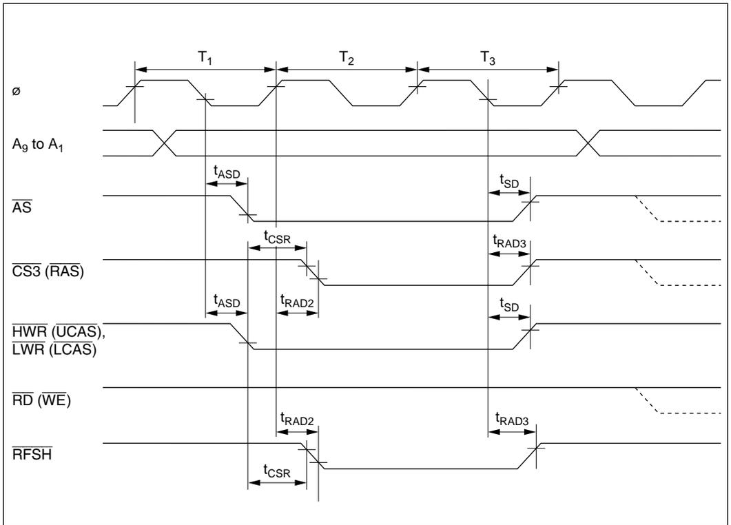
**Figure 18-11 DRAM Bus Timing (Refresh Cycle): Three-State Access**
