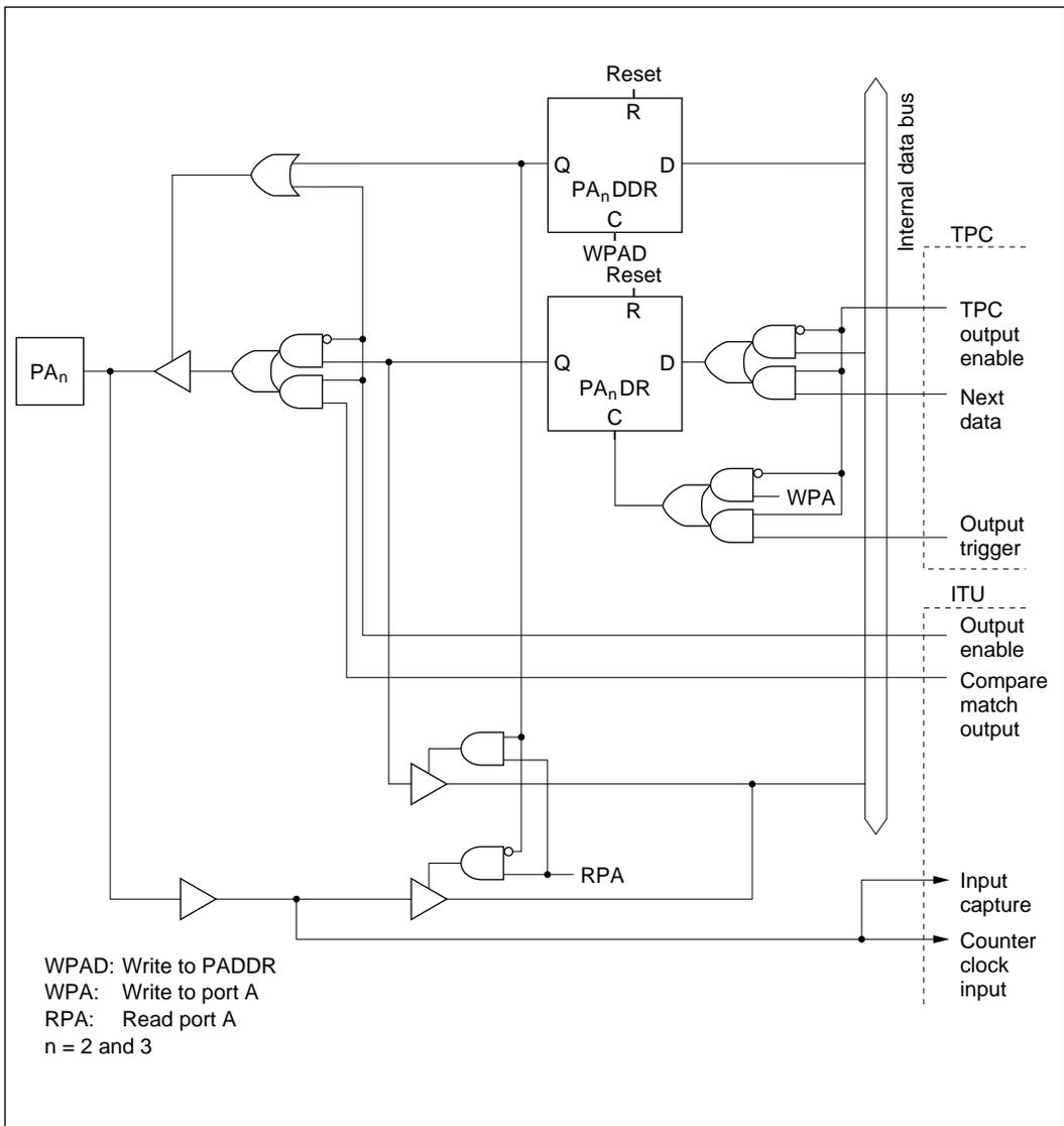
**Figure C-7 (b) Port A Block Diagram (Pins PA<sub>2</sub>, PA<sub>3</sub>)**
