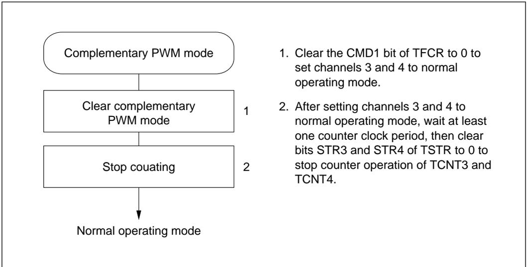
**Figure 10-34 Clearing Procedure for Complementary PWM Mode**
