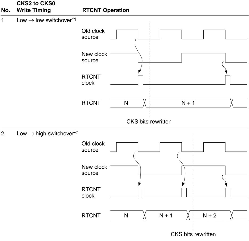
Notes: 1. Including switchovers from a low clock source to the halted state, and from the halted state to a low clock source.
