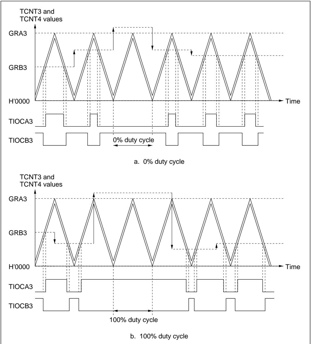
**Figure 10-36 Operation in Complementary PWM Mode
