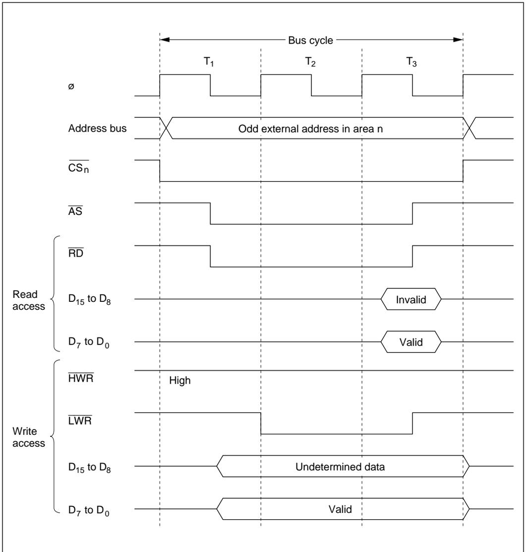
**Figure 6-7 Bus Control Signal Timing for 16-Bit, Three-State-Access Area (2)
