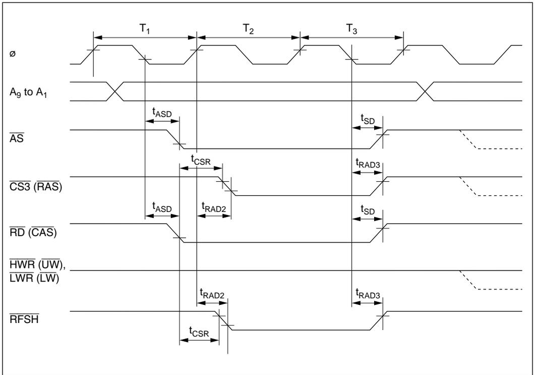
**Figure 18-8 DRAM Bus Timing (Refresh Cycle): Three-State Access**
