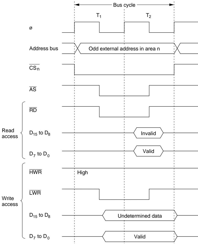
**Figure 6-10 Bus Control Signal Timing for 16-Bit, Two-State-Access Area (2)
