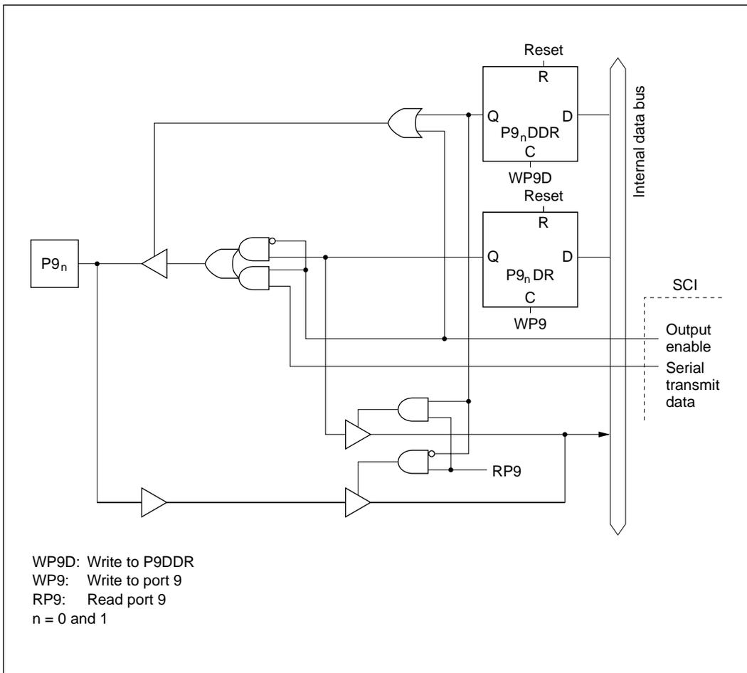
Figure C-6 (a) Port 9 Block Diagram (Pins  $P9_0$ ,  $P9_1$ )
