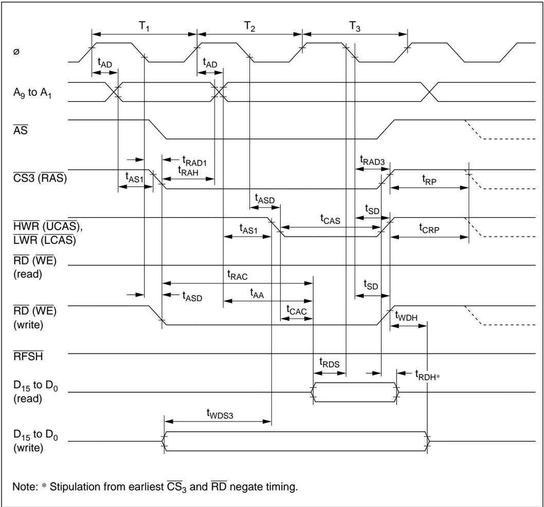
**Figure 18-10 DRAM Bus Timing (Read/Write): Three-State Access**
