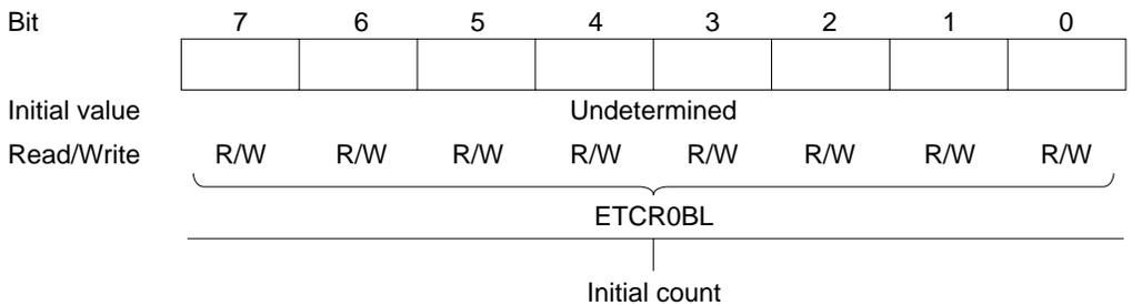
**ETCR0B H/L—Execute Transfer Count Register 0B H/L**
