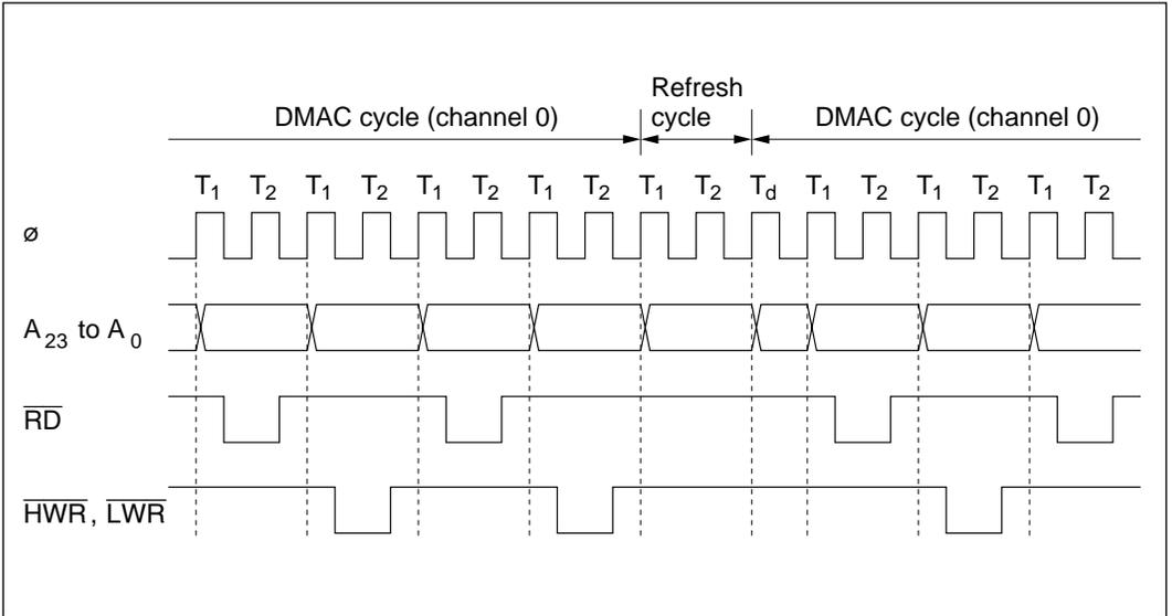
**Figure 8-21 Bus Timing of Refresh Controller and DMAC**
