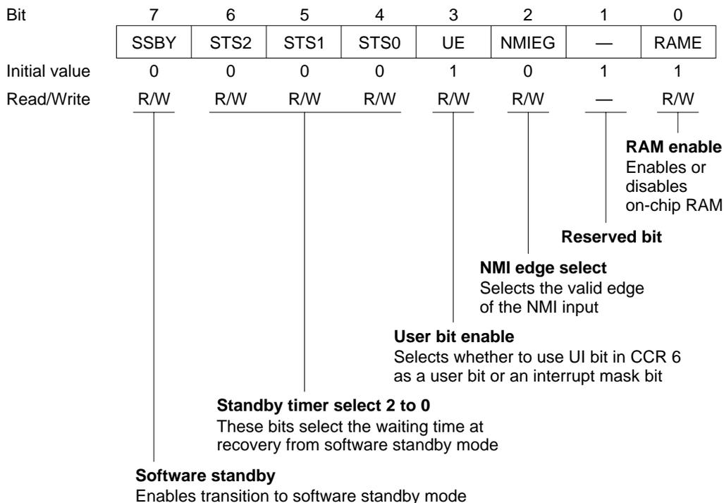
**Bit 7—Software Standby (SSBY):** Enables transition to software standby mode. (For further information about software standby mode see section 17, Power-Down State.)
