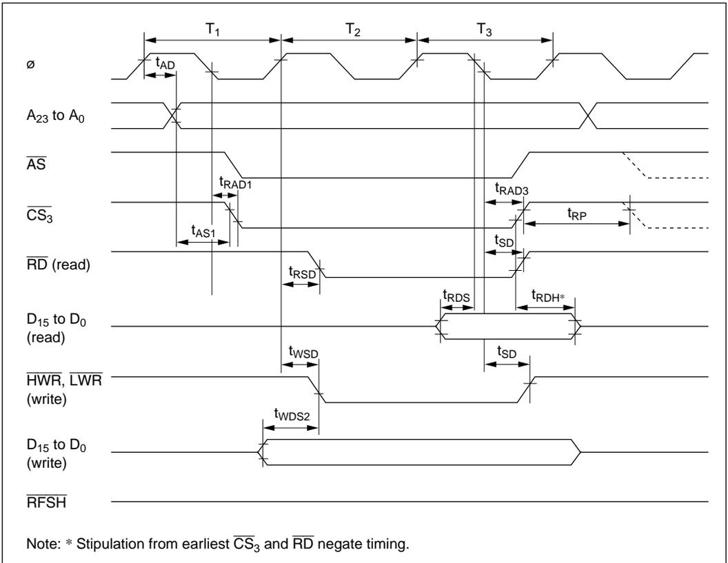
**Figure 18-13 PSRAM Bus Timing (Read/Write): Three-State Access**
