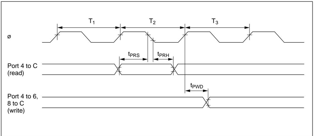
Figure 18-20 TPC and I/O Port Input/Output Timing
