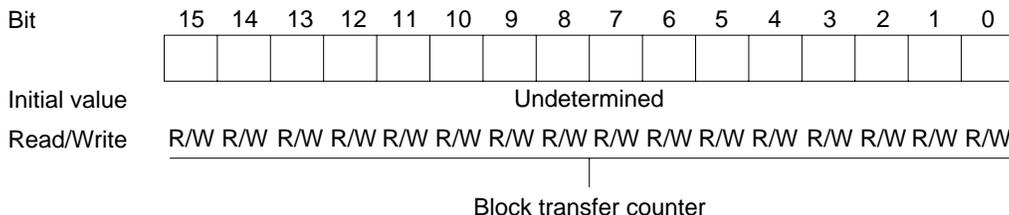
**IOAR0B—I/O Address Register 0B**
