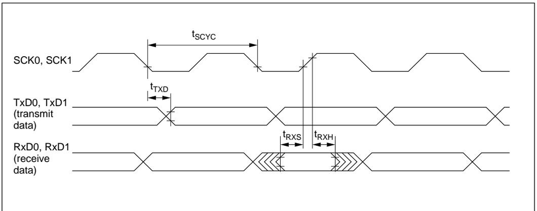
**Figure 18-24 SCI Input/Output Timing in Synchronous Mode**
