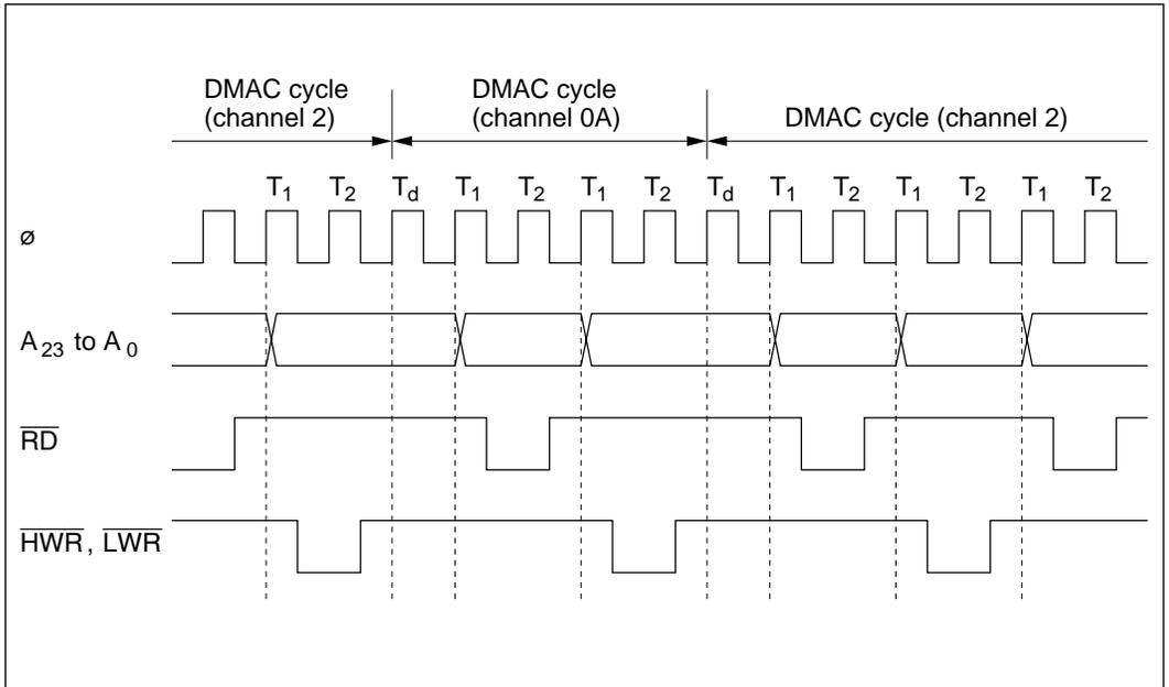
**Figure 8-20 Timing of Multiple-Channel Operations in Different Groups**
