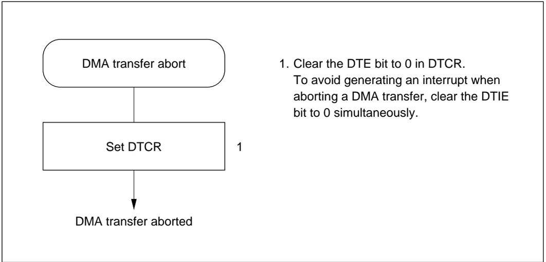
**Figure 8-23 Procedure for Aborting a DMA Transfer**
