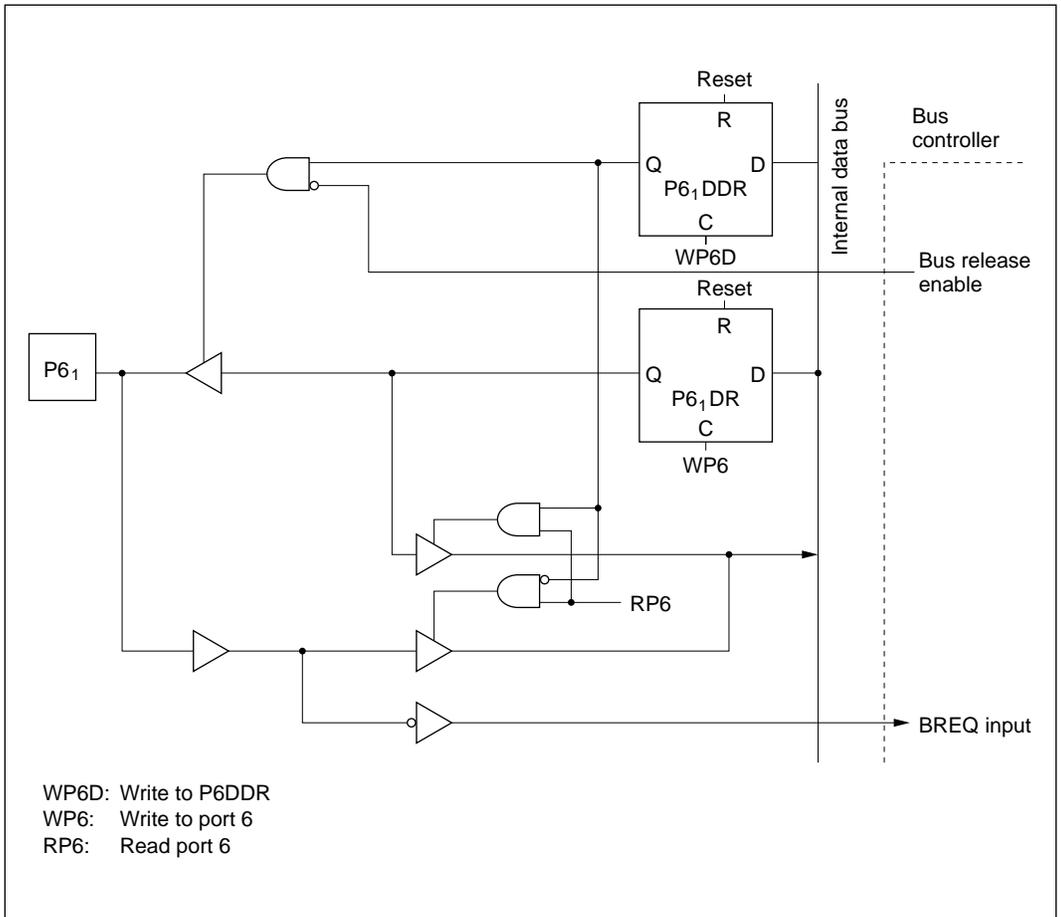
**Figure C-3 (b) Port 6 Block Diagram (Pin P6<sub>1</sub>)**
