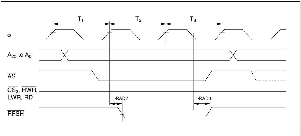
**Figure 18-14 PSRAM Bus Timing (Refresh Cycle): Three-State Access**
