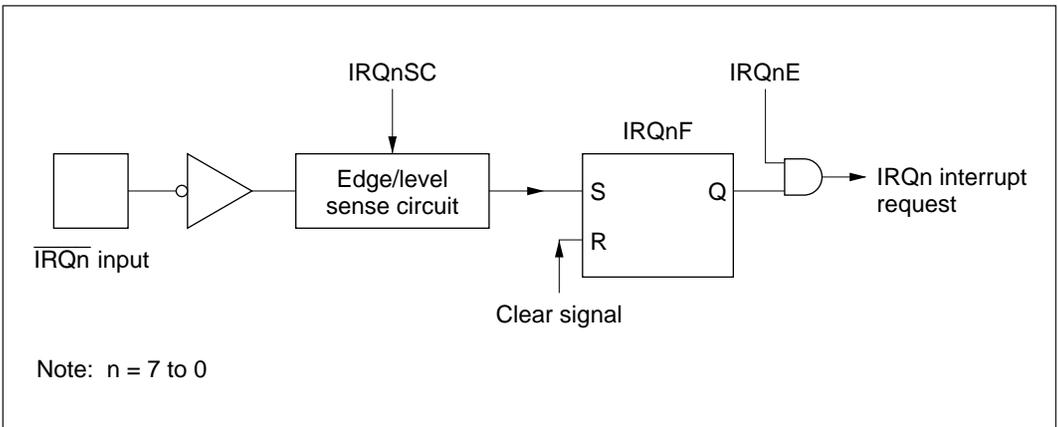
**Figure 5-2 Block Diagram of Interrupts  $IRQ_0$  to  $IRQ_7$**
