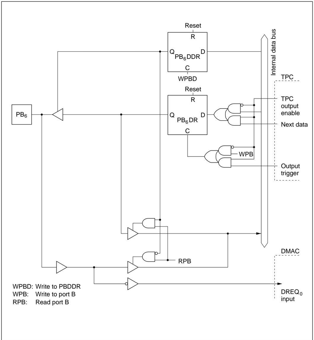
Figure C-8 (c) Port B Block Diagram (Pin PB<sub>6</sub>)
