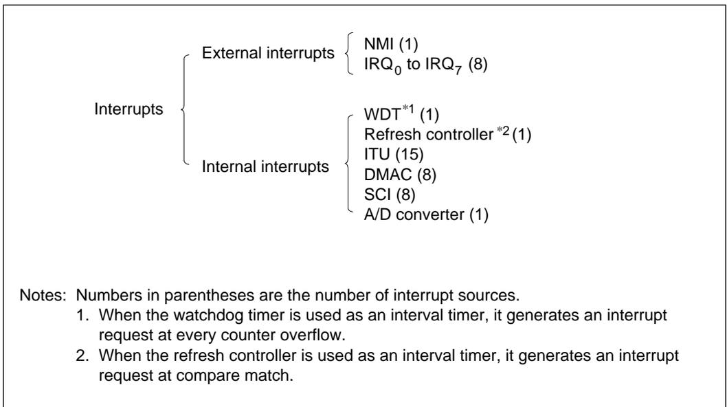
**Figure 4-4 Interrupt Sources and Number of Interrupts**
