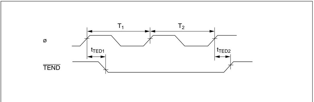
Figure 18-25 DMAC  $\overline{\text{TEND}}$  Output Timing/2 State Access
