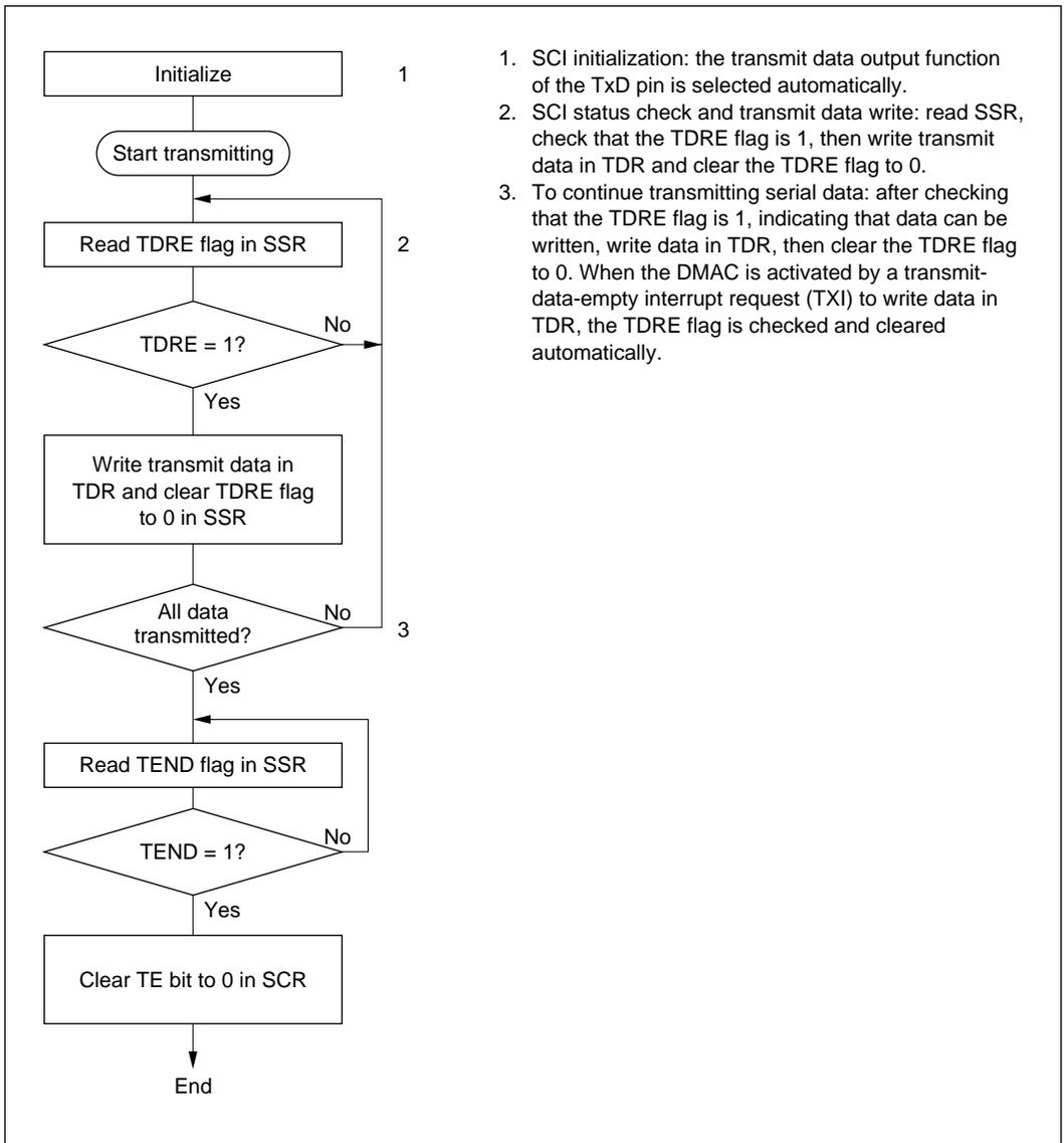
1. SCI initialization: the transmit data output function of the TxD pin is selected automatically.
