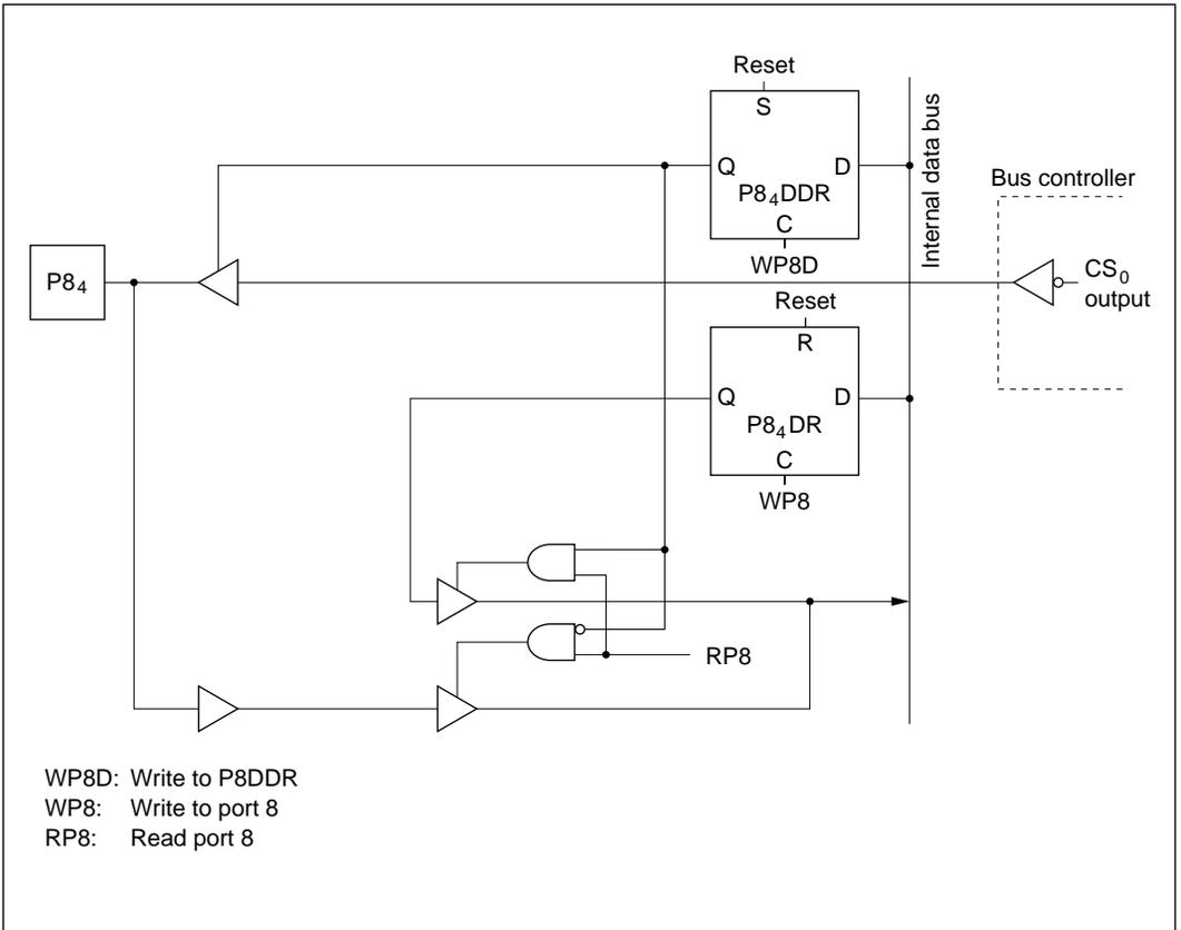
**Figure C-5 (c) Port 8 Block Diagram (Pin P8<sub>4</sub>)**
