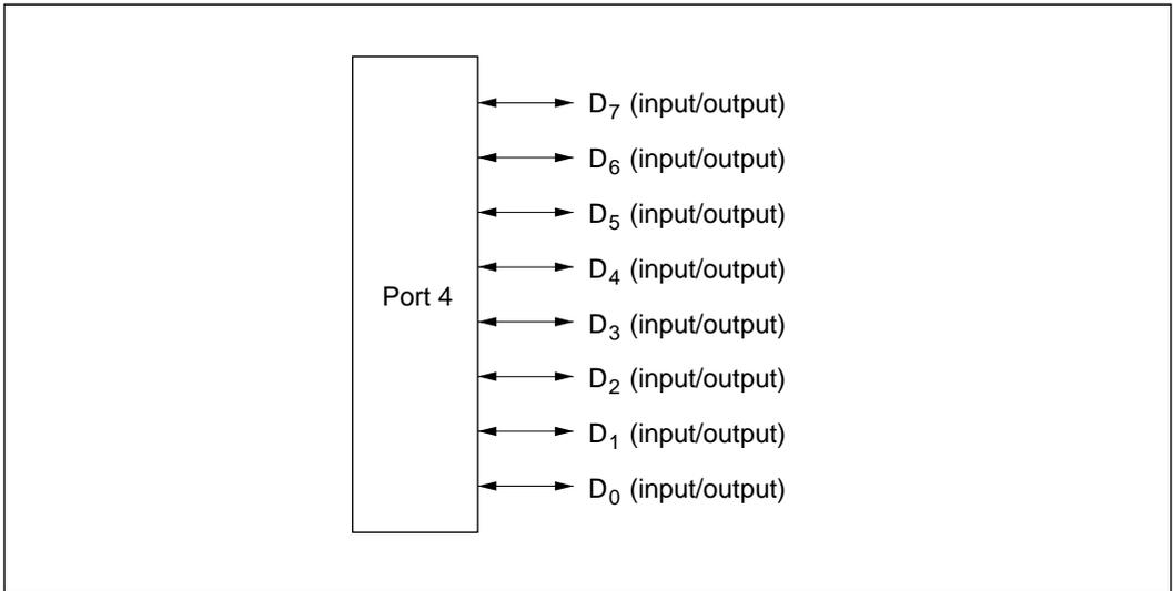
**Figure 9-3 Pin Functions in 16-Bit Bus Mode (Port 4)**
