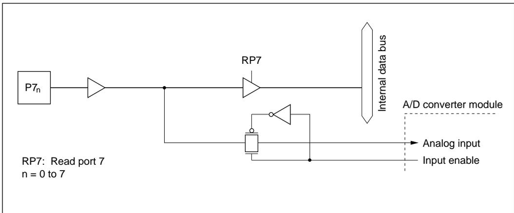
Figure C-4 Port 7 Block Diagram (Pin  $P7_n$ )
