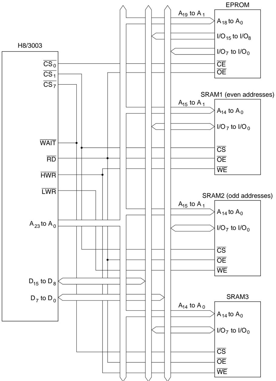
**Figure 6-18 Interconnections between H8/3003 and Memory (Example)**
