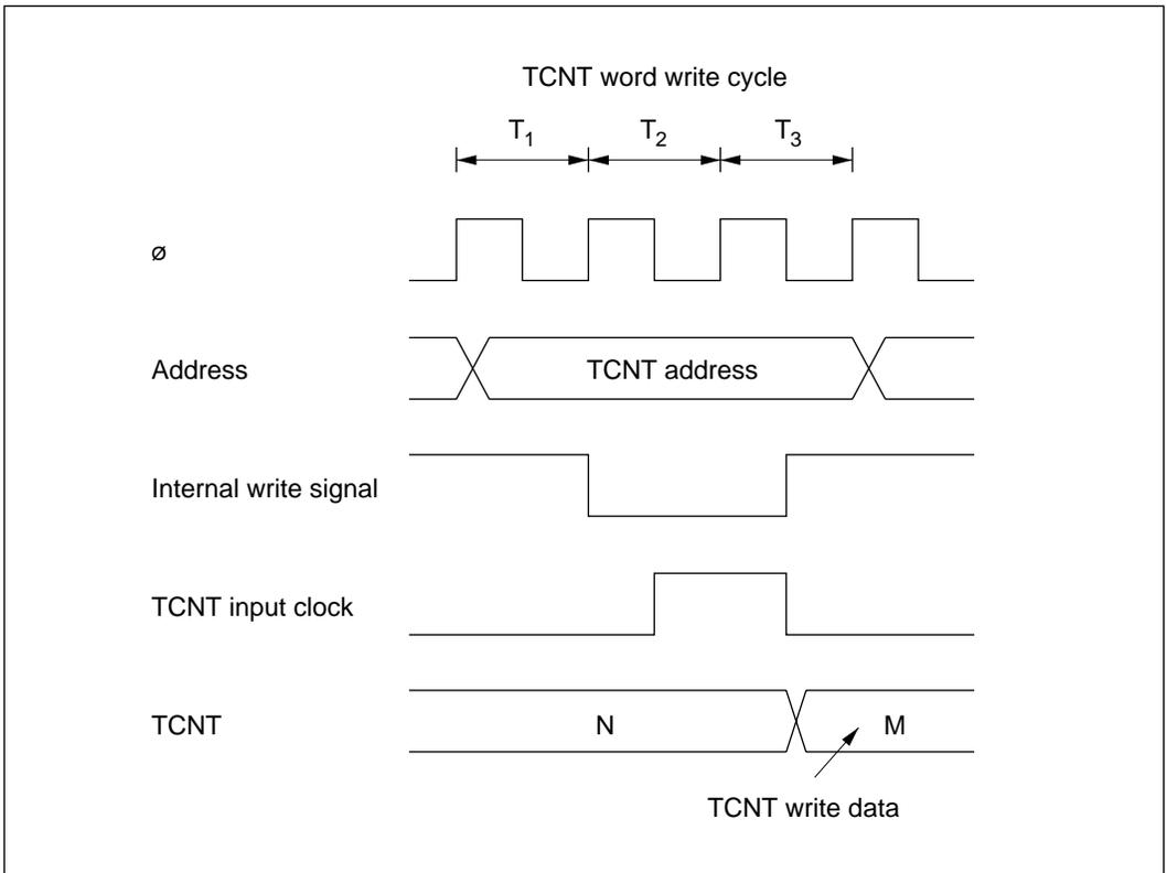
**Figure 10-62 Contention between TCNT Word Write and Increment**
