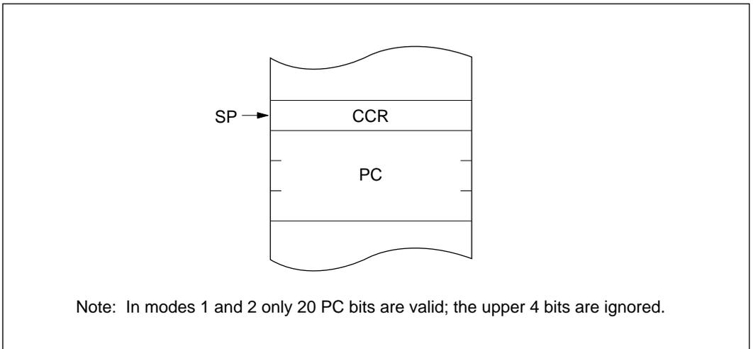
**Figure 4-5 Stack after Completion of Exception Handling**
