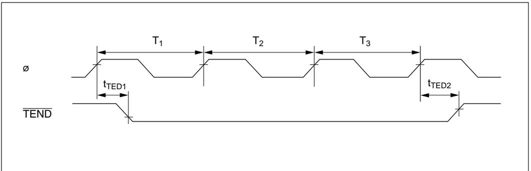
Figure 18-26 DMAC  $\overline{\text{TEND}}$  Output Timing/3 State Access
