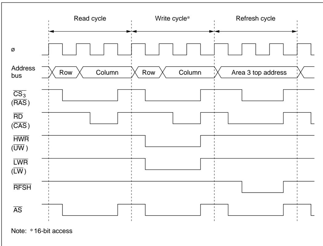
**Figure 7-5 DRAM Control Signal Output Timing (1) (2WE Mode)**
