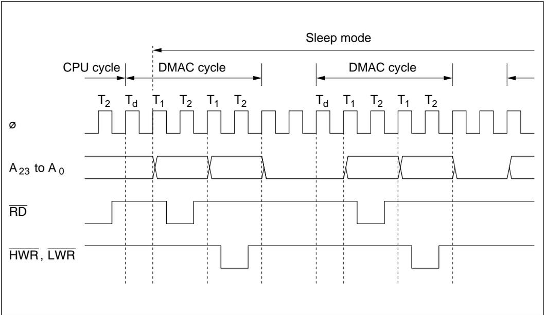
Figure 8-25 Timing of Cycle-Steal Transfer in Sleep Mode
