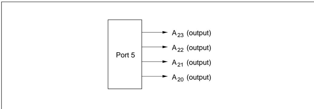
**Figure 9-6 Pin Functions in Modes 3 and 4 (Port 5)**
