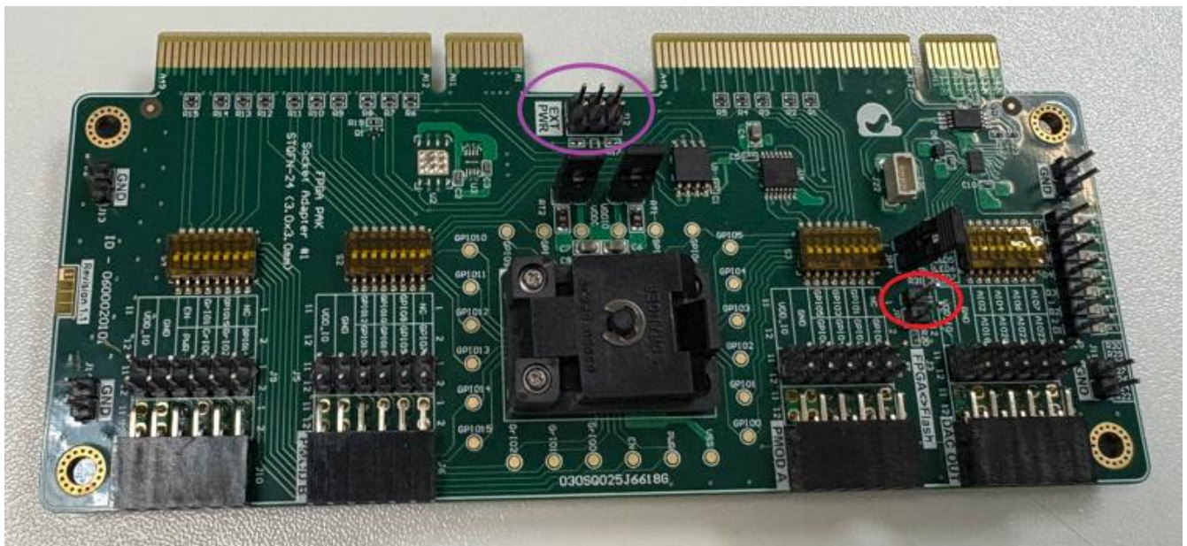
Figure 24. Jumpers and External Power Connection Points on the Board
