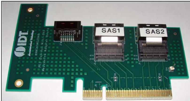
Figure 2.6 PCIe x8 Edge-to-SAS Adapter
