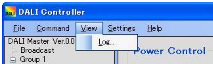
Log: Displays the Command Log Window. (For details, see **6.7 Command Log Window.**)
