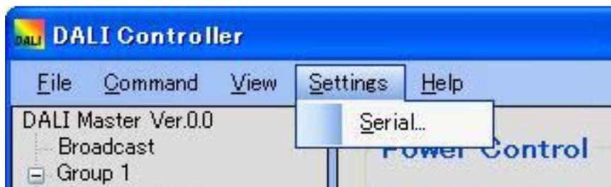
Serial: Specifies the COM port and communication speed. (For details, see **6.8 Serial Dialog Box.**)
