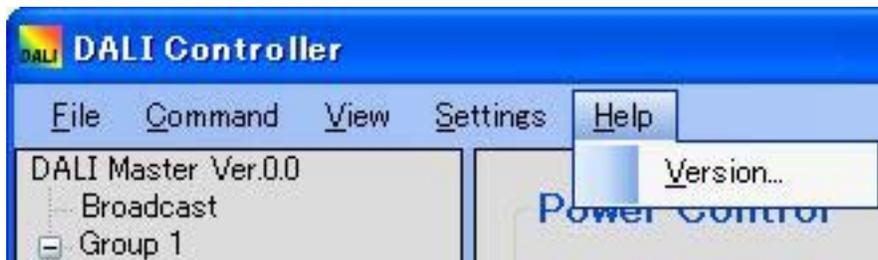
Version: Displays the DALI master controller GUI version. (For details, see **6.10 Version Dialog Box.**)
