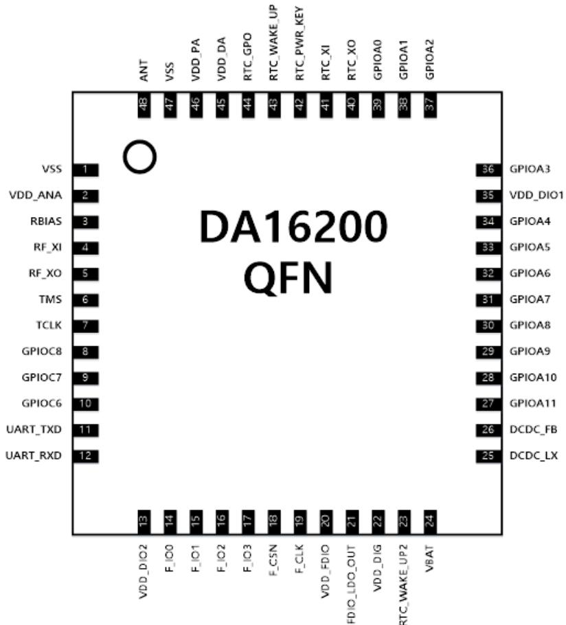
Figure 1. DA16200 QFN48 pinout diagram (Top view)
