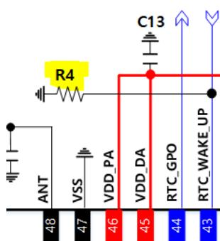
Figure 19. RTC\_WAKE\_UP circuit
