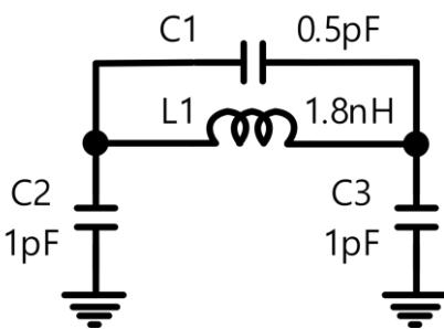
Figure 9. LC filter circuit
