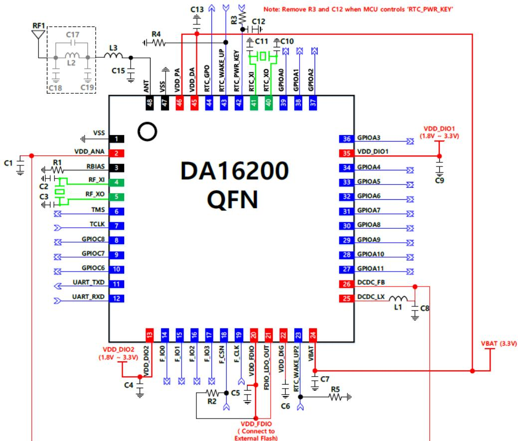
Figure 30. QFN reference for 1.8 V flash
