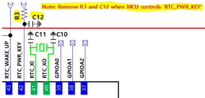
Figure 18. RTC\_PWR\_KEY circuit
