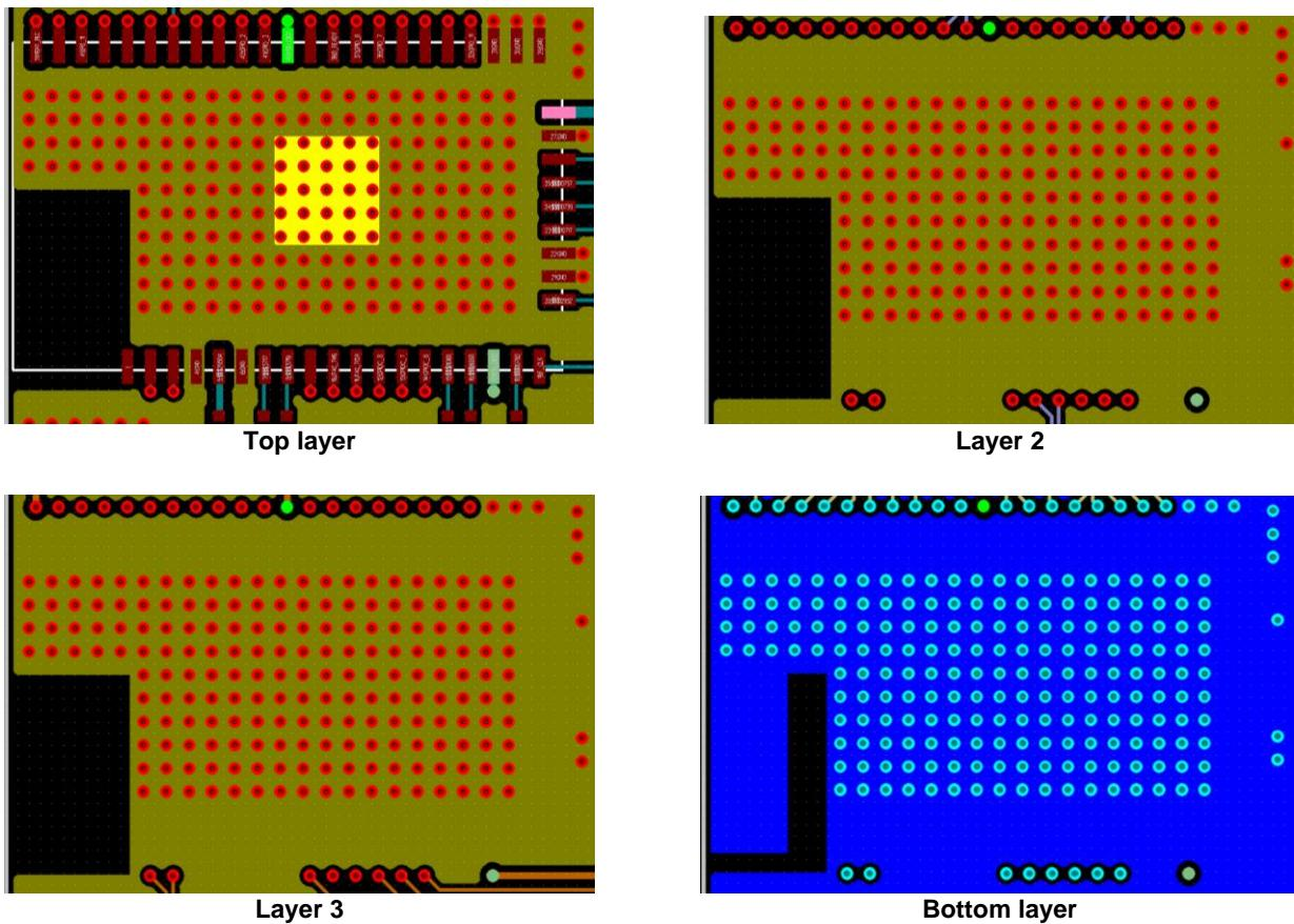
Figure 27. DA16600 4-layer PCB example
