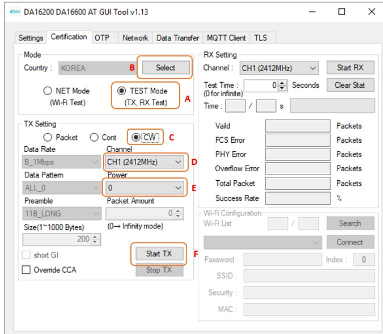
**Figure 11. Transmitting CW TX power setup**
