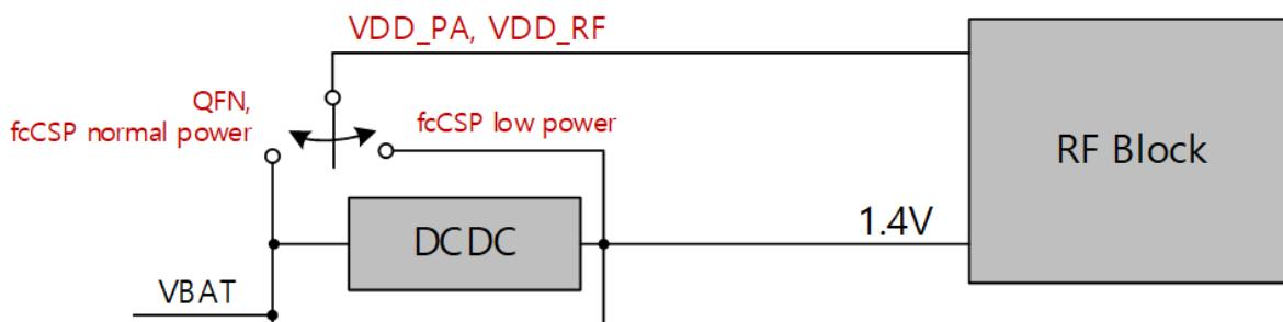
**Figure 5. High/Low TX power mode connection**
