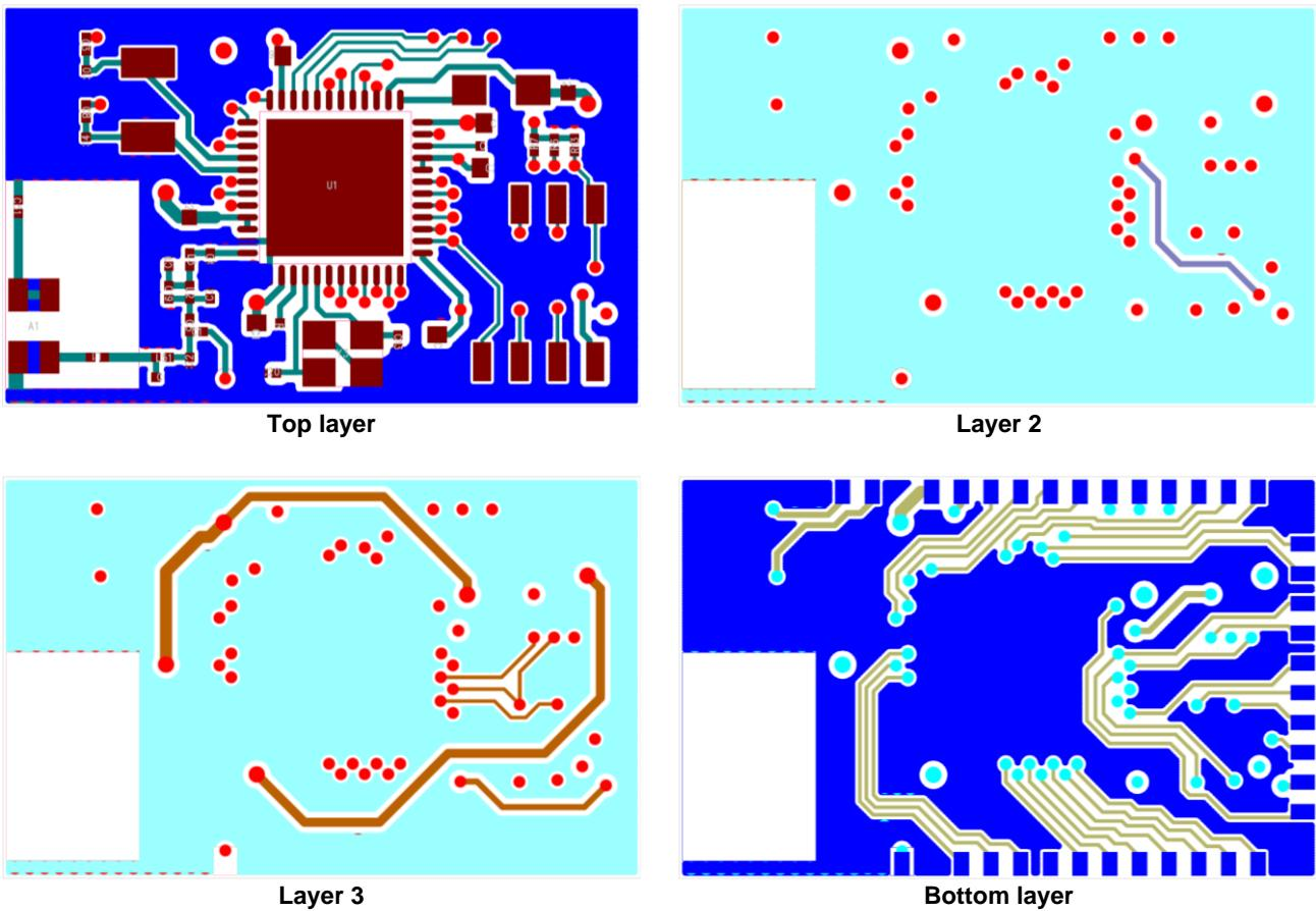
Figure 23. DA16200MOD 4-layer PCB example
