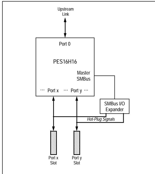
Figure 8.1 Hot-Plug on Switch Downstream Slots Application
