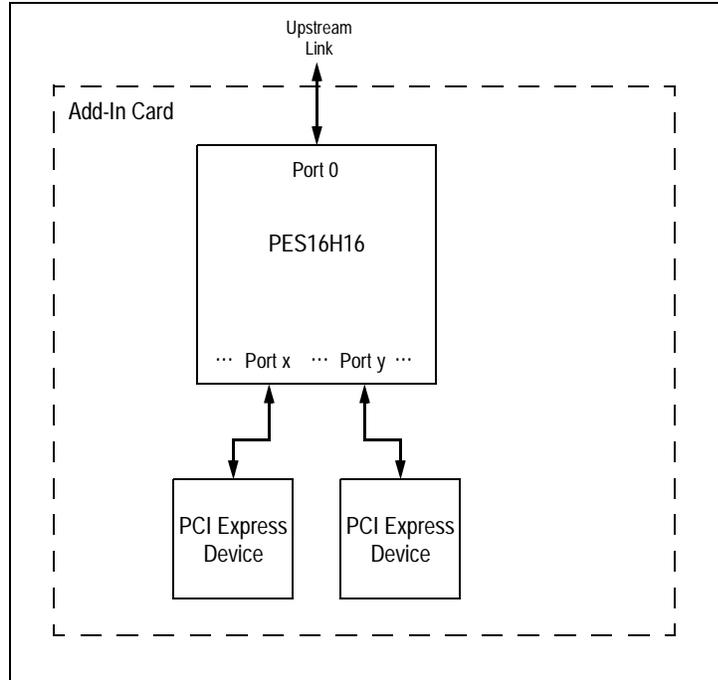
Figure 8.2 Hot-Plug with Switch on Add-In Card Application
