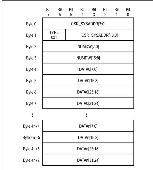
Figure 6.2 Sequential Double Word Initialization Sequence Format
