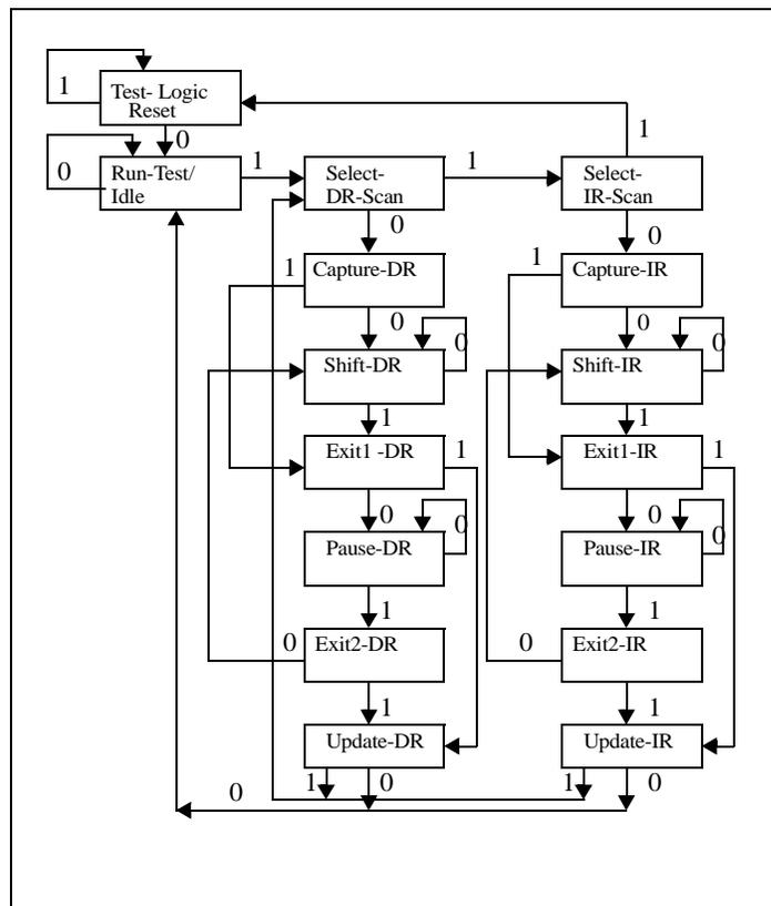
**Figure 10.2 State Diagram of PES16H16's TAP Controller**
