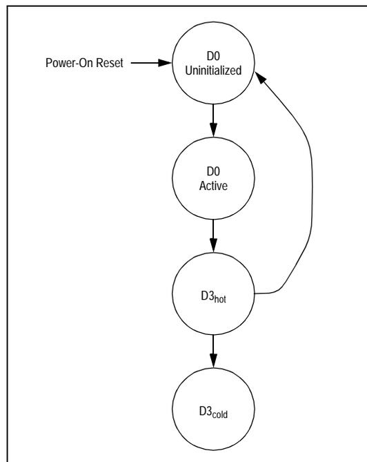
Figure 7.1 PES16H16 Power Management State Transition Diagram
