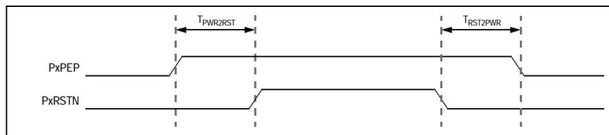
Figure 3.6 Power Enable Controlled Reset Output Mode Operation
