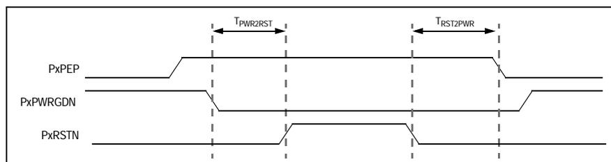
Figure 3.7 Power Good Controlled Reset Output Mode Operation
