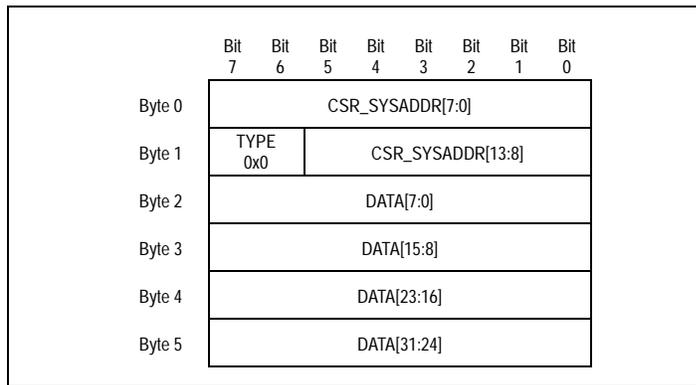
Figure 6.1 Single Double Word Initialization Sequence Format
