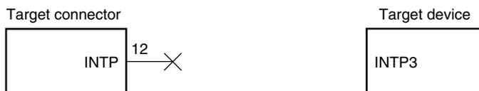
**Figure 20-4. Circuit Connection for the Case Where QB-MINI2 Is Used for Debugging and Debugging of INTP3 Pin Is Performed Only with Real Machine**
