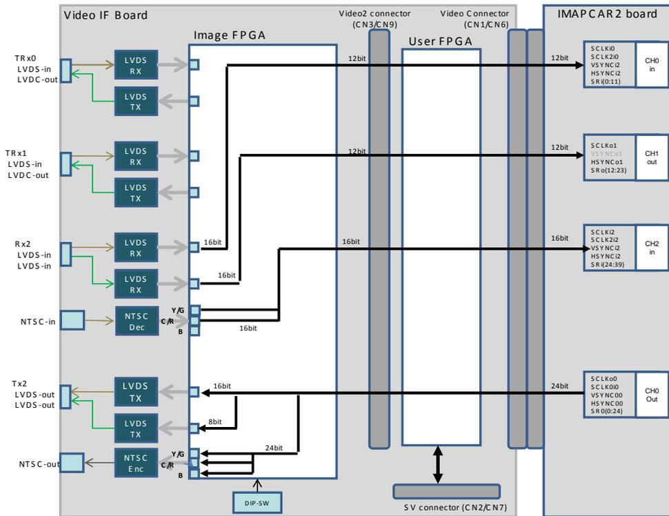
Internal composition of FPGA chart mode 5 (image system)
