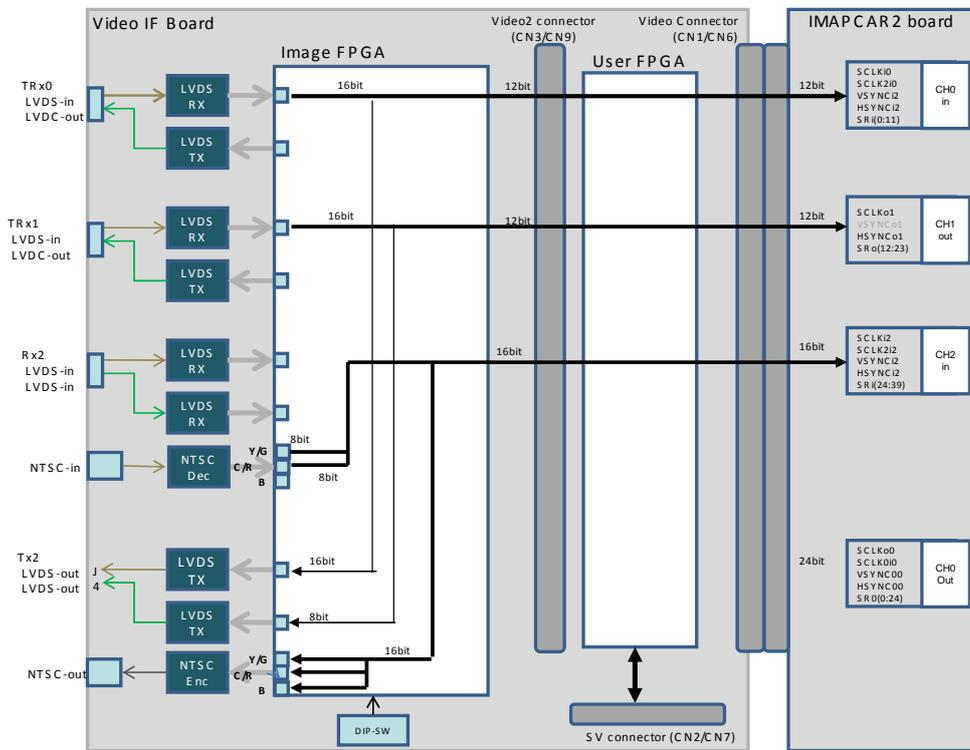
Internal composition of FPGA chart mode 4 (image system)
