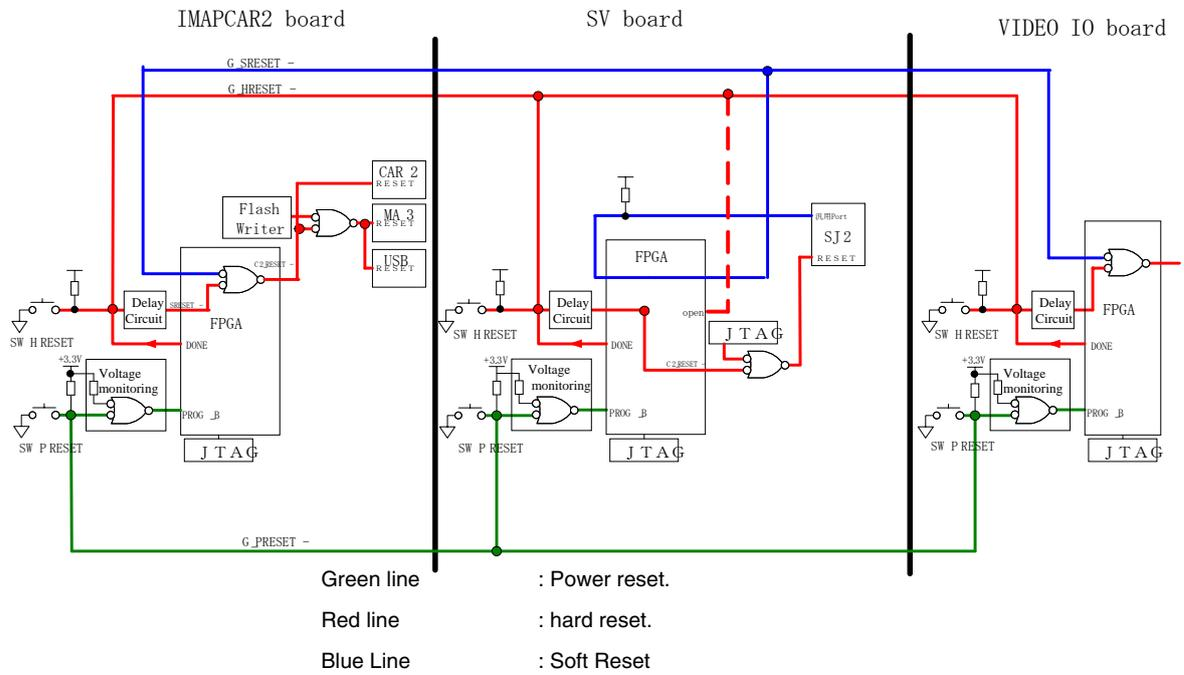
The following figure describes the reset schematic for the IMAPCAR2 video I/F board reset.
