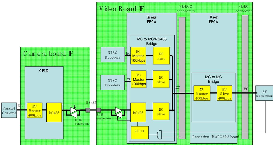
Internal composition of FPGA chart (I2C/ RS485 communication system)
