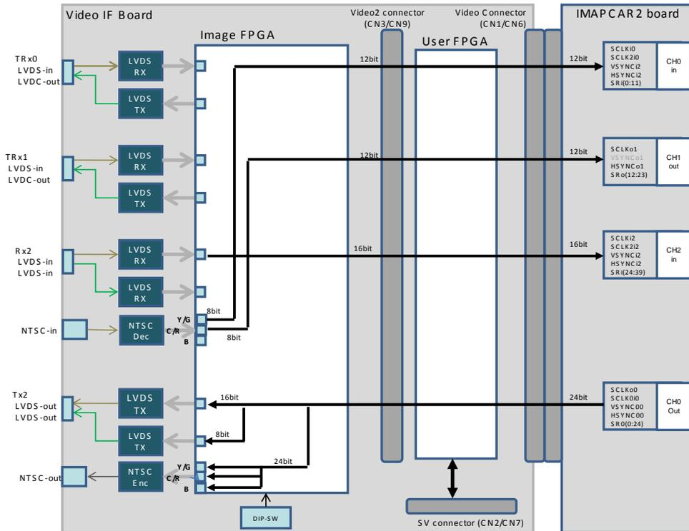
Internal composition of FPGA chart mode 3 (image system)
