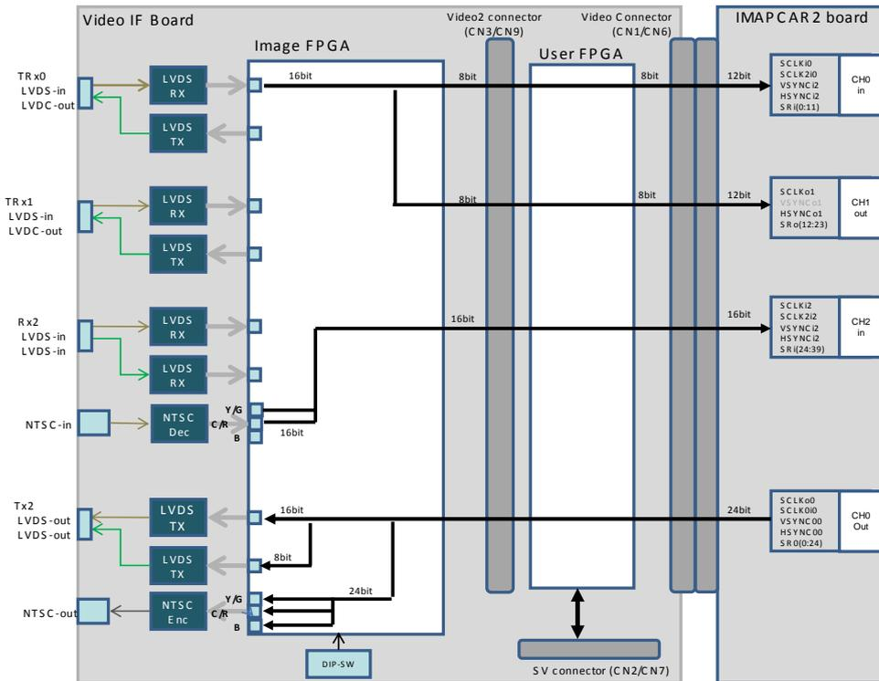
Internal composition of FPGA chart mode 1 (image system)
