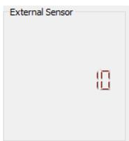
Ensure that the second row is selected (blue background), then click the *Start Measurement* button and turn the potentiometer cursor until the *External Sensor* numerical display shows 90%. Stop the measurement, and click the *Get Measurement Value for Calibration* button in the bottom left corner of the GUI.
