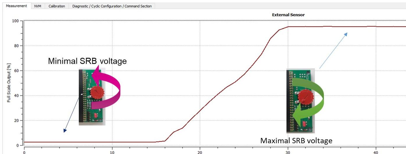
The output swings from 2,5% to 95% of the full scale.
