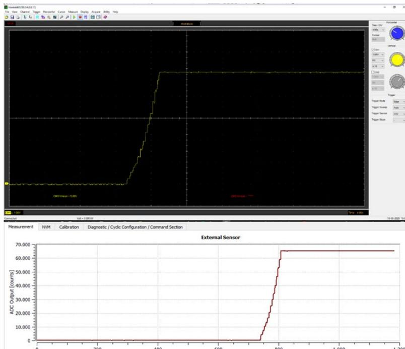
With a complete swing of a resistive bridge connected to the input of the IC, the analog output swings from 0V to about 5V (scale:1V/div.), while the digital output moves from a few hundreds to about 64K counts (corrected measurement visualized with a 16 bits resolution).
