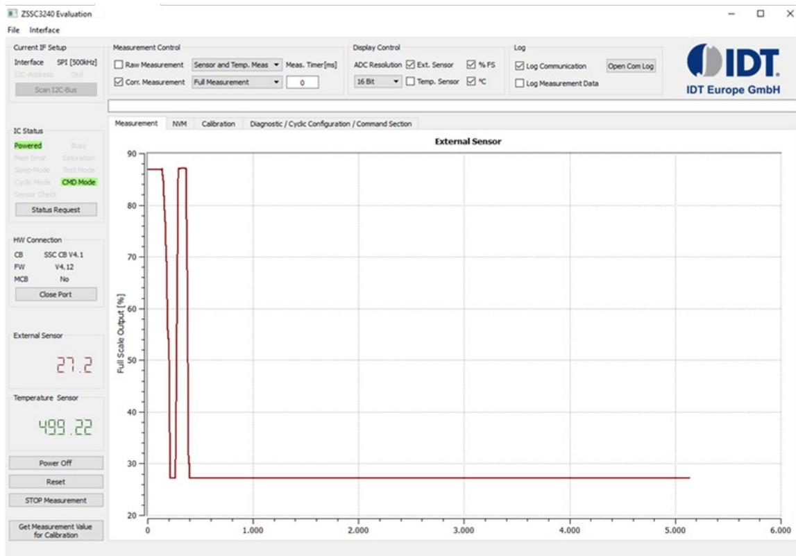
For most applications the maximum resolution of 24bits of data is not needed. The ADC resolution drop down menu allows scaling of the displayed data, regardless of the actual ADC setting of the ZSSC324x, as shown in Figure 18.
