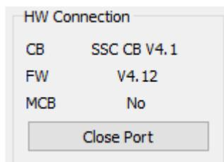
The *Open Port / Close Port* button allows opening and closing the USB communication port. This is useful for making hardware changes (for example, switching the DUT or jumper settings) without exiting the GUI.
