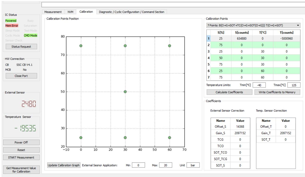
The primary purpose of the *Calibration* tab is the overview of the calibration data and the resulting coefficients. On the top right, the calibration input is displayed where the calibration points are entered. The resulting coefficients, which are the output of the calibration process, are shown below the *Calibration Point* table, see Figure 32.
