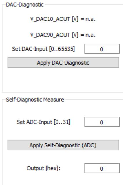
The DAC section gives the user the possibility to set a digital value to the input of the DAC. By clicking on the button *Apply DAC-Diagnostic*, the DAC output is updated and can be checked against its value in the selected output range. For further details, refer to the ZSSC324x Data Sheet.
