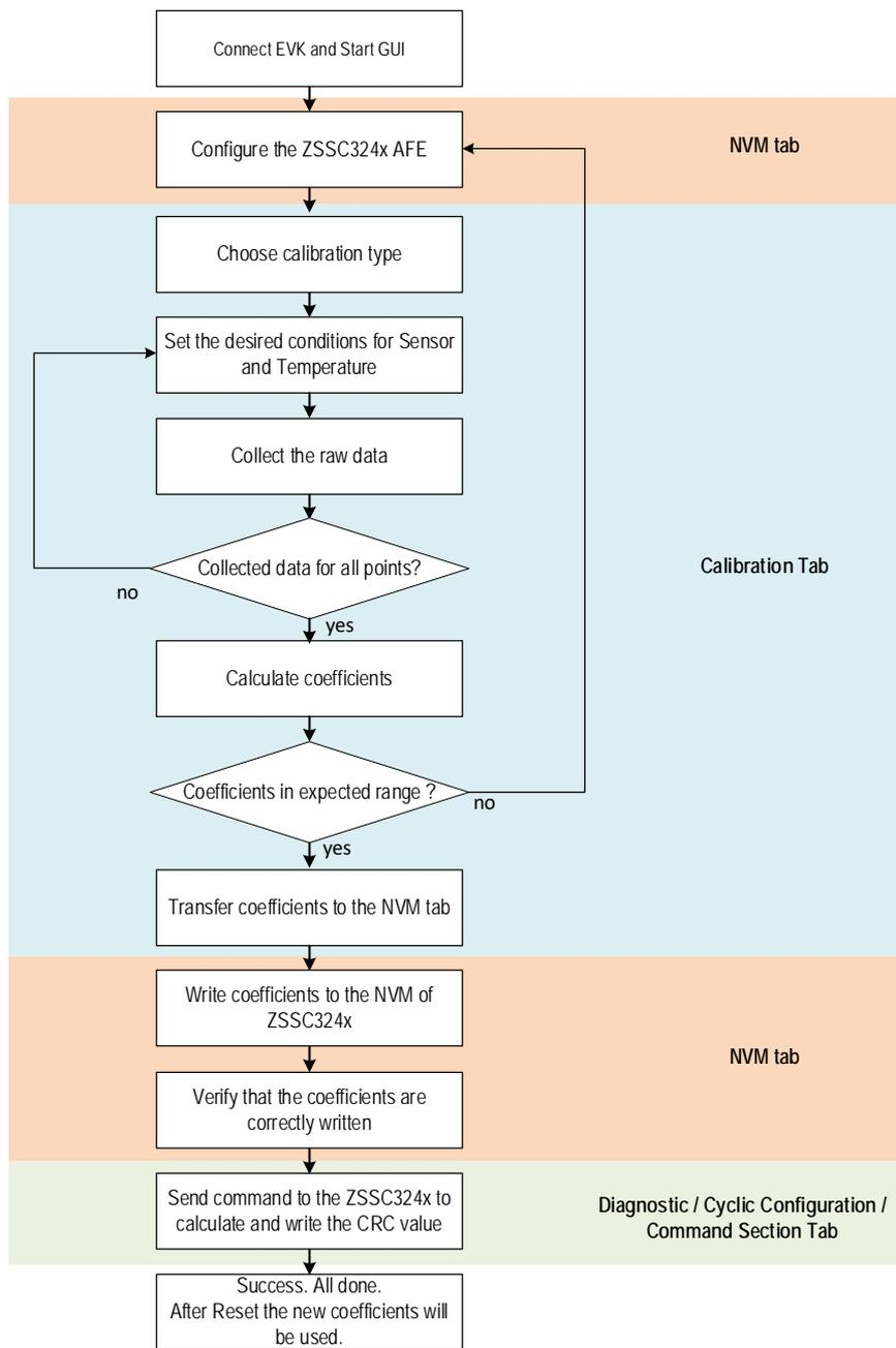
This calibration example uses the [Sensor Replacement Board](#) (SRB) to emulate a sensor signal. A typical calibration flow includes the five basic steps:
