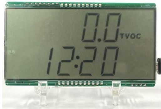
Figure 3. LCD Display in IAQ and RTC Mode
