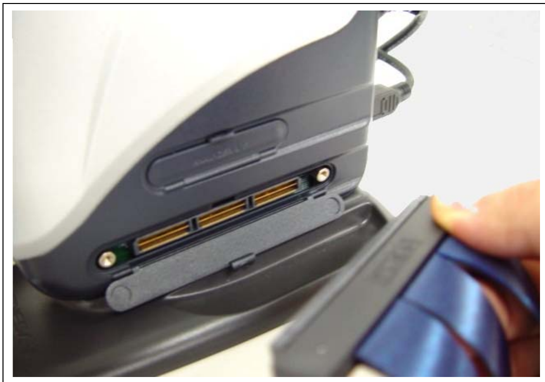
Figure 2.11 Connecting the Trace Cable to E200F when Using the EV-chip Unit
