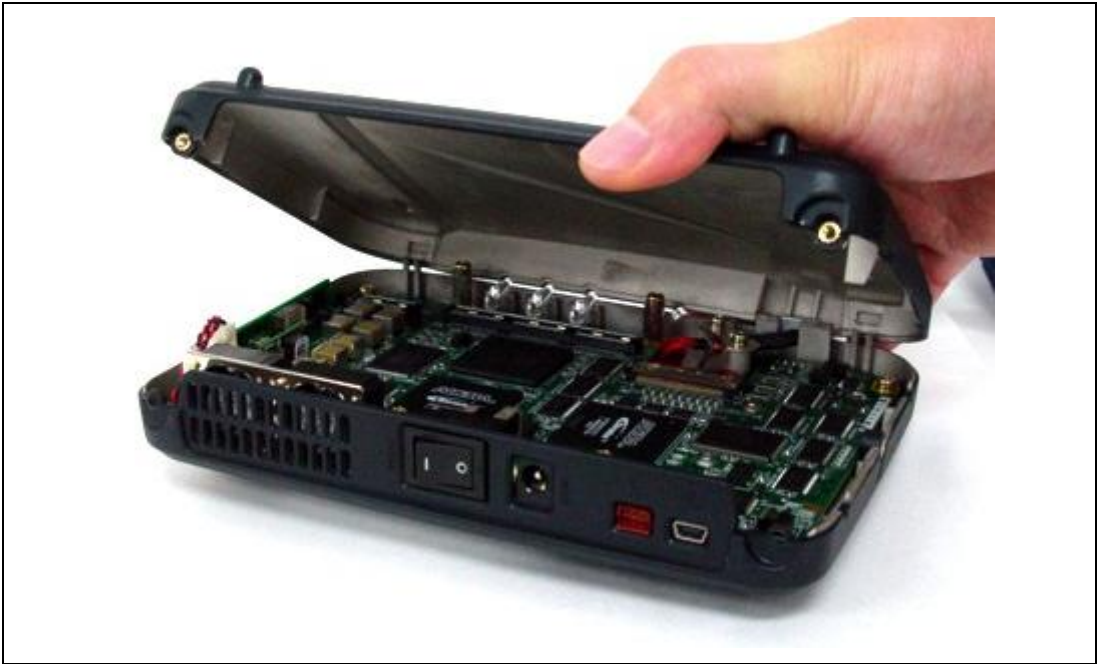
Figure 2.22 Removing the Main Unit Case
