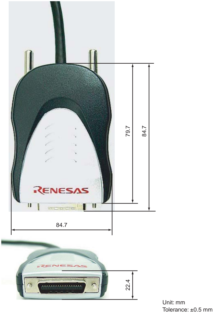
Figure 3.1 External Dimensions of the Probe H-UDI/AUD
