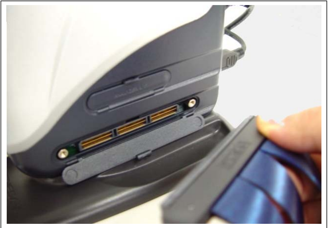
Figure 2.2 Connecting the Trace Cable to E200F
