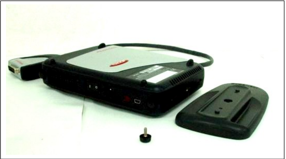
Figure 2.20 Removing the Base Unit for Placing the Emulator Vertically
