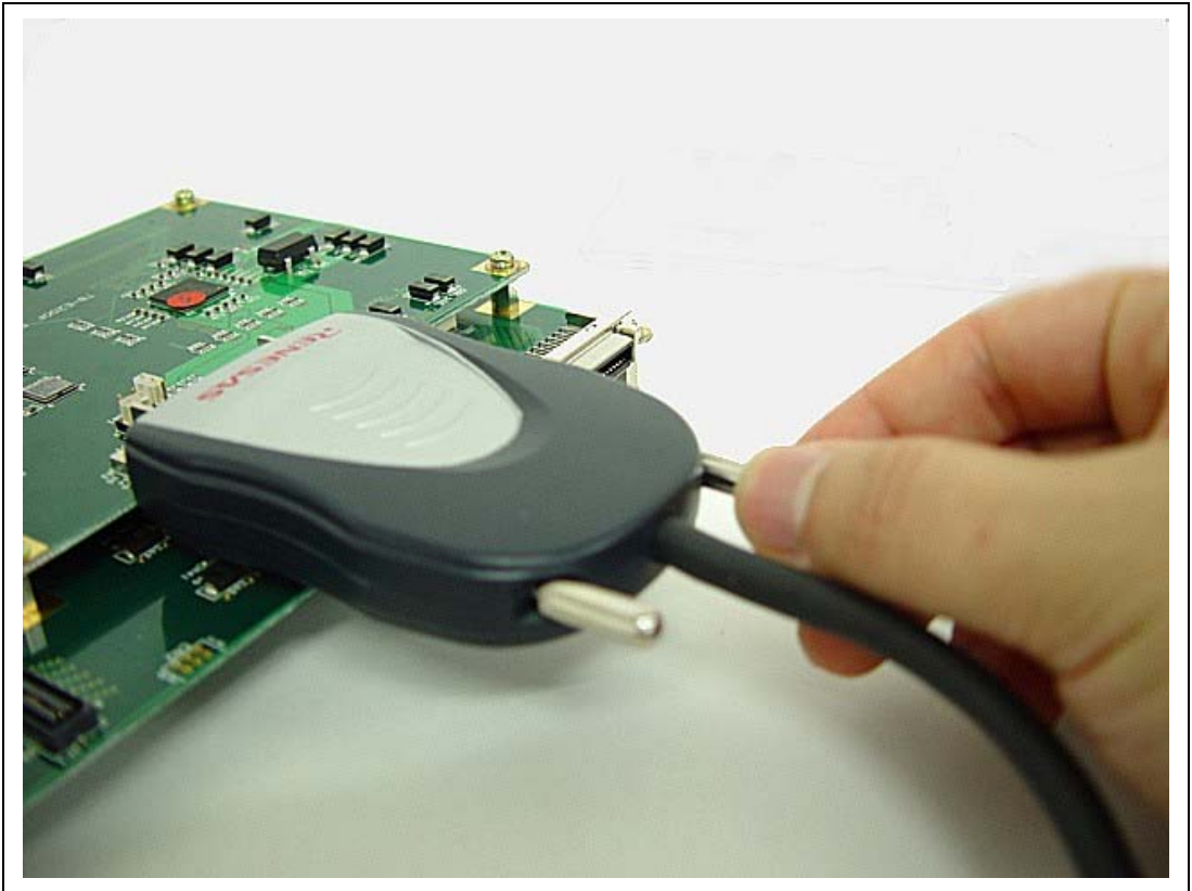
Figure 2.28 Fastening the User System and the H-UDI Probe
