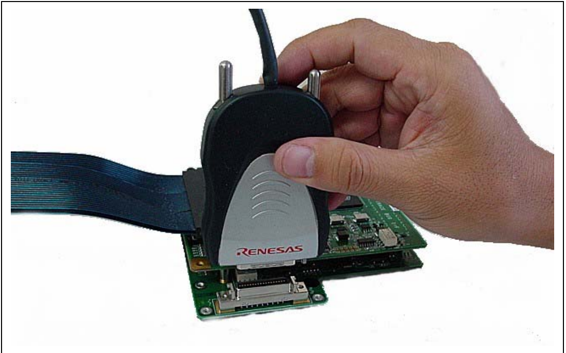
Figure 2.18 Connecting the Probe H-UDI/AUD to the EV-chip Unit
