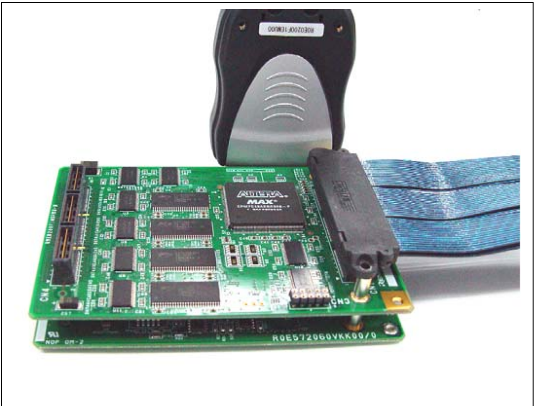
Figure 2.16 Connecting the Emulation Memory Unit, EV-chip Unit, and Trace Cable
