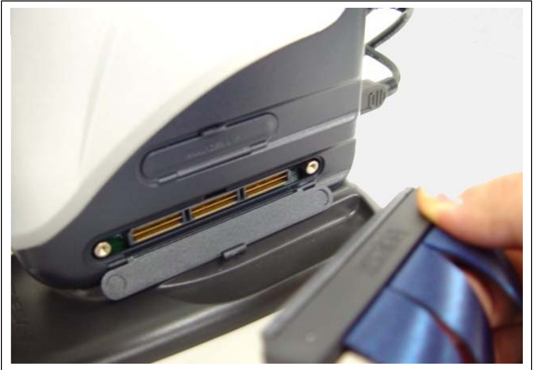
Figure 2.5 Connecting the Trace Cable to E200F
