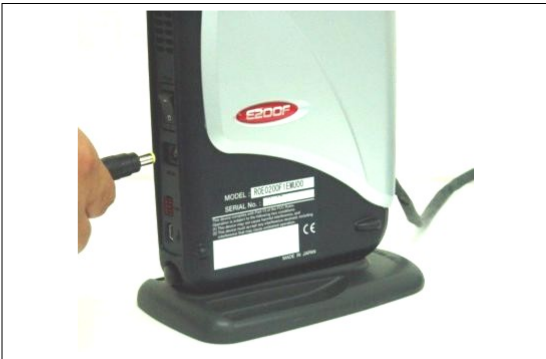
Figure 2.25 Connecting the AC Adapter to the Main Unit Case
