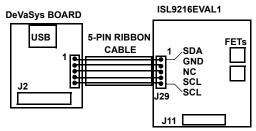
FIGURE 6. |2C CONNECTION TO ISL9216 PCB
