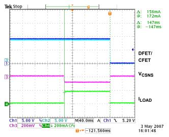
FIGURE 10. CHARGE OVERCURRENT TEST (0.1V THRESHOLD, 160ms TIME DELAY,  $0.5\Omega$  SENSE RESISTOR)
