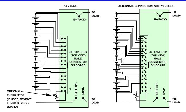
FIGURE 3. BATTERY CELL CONNECTION TO ISL9216 PCB
