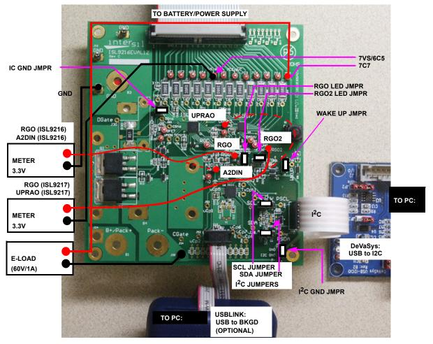
FIGURE 1. ISL9208EVAL1 BOARD CONNECTION
