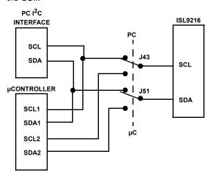
FIGURE 7. PC OR µC CONNECTION TO THE ISL9216
