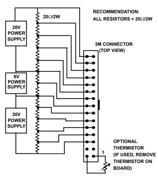
FIGURE 5. POWER SUPPLY/RESISTOR CONNECTION TO ISL9216 PCB
