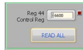
FIGURE 12. READ BACK FROM THE CONTROL REGISTER 44
