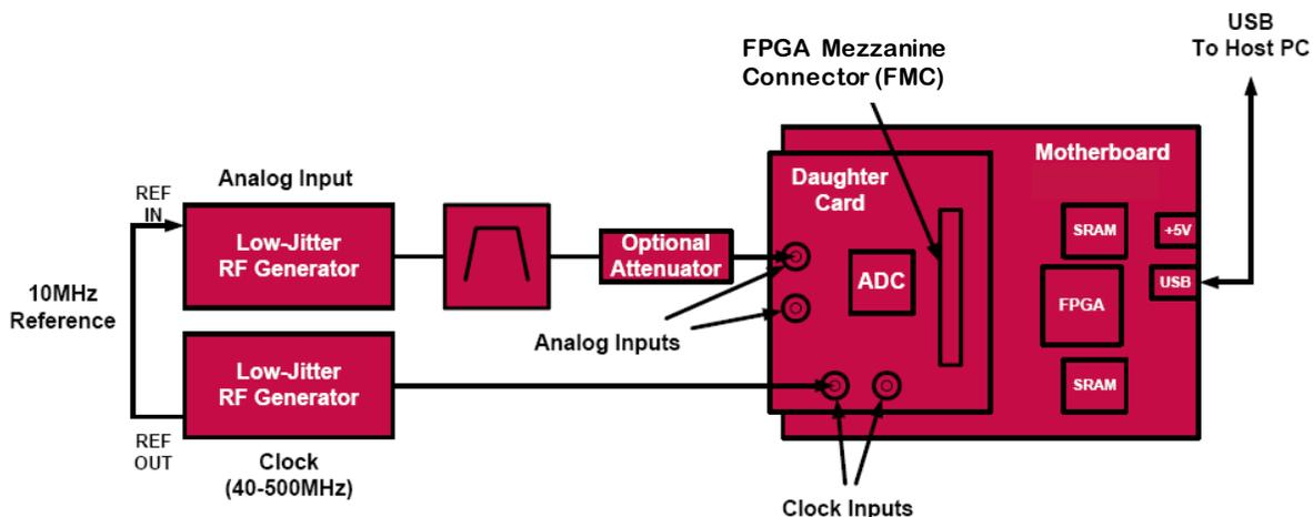
FIGURE 1. EVALUATION PLATFORM BLOCK DIAGRAM
