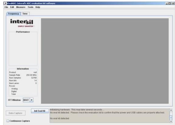
After clicking on the "Data Capture" button with a powered up evaluation kit attached, a window similar to the following is displayed. The diagram shows the major portions of the iEvalADC GUI.
