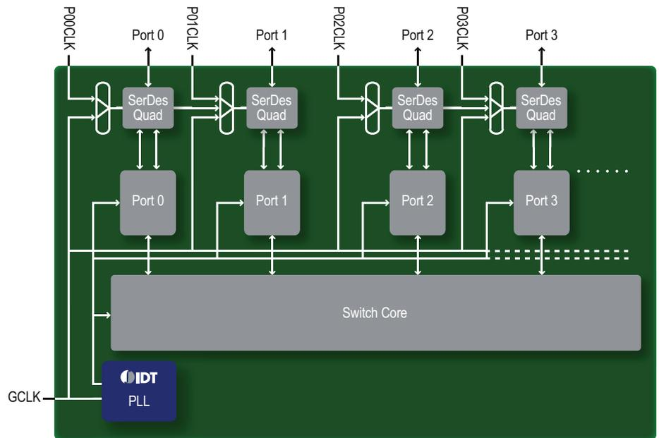
The Global Reference Clock inputs to the PLL are used to generate all of the clocks required by the internal switch logic and the SerDes. The Local Port Reference Clock input associated with a port (or a group of ports in the Gen2 Inter-Domain Switches) is used by the SerDes only when a port (or a group of ports in the Gen2 Inter-Domain Switches) is configured to function in local port clocked mode. Local Port Clock refers to the clock that a port uses to receive and transmit serial data.
