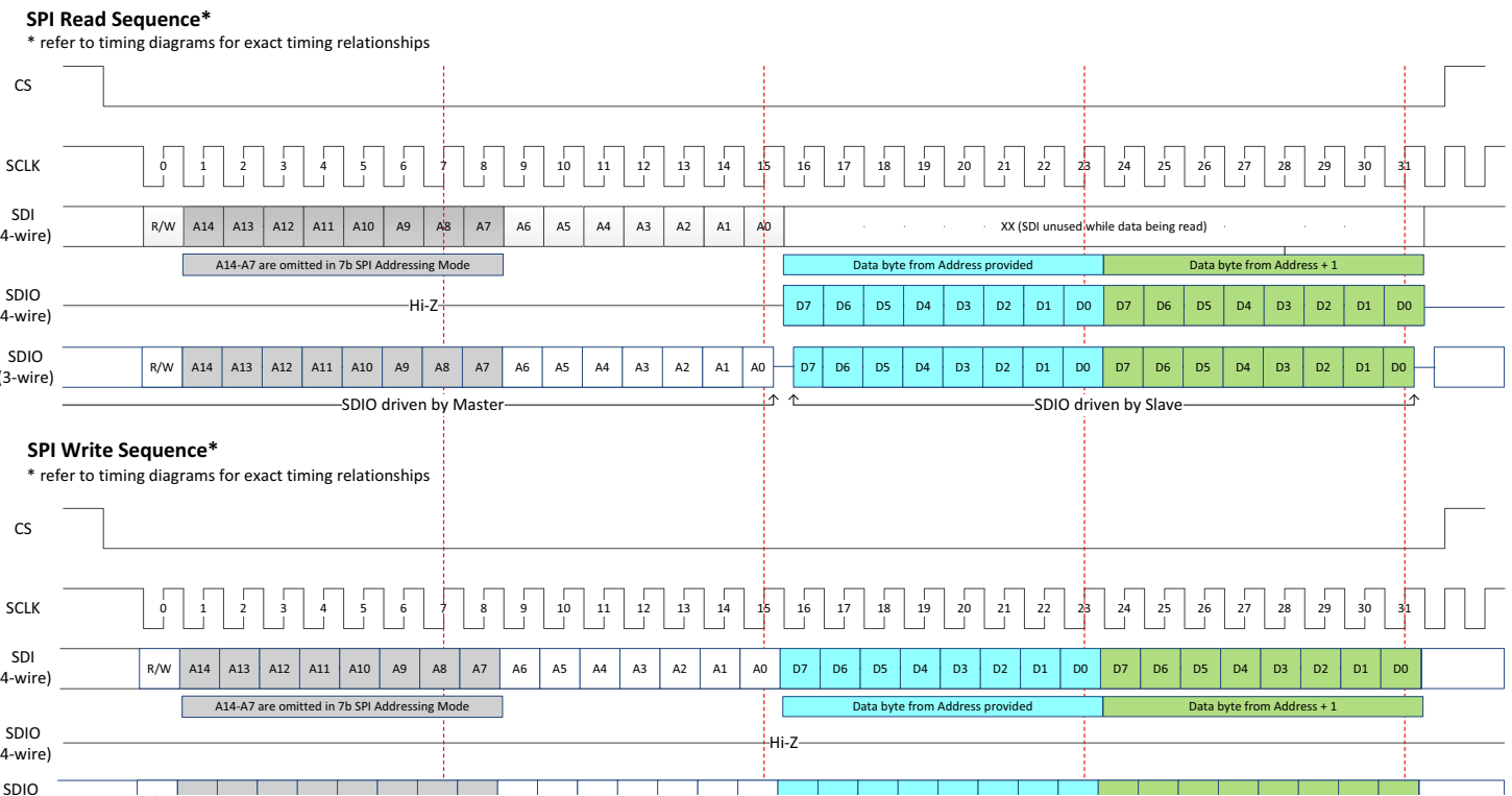
Figure 3: SPI Sequencing Diagram
