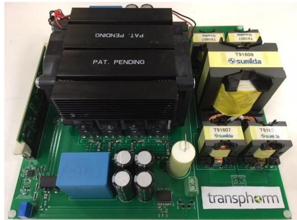
Figure 2. TPH3205WSBQA 100 kHz 3.3kW DAB prototype
