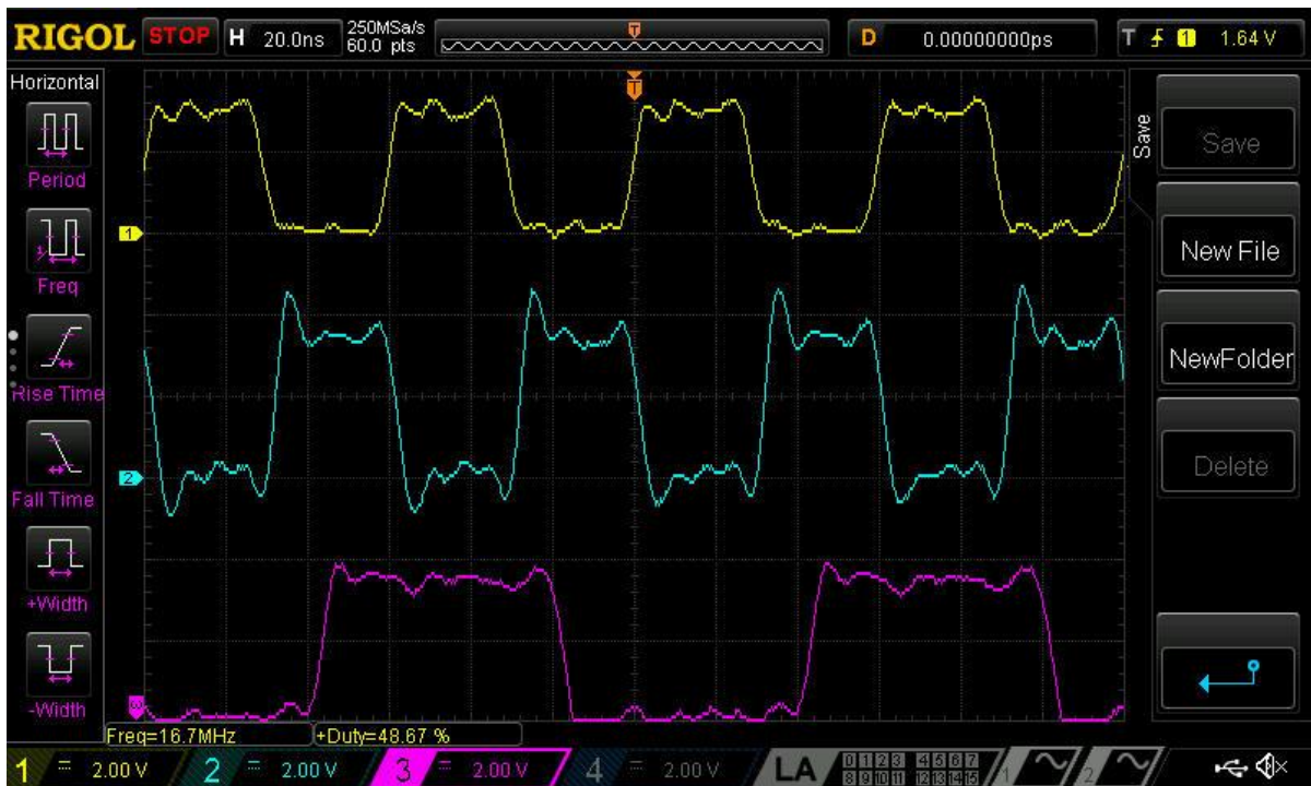
4. Period is 60ns. Pulse width is 40ns DC=66.67% (Correct functionality)
