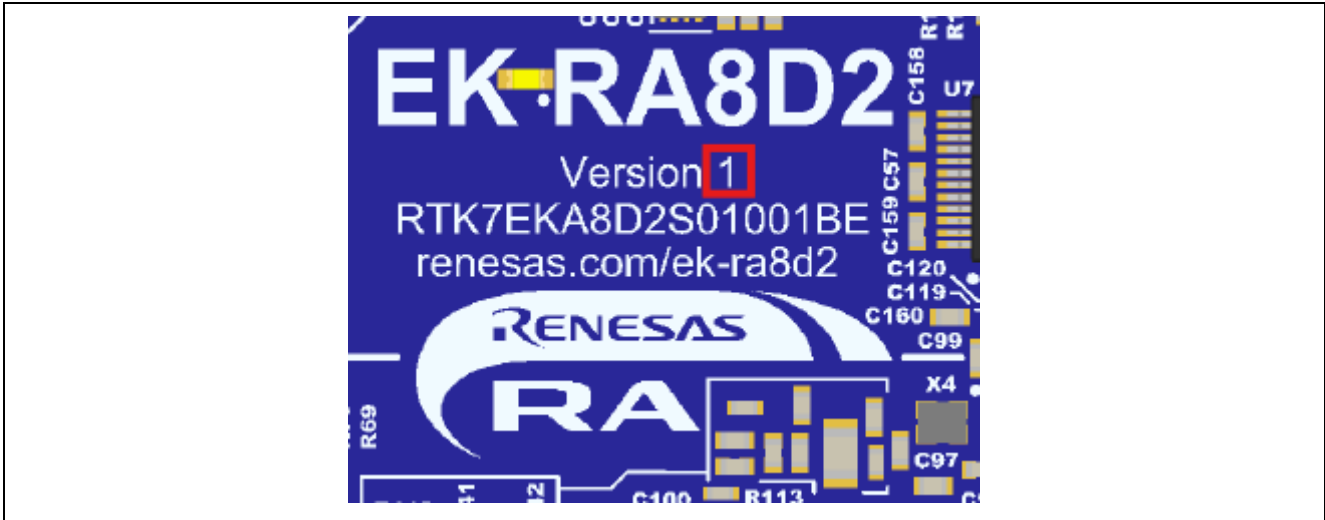
Figure 6. Identification of the Kit Version Number on the EK-RA8D2 Board
