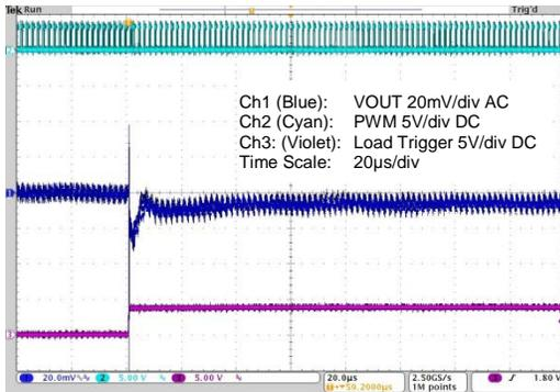
**Figure 4.39 ZSPM1035D with Capacitor Range #4 – Load Step 15 to 5A, Min. Capacitance**
