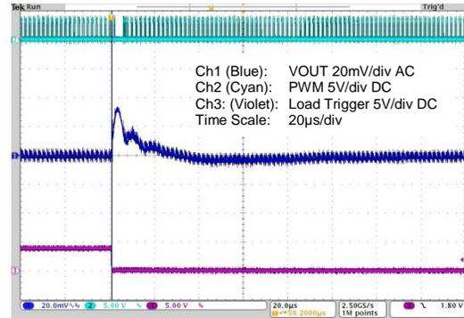
**Figure 4.20 ZSPM1035C with Capacitor Range #4 – Load Step 5 to 15A, Max. Capacitance**
