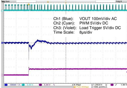
Figure 4.4 ZSPM1035C with Capacitor Range #1 – Load Step 15 to 5A, Min. Capacitance
