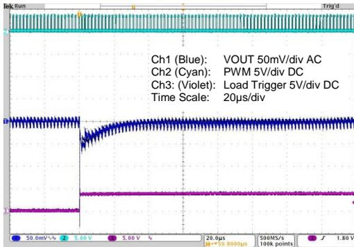
Figure 4.34 ZSPM1035D with Capacitor Range #3 – Load Step 15 to 5A, Min. Capacitance
