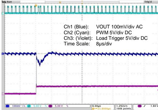
**Figure 4.24 ZSPM1035D with Capacitor Range #1 – Load Step 15 to 5A, Min. Capacitance**
