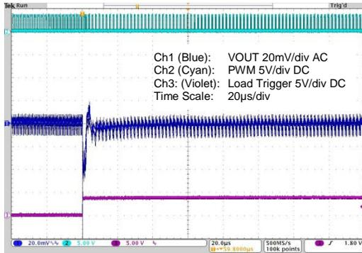
**Figure 4.14 ZSPM1035C with Capacitor Range #3 – Load Step 15 to 5A, Min. Capacitance**
