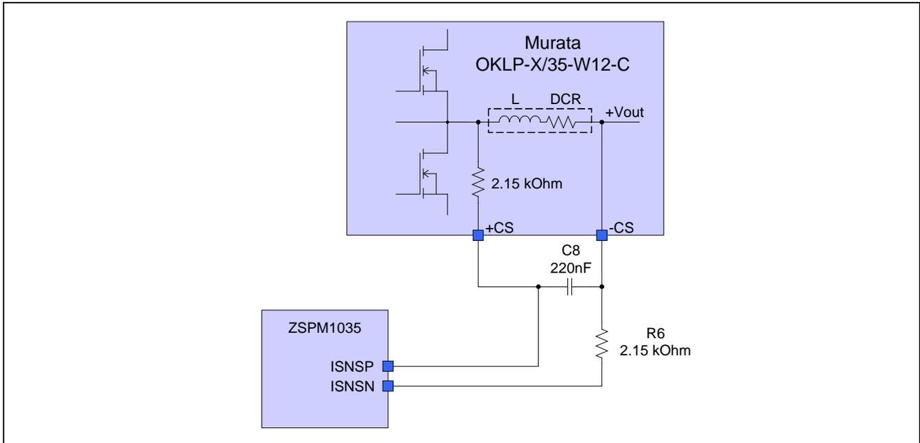
To improve the accuracy of the current measurement, which can be adversely affected by the temperature coefficient of the inductor's DCR, the ZSPM1035C/D features temperature compensation via the external temperature sensing. The temperature of the inductor can be measured with an external temperature sense element placed close to the inductor. This information is used to adapt the gain of the current sense path to compensate for the increase in actual DCR.
