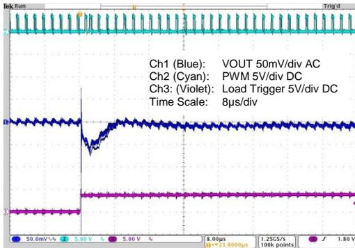
Figure 4.29 ZSPM1035D with Capacitor Range #2 – Load Step 15 to 5A, Min. Capacitance
