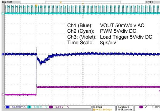
Figure 4.9 ZSPM1035C with Capacitor Range #2 – Load Step 15 to 5A, Min. Capacitance
