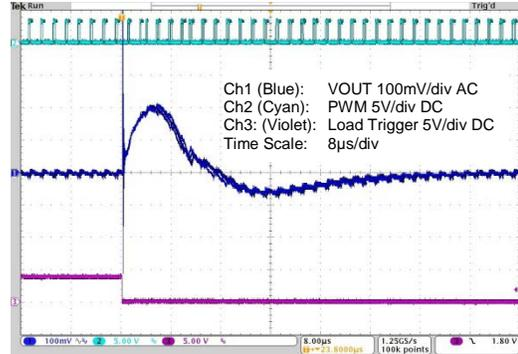
**Figure 4.25 ZSPM1035D with Capacitor Range #1 – Load Step 5 to 15A, Max. Capacitance**
