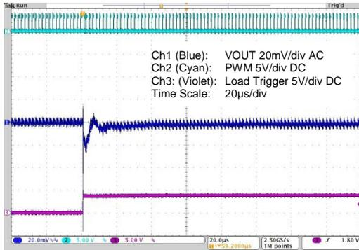
**Figure 4.19 ZSPM1035C with Capacitor Range #4 – Load Step 15 to 5A, Min. Capacitance**
