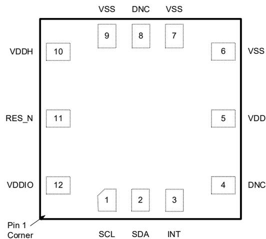
Figure 4. Pin Assignments – Top View
