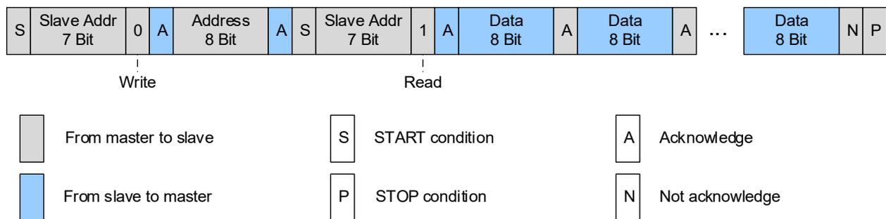
Figure 7. I<sup>2</sup>C Data Transmission Protocol
