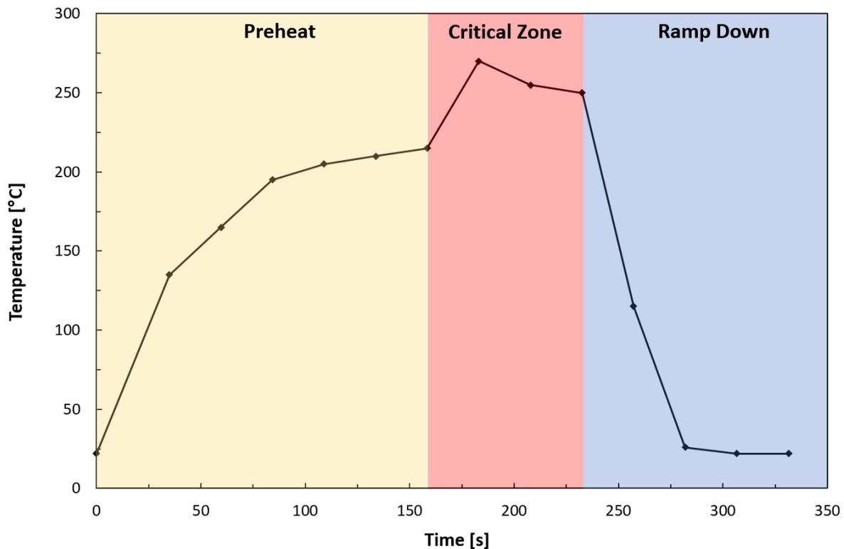
Figure 6. Typical Solder Profile
