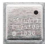
Figure 1. ZMOD4510 Gas Sensor
