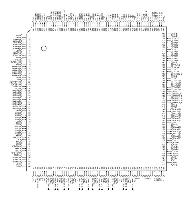
**Remark** IC: internal connect pin. Leave the IC pins open.
