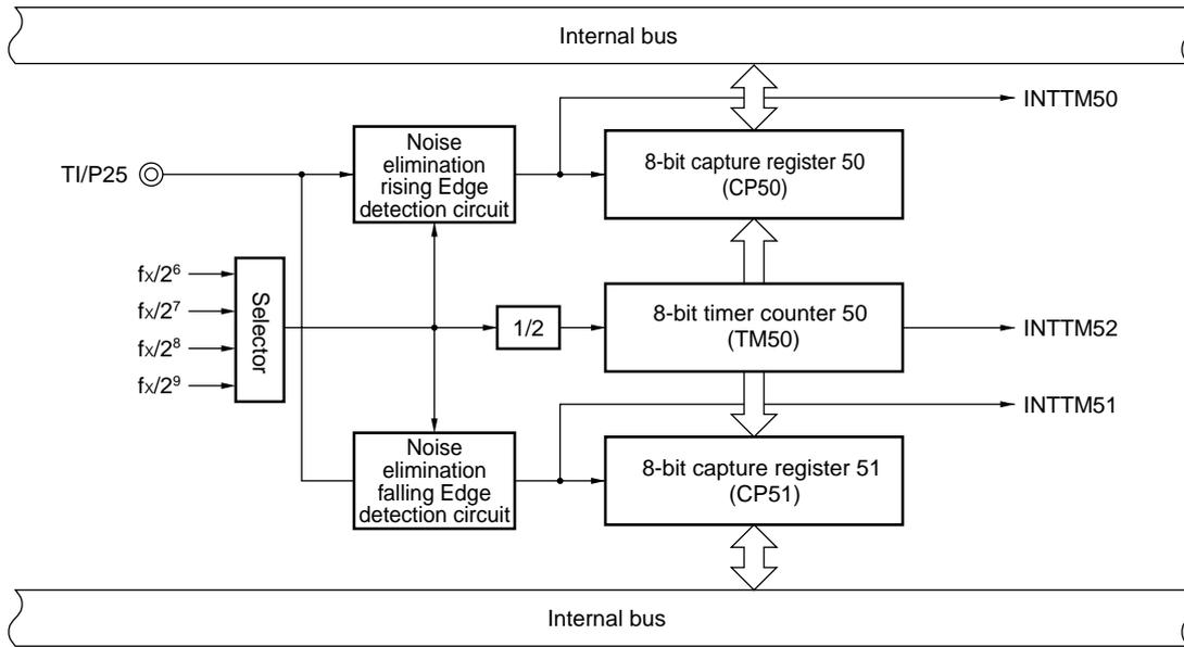
Figure 5-3. Block Diagram of 8-Bit Timer 80
