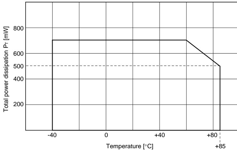
How to calculate total power dissipation
