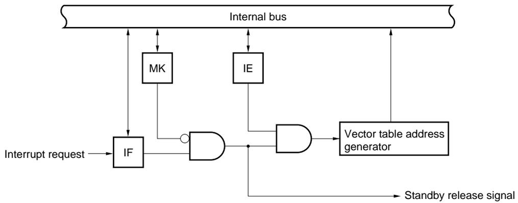
(C) External maskable interrupt (INTP0, INTP1)
