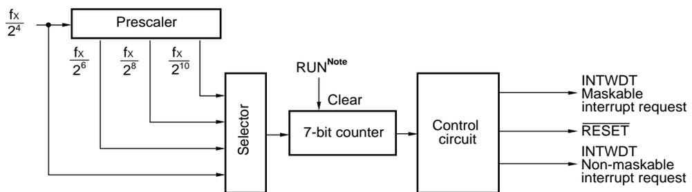
**Note** Bit 7 of the Watchdog timer mode control register (WDTM)
