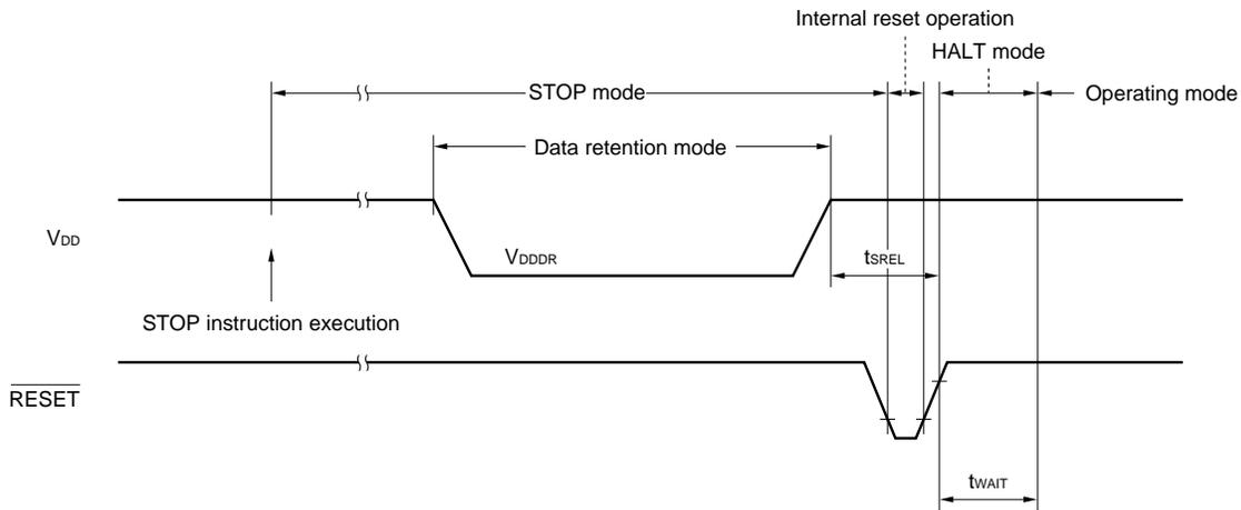
**Data Retention Timing (Standby release signal: STOP mode release by interrupt signal)**
