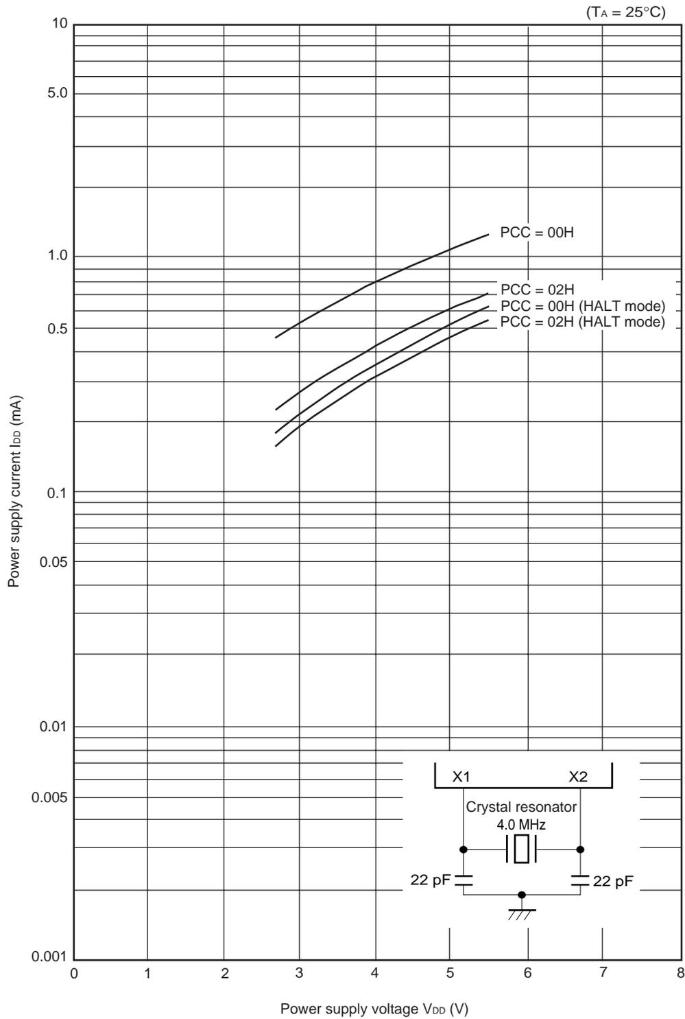
I<sub>DD</sub> vs V<sub>DD</sub> (System clock: 2.0-MHz crystal resonator)
