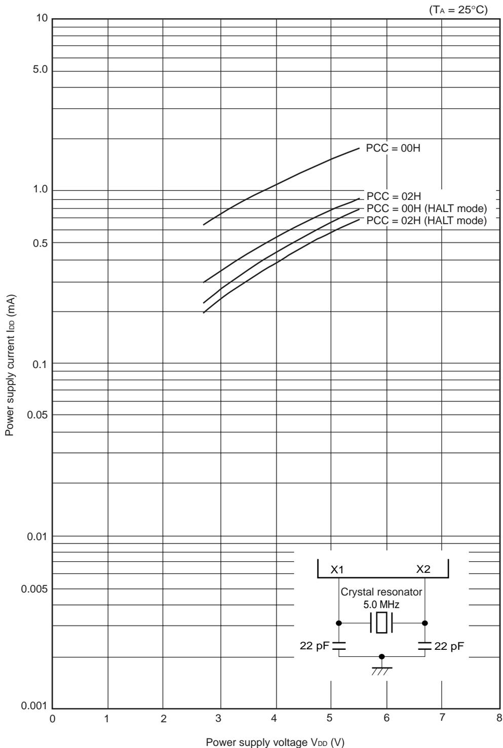
I<sub>DD</sub> vs V<sub>DD</sub> (System clock: 4.0-MHz crystal resonator)
