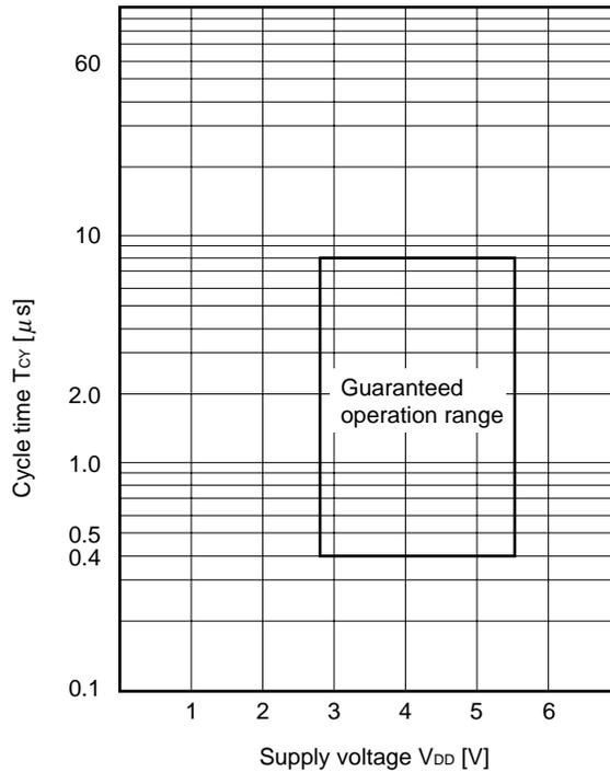
(2) Serial interface (T<sub>A</sub> = -40 to +85°C, V<sub>DD</sub> = 2.7 to 5.5 V)
