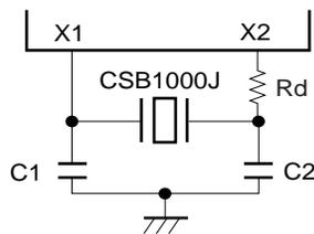
**Caution** The oscillator constant and oscillation voltage range indicate conditions of stable oscillation. Oscillation frequency precision is not guaranteed. For applications requiring oscillation frequency precision, the oscillation frequency must be adjusted on the implementation circuit. For details, please contact directly the manufacturer of the resonator you will use.
