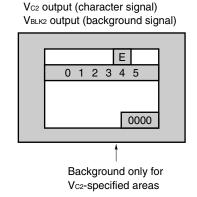
**Remarks 1.** The above figures are only examples. Actually, the background can be controlled independently for each output channel (only in RGB+Vc1+Vc2 mode), for example, by applying background (overall/minimum) for the RGB channel but not for the other channels.
