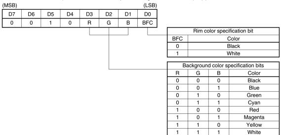
(2) For LSB-first transfer (Command bits are input starting from the LSB (D0). The function of each bit is the same as that for MSB-first transfer.)
