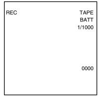
The Vc1 channel outputs the characters of all rows regardless of the setting of the Vc1 bit, excluding the characters for which the Vc2 channel is specified. Characters output via  $V_{\text{C2}}$  channel (specified characters of specified rows)
