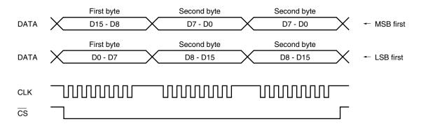
The 2-byte continuous command is used to write characters to video RAM. When continuously writing characters for which the specifications for the color, blinking, reversing, and Vc2 channel are the same, transfer the first byte of the first command then continuously transfer only the second bytes (character pattern addresses) of the commands.
