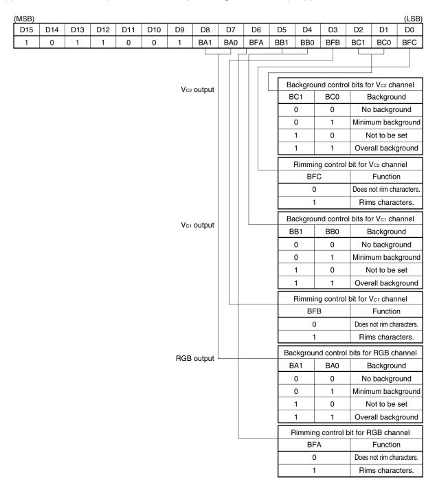
(2) For LSB-first transfer (Command bits are input starting from the LSB (D0). The function of each bit is the same as that for MSB-first transfer.)
