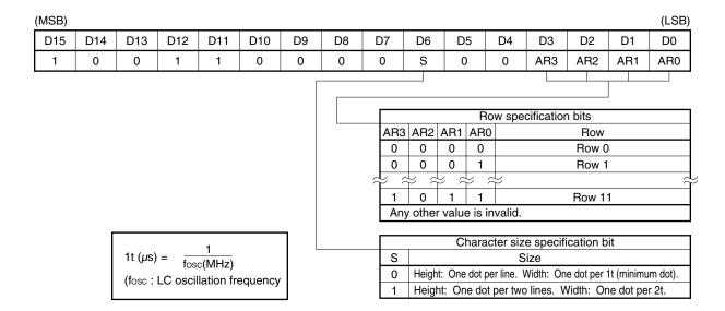
(2) For LSB-first transfer (Command bits are input starting from the LSB (D0). The function of each bit is the same as that for MSB-first transfer.)
