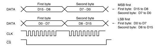
When inputting a 2-byte command, keep the  $\overline{\text{CS}}$  signal low between the first and second bytes of the command.
