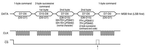
It is not necessary to make  $\overline{\text{CS}}$  low and then back high again.
