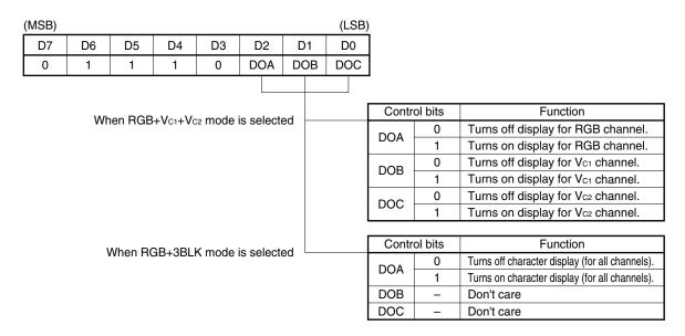
(2) For LSB-first transfer (Command bits are input starting from the LSB (D0). The function of each bit is the same as that for MSB-first transfer.)
