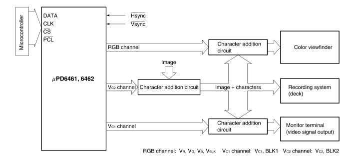
Example of application to a camcorder (2) (in RGB+3BLK mode for RGB compatible blanking) (The V<sub>R</sub>, V<sub>G</sub>, V<sub>B</sub>, R<sub>BLK</sub>, G<sub>BLK</sub>, and B<sub>BLK</sub> pins are used.)
