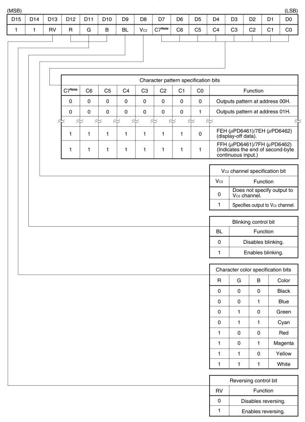
**Note** C7 bit is "don't care" at the  $\mu$ PD6462. However, this data sheet explains the  $\mu$ PD6462 with "0" in the C7 bit.
