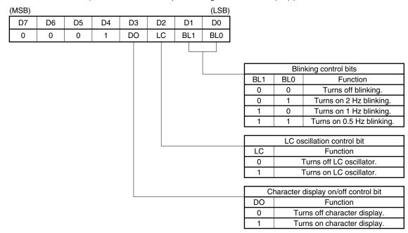
(2) For LSB-first transfer (Command bits are input starting from the LSB (D0). The function of each bit is the same as that for MSB-first transfer.)
