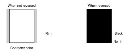
Display-off data does not change when reversed. When blank data is reversed, it becomes a solid character for which the character color is initially set. The character color can be set only for the RGB channel. It is always white (black when reversed) for the  $V_{C1}$  and  $V_{C2}$  channels.
