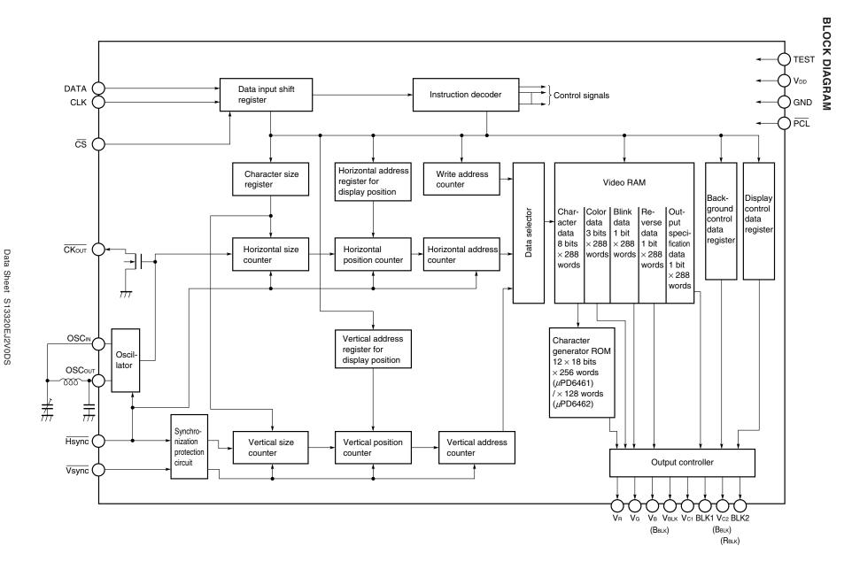
Remark Signals in ( ) are set by a mask option (RGB + RGB compatible blanking).
