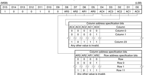
(2) For LSB-first transfer (Command bits are input starting from the LSB (D0). The function of each bit is the same as that for MSB-first transfer.)
