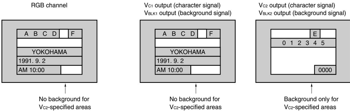
**Remarks 1.** The above figures are only examples. Actually, the background can be controlled independently for each output channel (only in RGB+Vc1+Vc2 mode), for example, by applying background (overall/minimum) for the RGB channel but not for the other channels.
