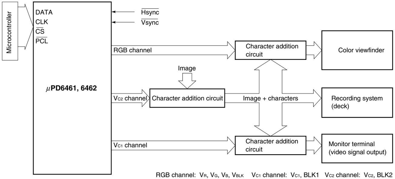
Example of application to a camcorder (2) (in RGB+3BLK mode for RGB compatible blanking)
