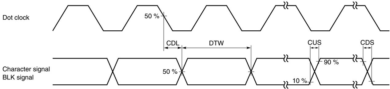
**OUTPUT TIMINGS** (T<sub>A</sub> = -20 to +75°C, pins: V<sub>R</sub>, V<sub>G</sub>, V<sub>B</sub>, V<sub>BLK</sub>, V<sub>C1</sub>, BLK1, V<sub>C2</sub>, BLK2, (R<sub>BLK</sub>, G<sub>BLK</sub>, B<sub>BLK</sub>))
