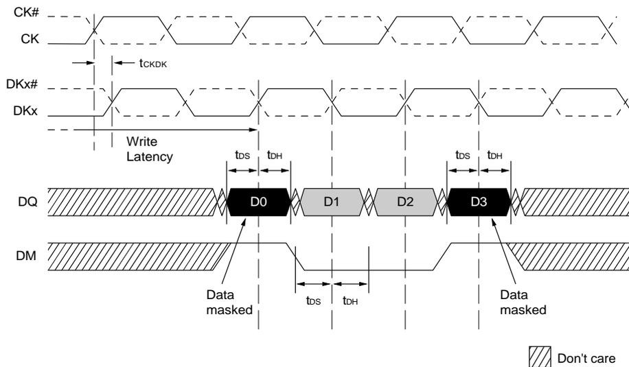
Figure 2-8. WRITE Burst Basic Sequence: BL=2, RL=4, WL=5, Configuration 1
