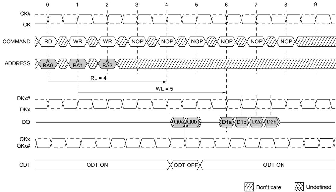
Figure 2-25. WRITE followed by READ with ODT: BL=2, Configuration 1
