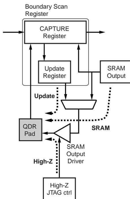
Boundary Scan Register Status of Output Pins CQ, CQ# and Q
