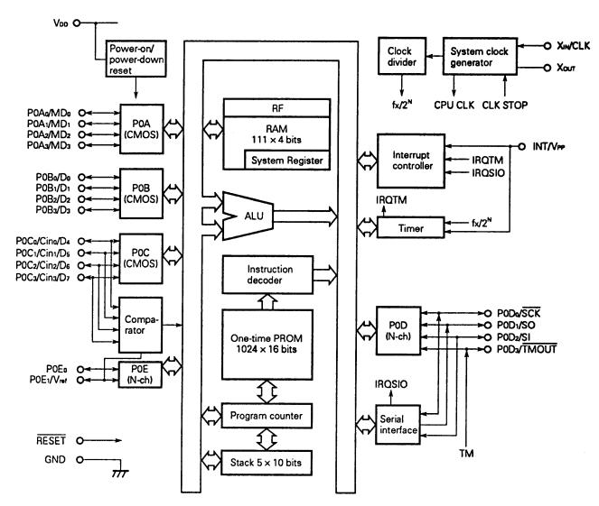
Remark The terms CMOS and N-ch in parentheses indicate the output form of the port.
