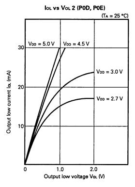
Caution The absolute maximum rating of the current is 30 mA per pin. The input voltage or output voltage of the P0E1 pin must not be higher than Voo + 0.3 V.
