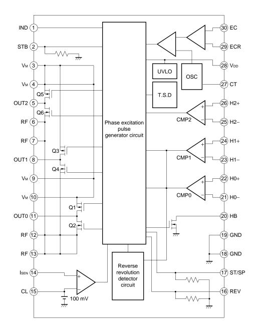
Remarks 1. The CL pin is used to connect a filter. Leave this pin open when it is not used.
