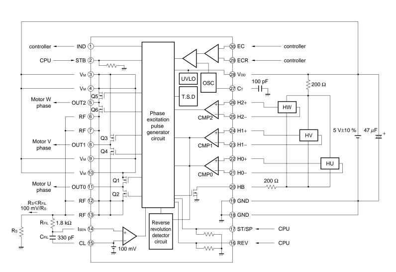
Caution  $\,$  It is recommended that a tantalum capacitor of several 10  $\mu F$  be inserted between V<sub>M</sub> and GND the rating. to reduce noise during PWM. Determine the value of Rs so that the output current does not exceed
