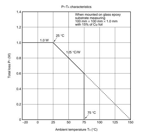
Caution If the ambient temperature is 25 °C or less, a power of up to 1 W can be applied. If the temperature rises beyond 25 °C, perform derating by referring to the above figure. At 75 °C, which is the maximum level of the recommended operating temperature, a power of up to 0.6 W can be applied to the IC.
