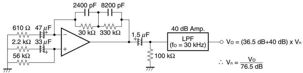
Fig.3 Flat Noise Measurement Circuit (FLAT+JIS A)
