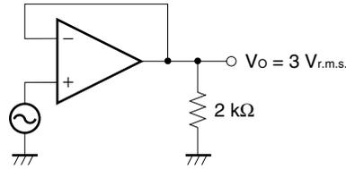
Fig.2 Noise Measurement Circuit (RIAA)
