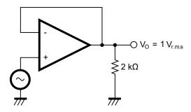
Figure 2: Noise Measurement Circuit (RIAA)
