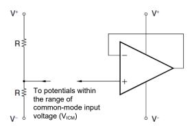
Remark: In this example, an intermediate potential between V + and V - is applied.
