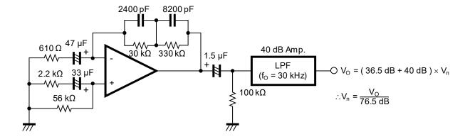
Figure 3: Noise Measurement Circuit (FLAT+JIS A)
