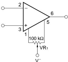
★ **Remark** The OFFSET NULL pins should be left open or connected to V<sup>-</sup> via a resistor as shown in the left figure. Don't connect to any lines other than V<sup>-</sup>, otherwise malfunction, degradation, or failure may occur.
