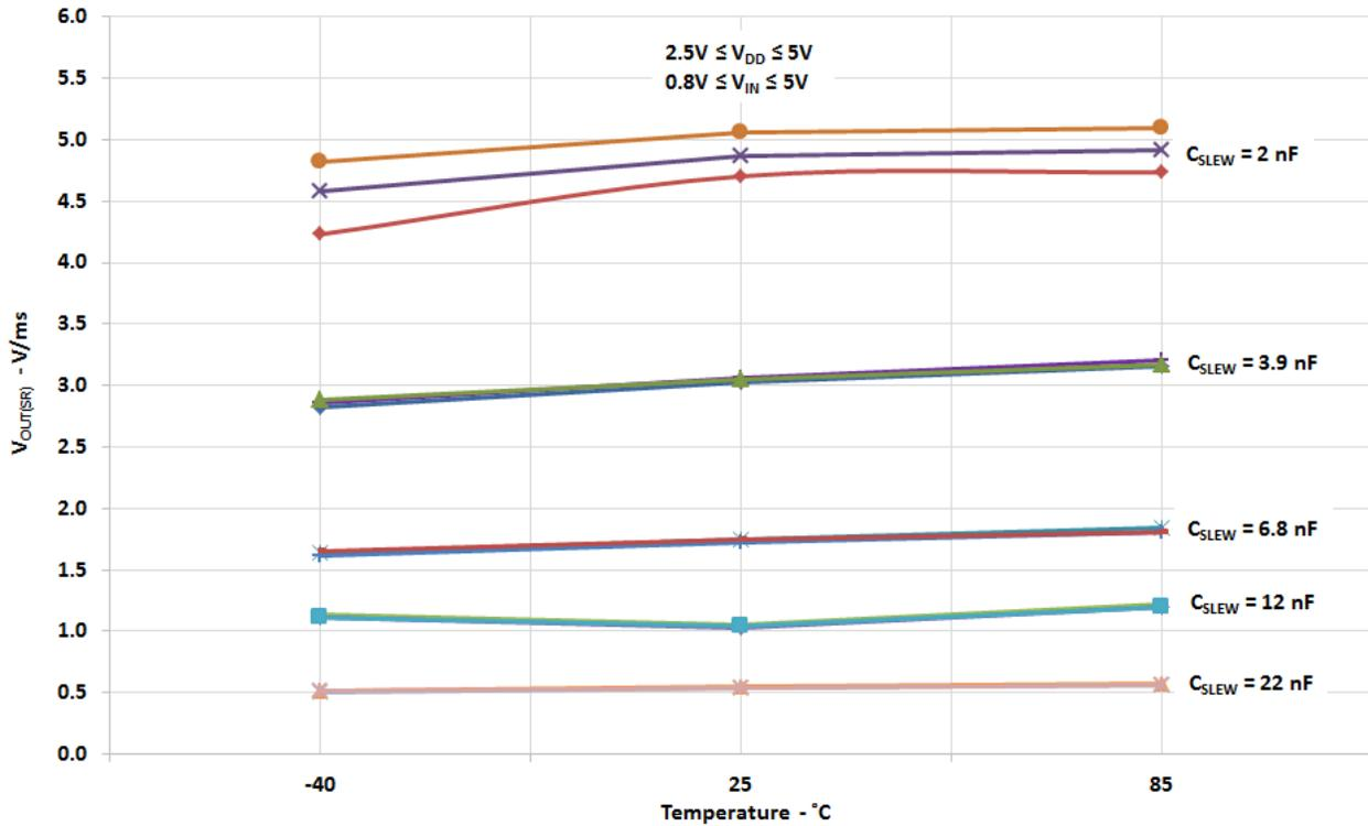
$V_{OUT(SR)}$  vs.  $C_{SLEW}$ ,  $V_{IN}$ ,  $V_{DD}$ , and Temperature
