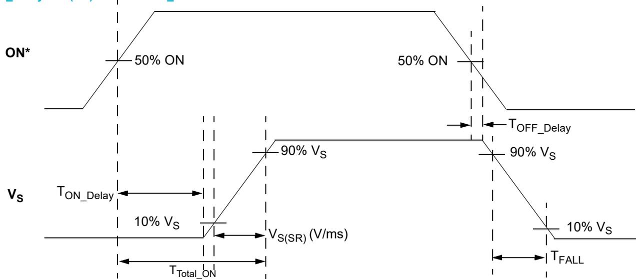
Note: \* Rise and Fall times of the ON signal are 100 ns
