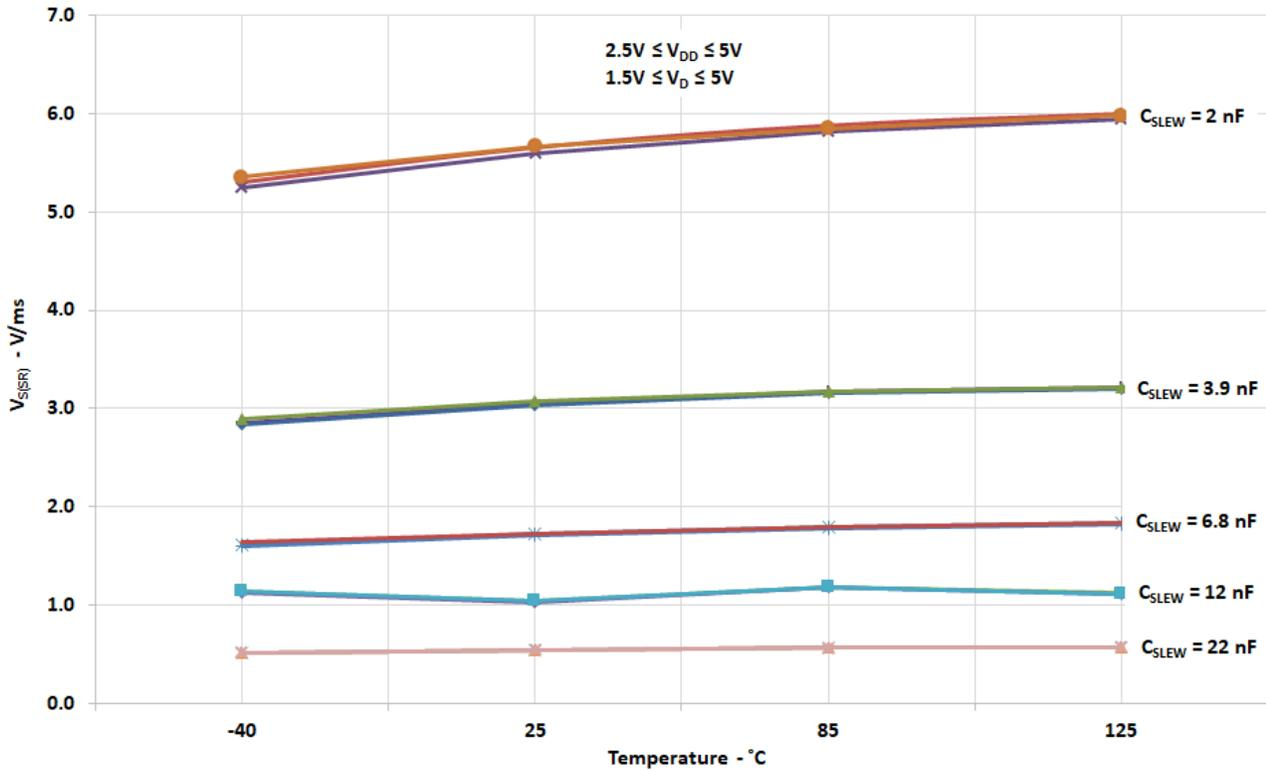
T<sub>Total ON</sub> vs. C<sub>SLEW</sub>, V<sub>D</sub>, V<sub>DD</sub>, and Temperature
