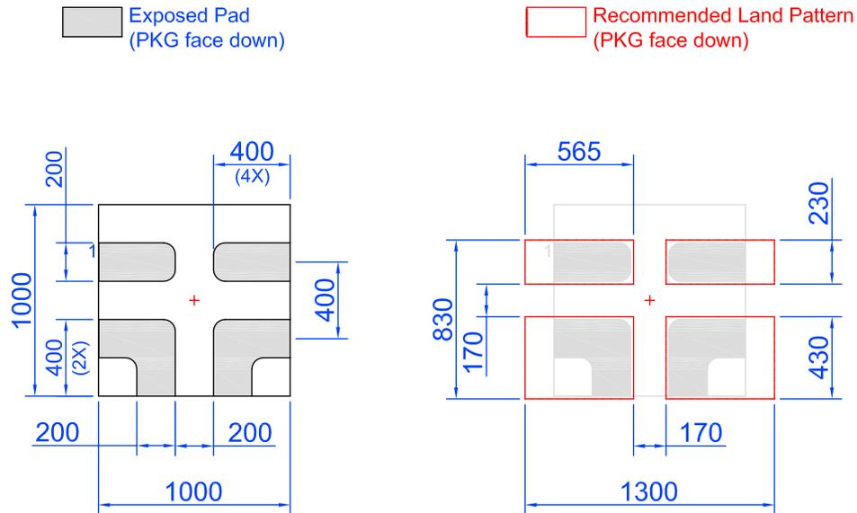
Note: All dimensions shown in micrometers (μm)
