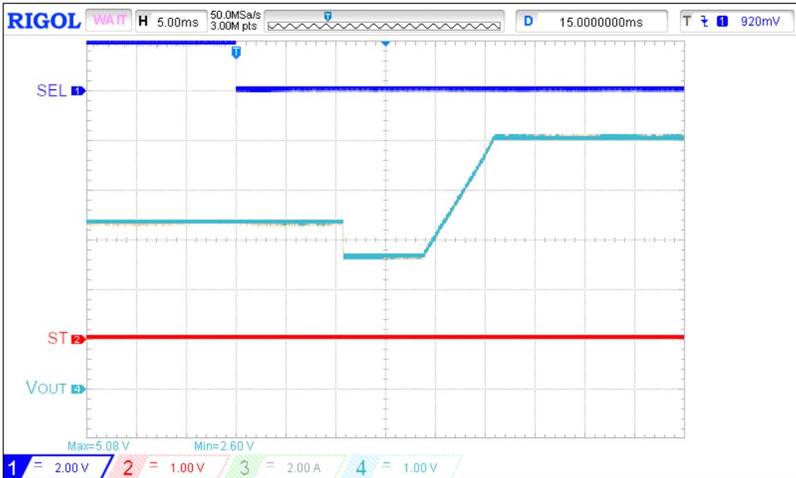
Figure 7. Switchover operation waveform for  $V_{IN1} = 5\text{ V}$ ,  $V_{IN2} = 3.3\text{ V}$ ,  $C_{SS} = 220\text{ nF}$ ,  $PR = 0\text{ V}$ ,  $SEL = \text{High} \rightarrow \text{Low}$ ,  $R_{LOAD} = 100\ \Omega$ ,  $C_{LOAD} = 2\ \mu\text{F}$  (extended view)
