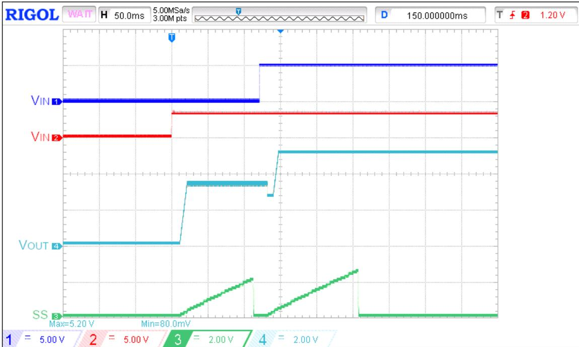
Figure 12. Higher voltage level priority operation waveform when IN1 is applied after first SS rise is done for  $V_{IN1} = 5\text{ V}$ ,  $V_{IN2} = 3.3\text{ V}$ ,  $SEL = 0\text{ V}$ ,  $PR = 0\text{ V}$ ,  $C_{SS} = 220\text{ nF}$ ,  $R_{LOAD} = 100\ \Omega$ ,  $C_{LOAD} = 2\ \mu\text{F}$
