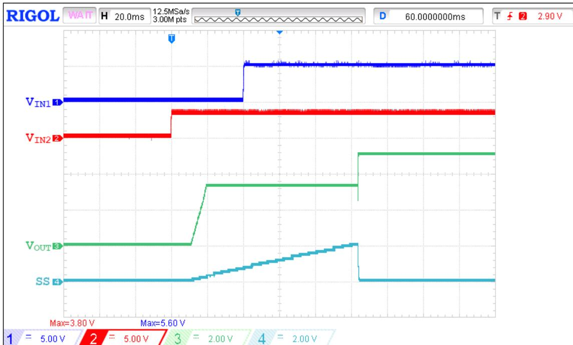
Figure 15. Higher voltage level priority operation waveform when IN1 is applied before first SS rise is done for  $V_{IN1} = 5\text{ V}$ ,  $V_{IN2} = 3.3\text{ V}$ ,  $SEL = 0\text{ V}$ ,  $PR = 0\text{ V}$ ,  $C_{SS} = 220\text{ nF}$ ,  $R_{LOAD} = 100\ \Omega$ ,  $C_{LOAD} = 2\ \mu\text{F}$
