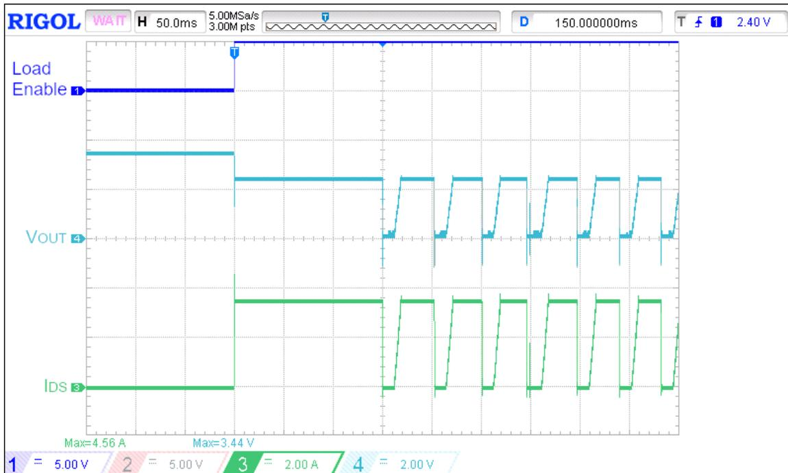
Figure 20. Active Current Limit operation waveform for  $V_{IN2} = 3.3\text{ V}$ ,  $C_{SS} = 220\text{ nF}$ ,  $R_{LIM} = 31.6\text{ k}\Omega$ ,  $R_{LOAD} = 0.66\ \Omega$ ,  $C_{LOAD} = 2\ \mu\text{F}$
