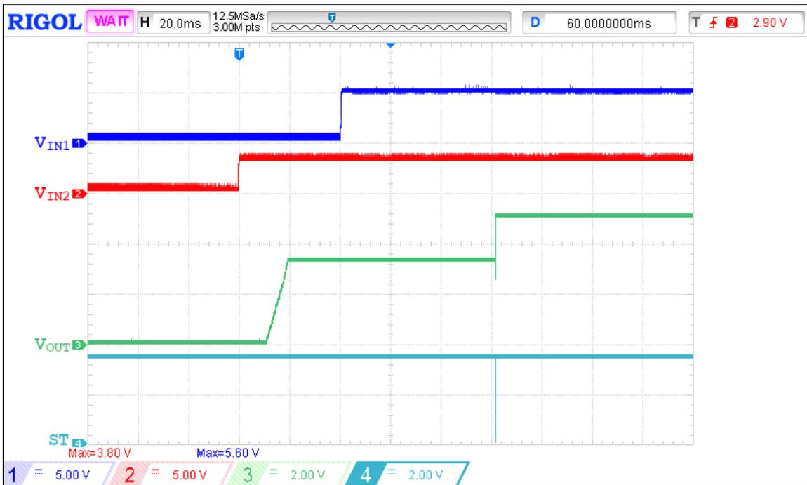
Figure 13. Higher voltage level priority operation waveform when IN1 is applied before first SS is done for  $V_{IN1} = 5\text{ V}$ ,  $V_{IN2} = 3.3\text{ V}$ ,  $SEL = 0\text{ V}$ ,  $PR = 0\text{ V}$ ,  $C_{SS} = 220\text{ nF}$ ,  $R_{LOAD} = 100\ \Omega$ ,  $C_{LOAD} = 2\ \mu\text{F}$
