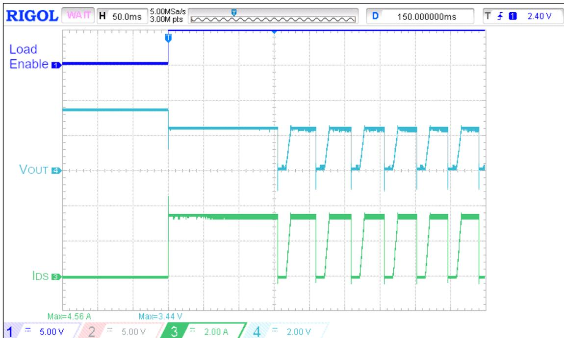
Figure 18. Active Current Limit operation waveform for  $V_{IN1} = 3.3 \text{ V}$ ,  $C_{SS} = 220 \text{ nF}$ ,  $R_{ILIM} = 31.6 \text{ k}\Omega$ ,  $R_{LOAD} = 0.66 \text{ }\Omega$ ,  $C_{LOAD} = 2 \text{ }\mu\text{F}$
