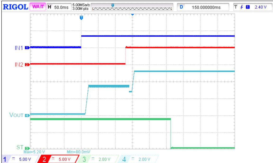
Figure 10. Higher voltage level priority operation waveform when IN2 is applied after first SS rise is done for  $V_{IN1} = 3.3\text{ V}$ ,  $V_{IN2} = 5\text{ V}$ ,  $SEL = 0\text{ V}$ ,  $PR = 0\text{ V}$ ,  $C_{SS} = 220\text{ nF}$ ,  $R_{LOAD} = 100\ \Omega$ ,  $C_{LOAD} = 2\ \mu\text{F}$
