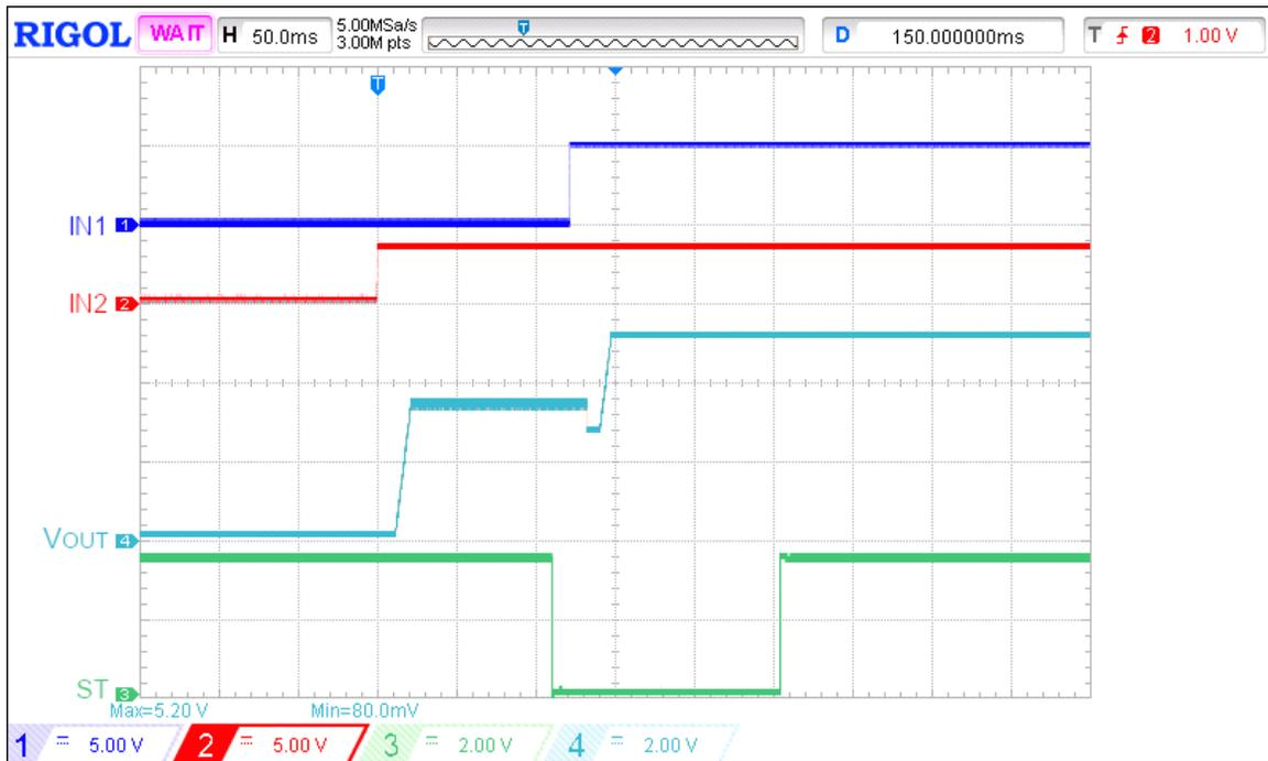
Figure 11. Higher voltage level priority operation waveform when IN1 is applied after first SS rise is done for  $V_{IN1} = 5\text{ V}$ ,  $V_{IN2} = 3.3\text{ V}$ ,  $SEL = 0\text{ V}$ ,  $PR = 0\text{ V}$ ,  $C_{SS} = 220\text{ nF}$ ,  $R_{LOAD} = 100\ \Omega$ ,  $C_{LOAD} = 2\ \mu\text{F}$
