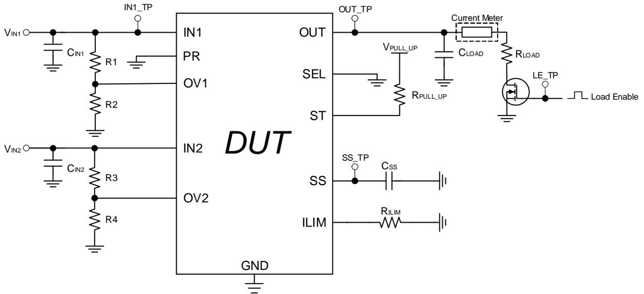
Figure 17. Test setup for Active Current Limit Operation
