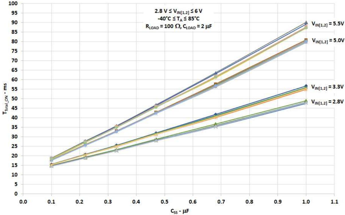
$V_{OUT}$  Slew Rate vs  $C_{SS}$ ,  $V_{IN[1,2]}$ , and Temperature
