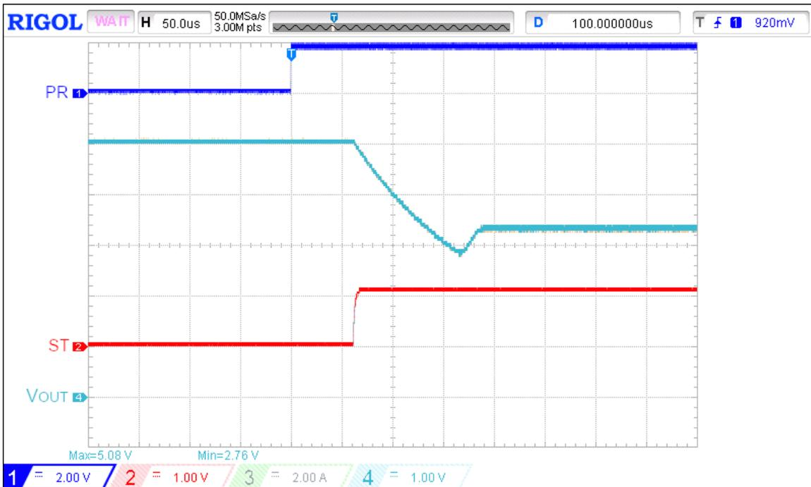
Figure 8. Switchover operation waveform for  $V_{IN1} = 3.3\text{ V}$ ,  $V_{IN2} = 5\text{ V}$ ,  $C_{SS} = 220\text{ nF}$ ,  $SEL = 0\text{ V}$ ,  $PR = \text{Low} \rightarrow \text{High}$ ,  $R_{LOAD} = 100\ \Omega$ ,  $C_{LOAD} = 2\ \mu\text{F}$
