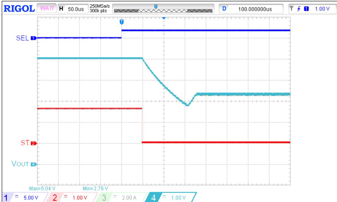
Figure 5. Switchover operation waveform for  $V_{IN1} = 5\text{ V}$ ,  $V_{IN2} = 3.3\text{ V}$ ,  $C_{SS} = 220\text{ nF}$ ,  $PR = 0\text{ V}$ ,  $SEL = \text{Low} \rightarrow \text{High}$ ,  $R_{LOAD} = 100\ \Omega$ ,  $C_{LOAD} = 2\ \mu\text{F}$
