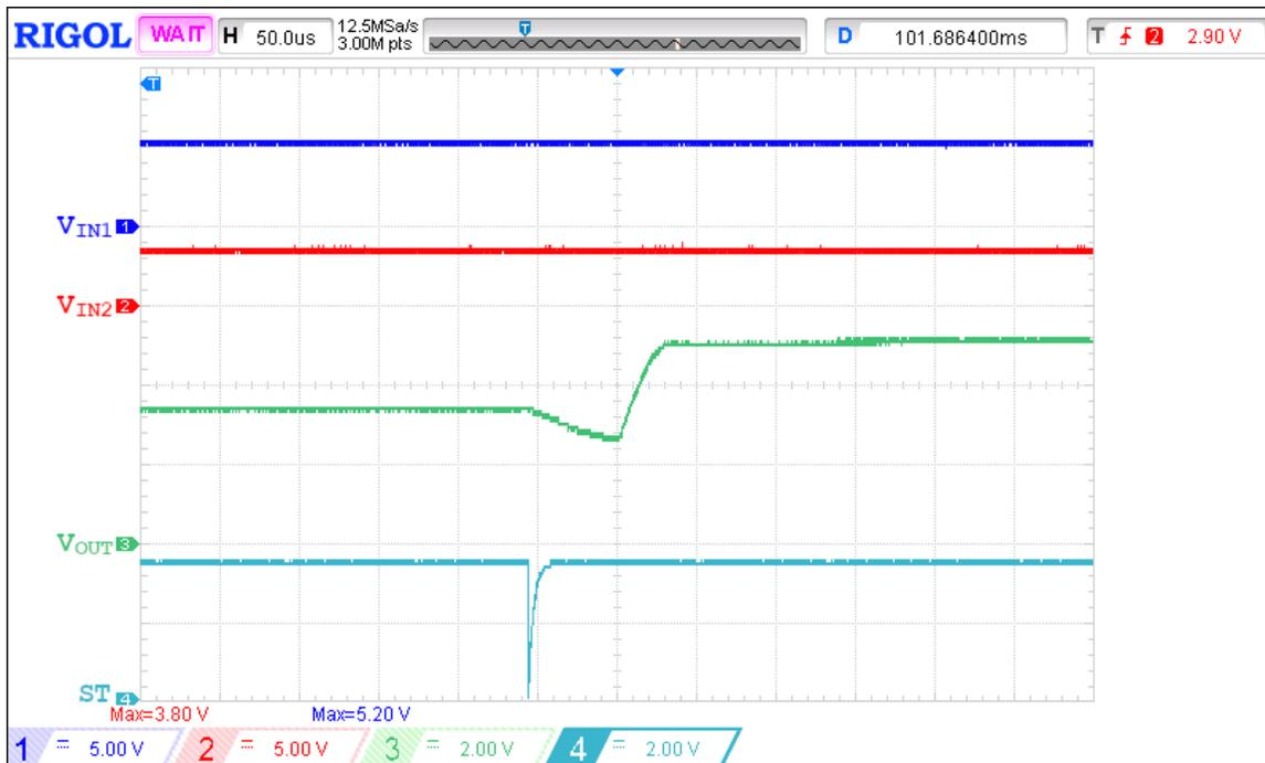
Figure 14. Higher voltage level priority operation waveform when IN1 is applied before first SS rise is done for  $V_{IN1} = 5\text{ V}$ ,  $V_{IN2} = 3.3\text{ V}$ ,  $SEL = 0\text{ V}$ ,  $PR = 0\text{ V}$ ,  $C_{SS} = 220\text{ nF}$ ,  $R_{LOAD} = 100\ \Omega$ ,  $C_{LOAD} = 2\ \mu\text{F}$  (extended view)
