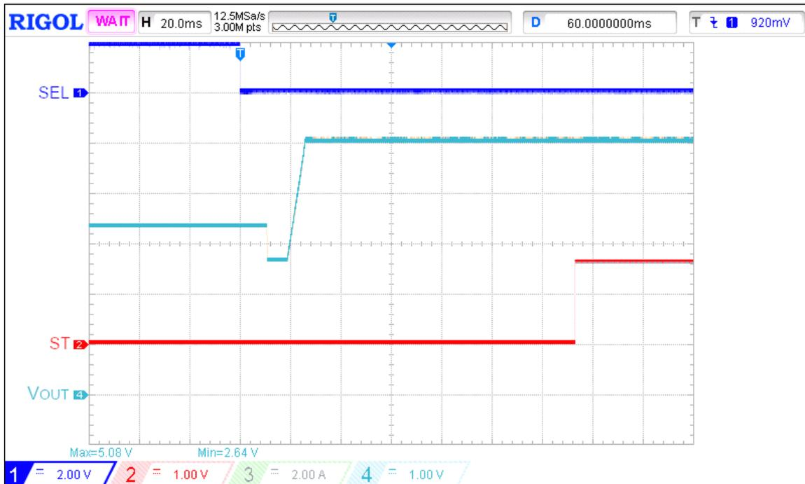
Figure 6. Switchover operation waveform for  $V_{IN1} = 5\text{ V}$ ,  $V_{IN2} = 3.3\text{ V}$ ,  $C_{SS} = 220\text{ nF}$ ,  $PR = 0\text{ V}$ ,  $SEL = \text{High} \rightarrow \text{Low}$ ,  $R_{LOAD} = 100\ \Omega$ ,  $C_{LOAD} = 2\ \mu\text{F}$
