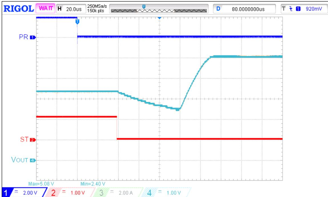
Figure 9. Switchover operation waveform for  $V_{IN1} = 3.3\text{ V}$ ,  $V_{IN2} = 5\text{ V}$ ,  $C_{SS} = 220\text{ nF}$ ,  $SEL = 0\text{ V}$ ,  $PR = \text{High} \rightarrow \text{Low}$ ,  $R_{LOAD} = 100\ \Omega$ ,  $C_{LOAD} = 2\ \mu\text{F}$
