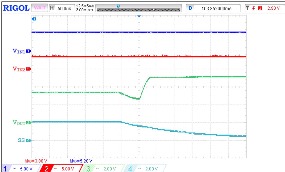
Figure 16. Higher voltage level priority operation waveform when IN1 is applied before first SS rise is done for V<sub>IN1</sub> = 5 V, V<sub>IN2</sub> = 3.3 V, SEL = 0 V, PR = 0 V, C<sub>SS</sub> = 220 nF, R<sub>LOAD</sub> = 100 Ω, C<sub>LOAD</sub> = 2 μF (extended view)
