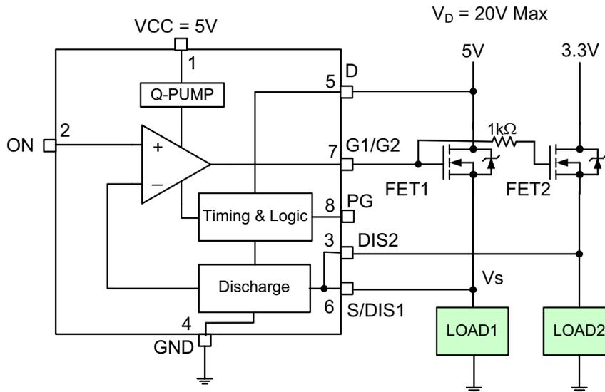
The highest  $V_D$  being switched must be at FET1 and pin 5 of the SLG55221 and SLG55220
