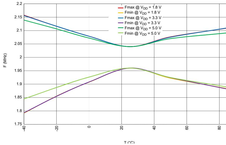
Figure 32. RC Oscillator Frequency vs. Temperature, RC OSC = 2 MHz
