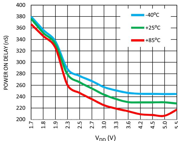
**Figure 29. Maximum Power-On Delay vs.  $V_{DD}$ , RC OSC = 2 MHz**
