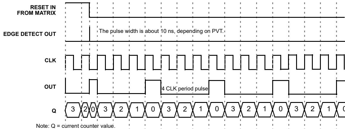
Figure 17. Timing (Reset Falling Edge Mode, Oscillator is Forced On) for Count Data = 3
