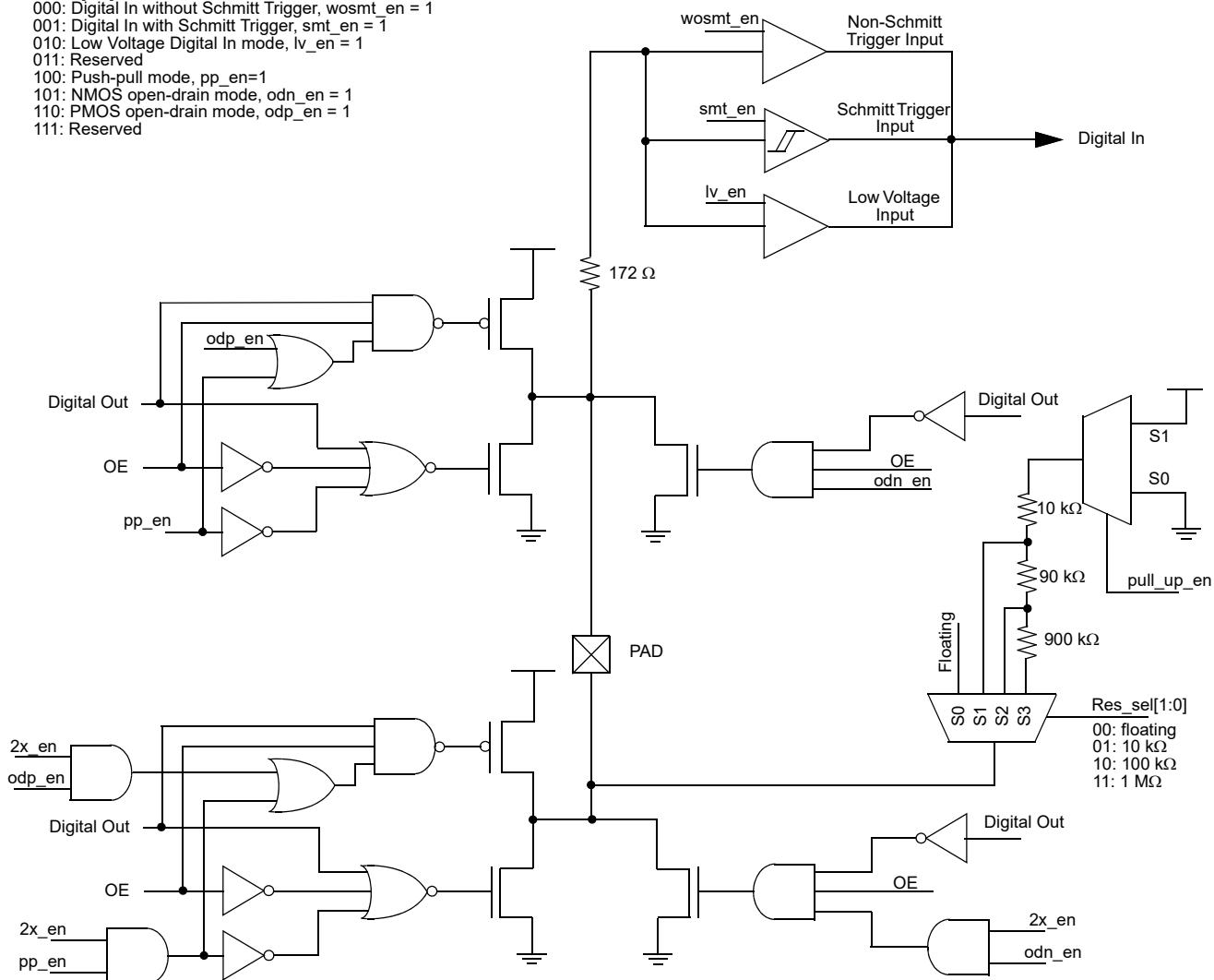
Figure 5. Register OE IO Structure Diagram
