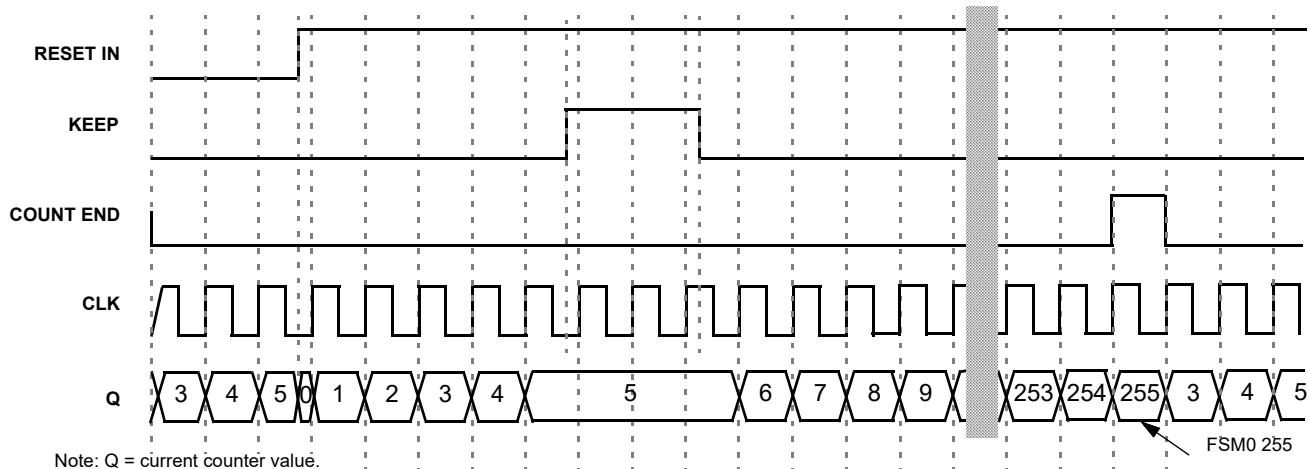
Figure 21. Timing (Reset Rising Edge Mode, Oscillator is Forced On, UP = 1) for Count Data = 3
