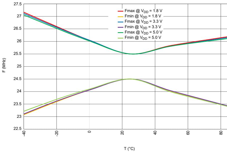
Figure 33. RC Oscillator Frequency vs. Temperature, RC OSC = 25 kHz
