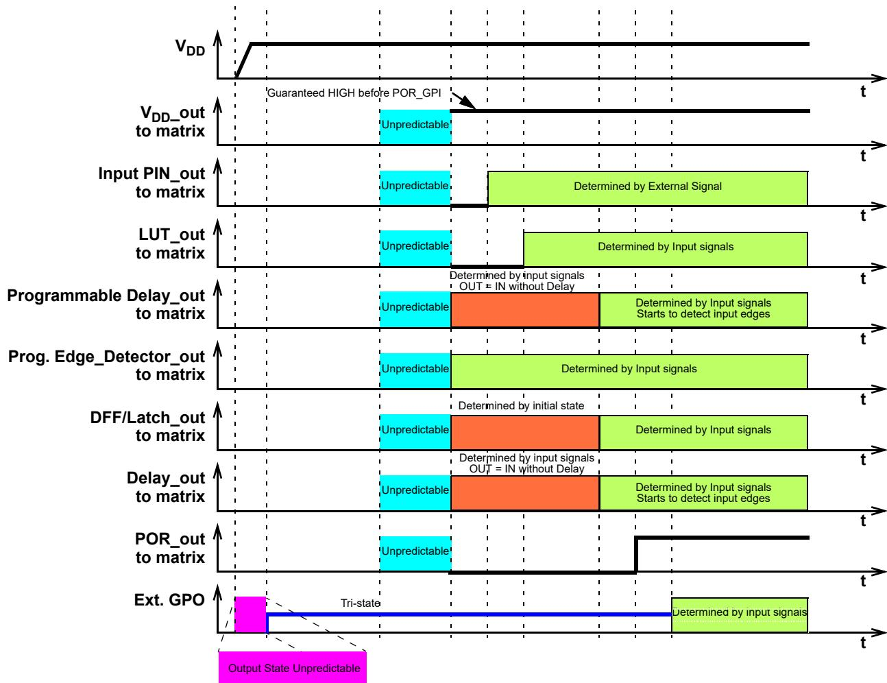
Figure 35. Internal Macrocell States during POR Sequence
