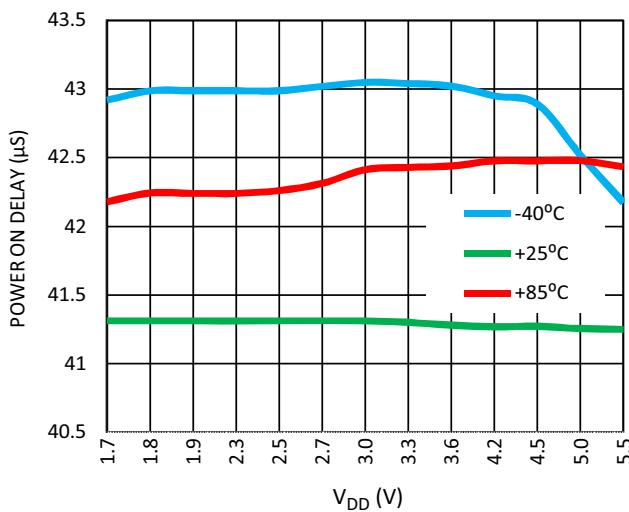
**Figure 30. Maximum Power-On Delay vs. V<sub>DD</sub>, RC OSC = 25 kHz**
