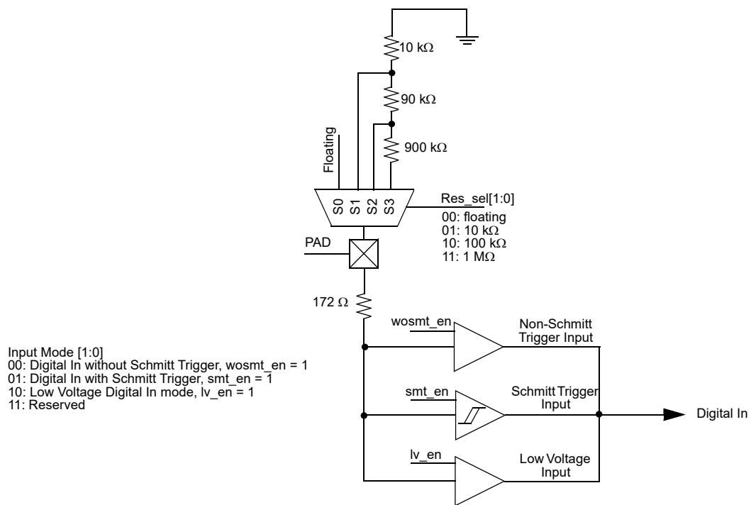
Figure 3. Pin 2 GPIO IO Structure Diagram
