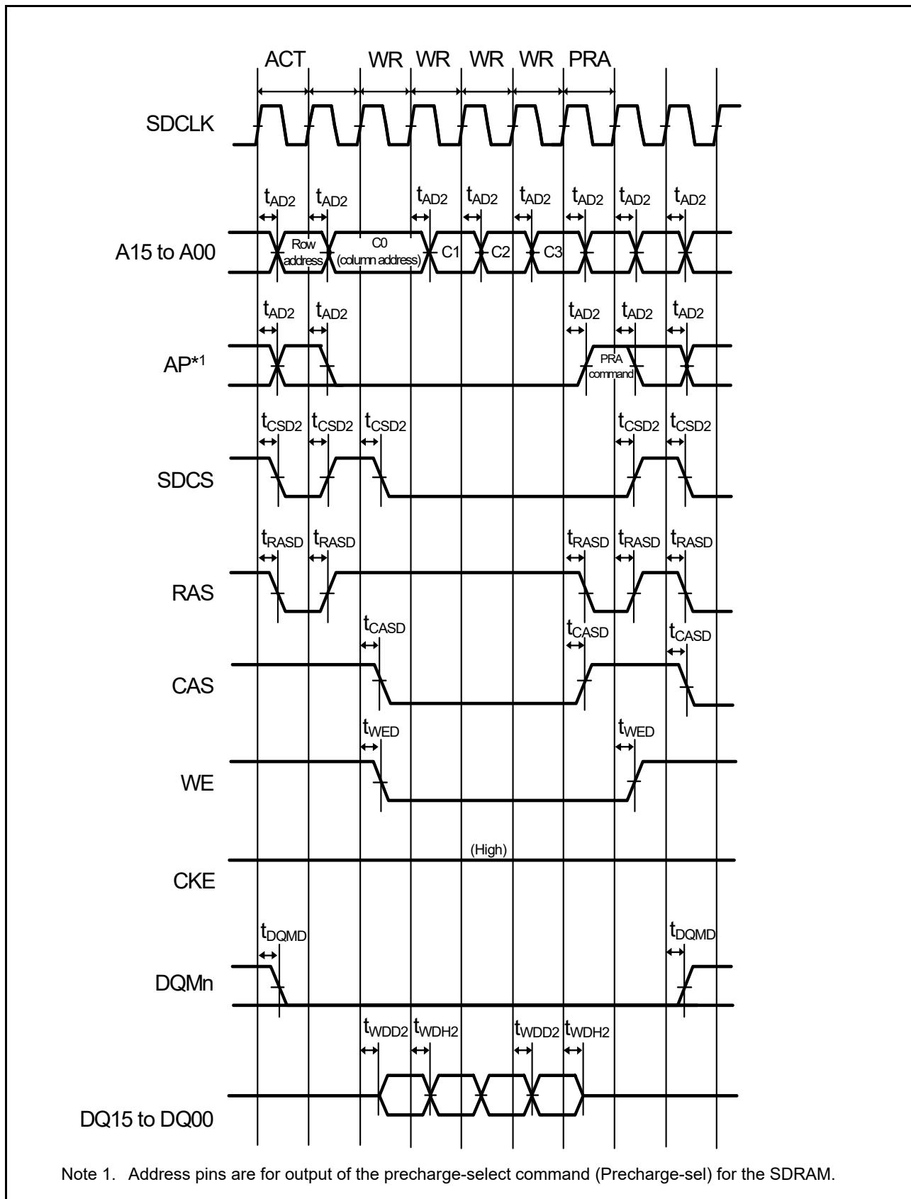
Figure 2.24 SDRAM multiple write timing
