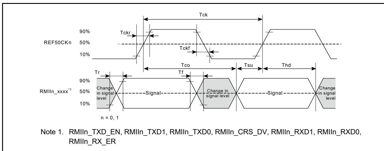
Figure 2.60 REF50CKn and RMII signal timing ( $n = 0$  and  $1$ )
