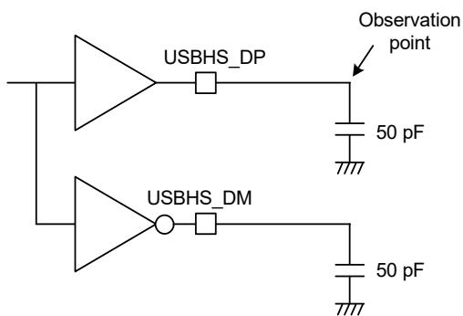
Figure 2.79 Test circuit in full-speed mode
