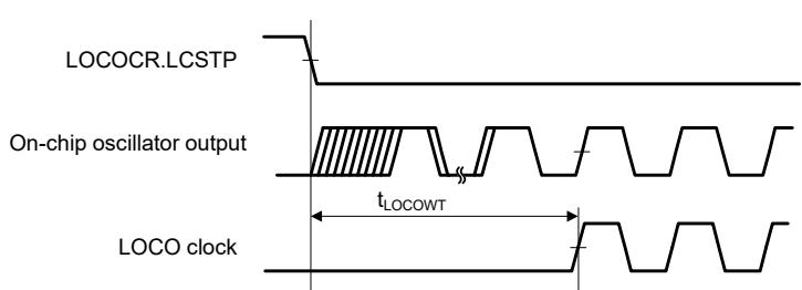
**Figure 2.6 LOCO clock oscillation start timing**
