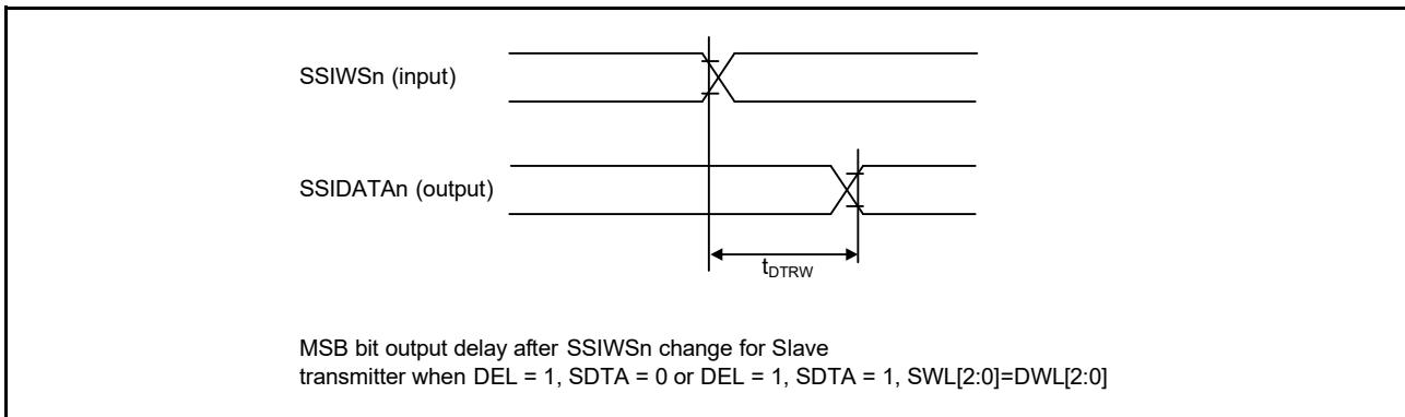
**Figure 2.58** SSI data output delay after SSIWSn change
