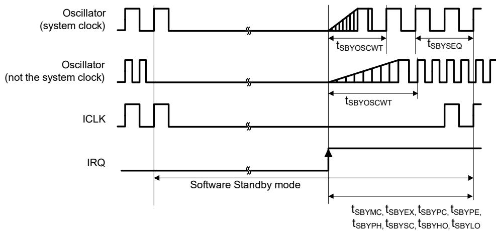
**When stabilization of an oscillator other than the system clock is slower**
