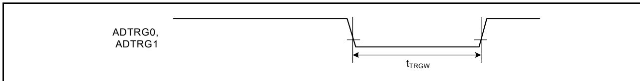
Figure 2.35 ADC12 trigger input timing
