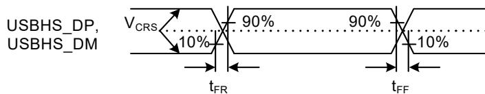
Figure 2.78 USBHS\_DP and USBHS\_DM output timing in full-speed mode
