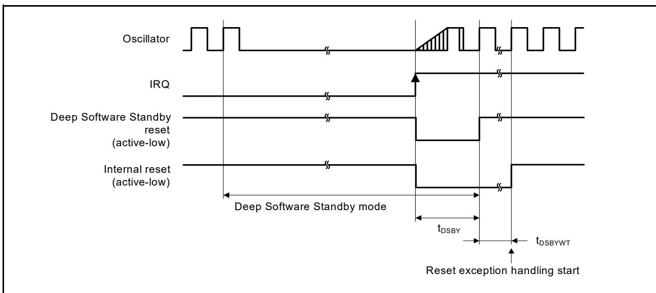
Figure 2.12 Deep Software Standby mode cancellation timing
