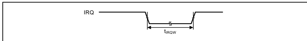
**Figure 2.15 IRQ interrupt input timing**
