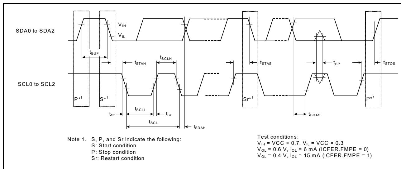
**Figure 2.54 I<sup>2</sup>C bus interface input/output timing**
