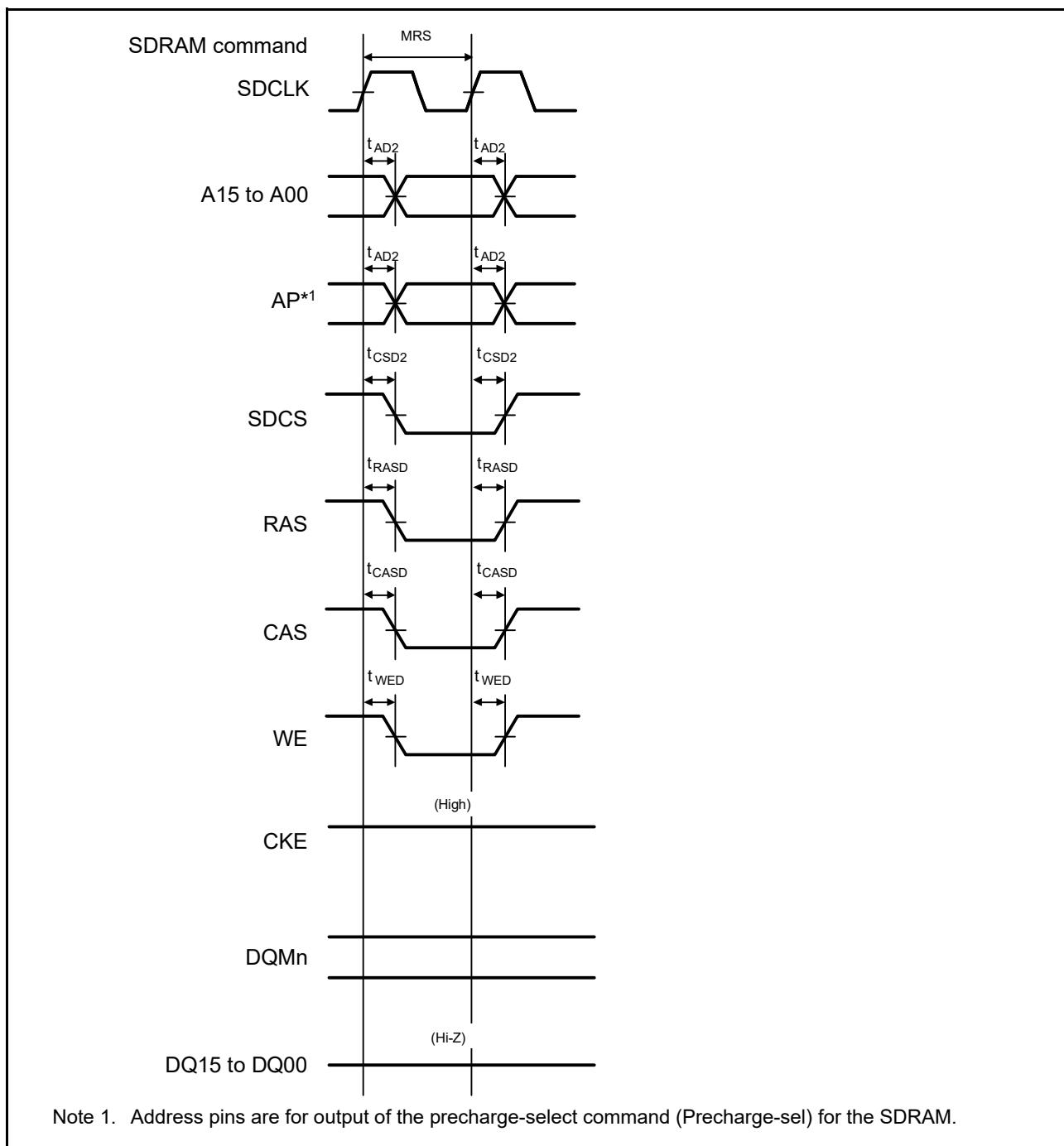
**Figure 2.26 SDRAM mode register set timing**
