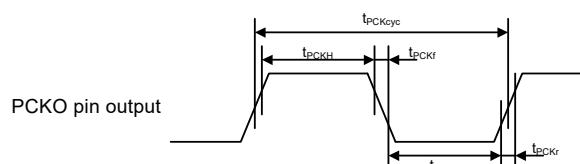
**Figure 2.71 PDC output clock timing**
