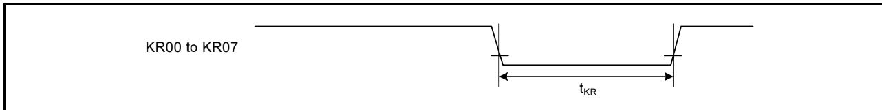
Figure 2.36 Key interrupt input timing
