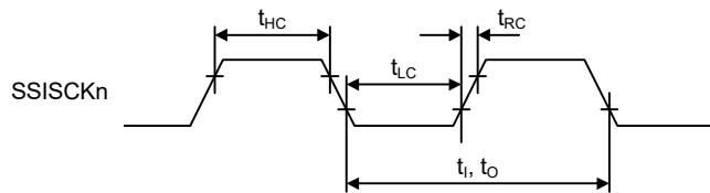
**Figure 2.55 SSI clock input/output timing**
