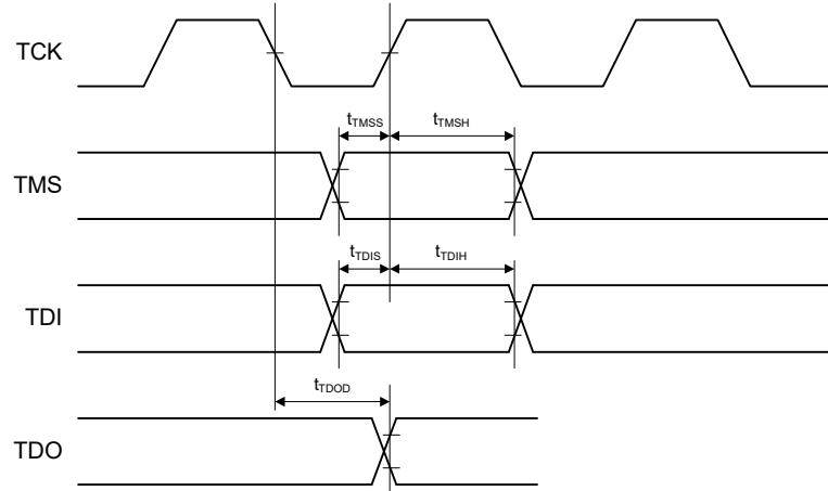
**Figure 2.97** Boundary scan input/output timing
