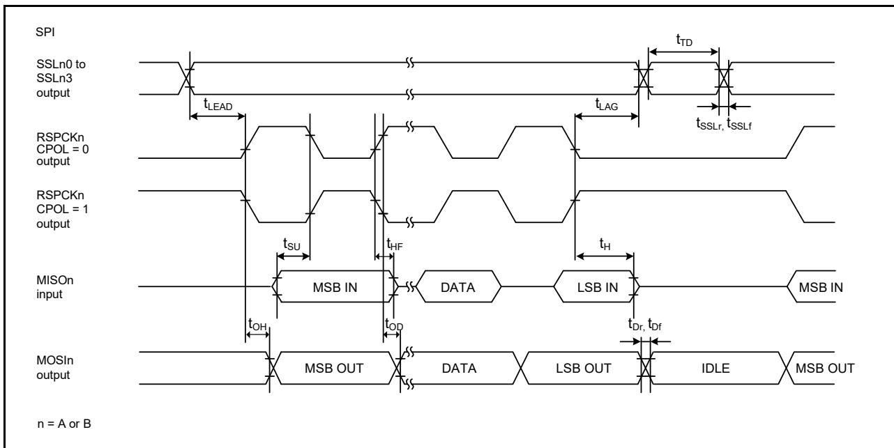
Figure 2.49 SPI timing for master when  $\text{CPHA} = 1$  and the bit rate is set to  $\text{PCLKA}/2$
