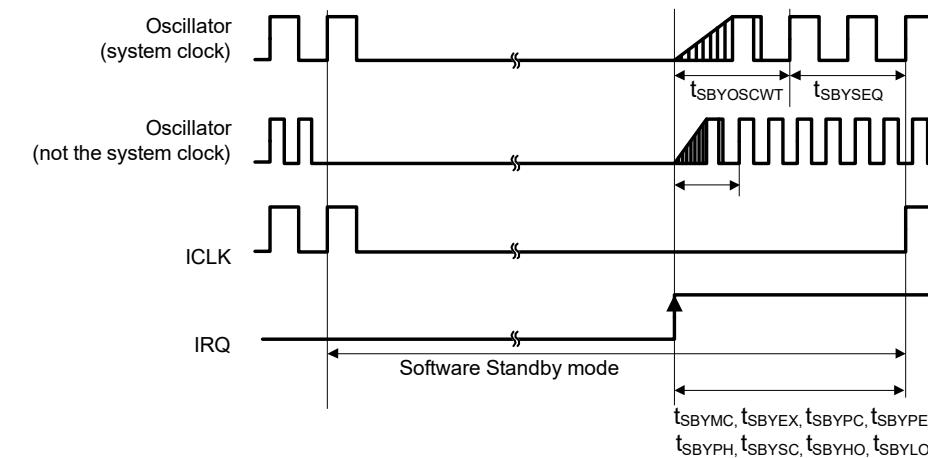
**When stabilization of the system clock oscillator is slower**
