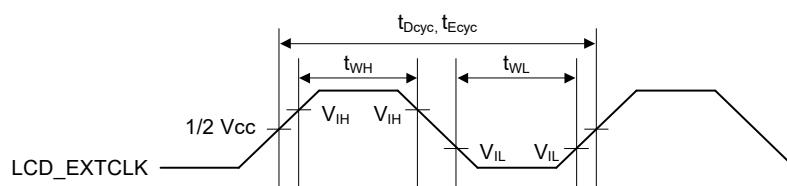
**Figure 2.73 LCD\_EXTCLK clock input timing**
