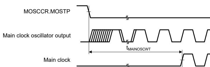
**Figure 2.5 Main clock oscillation start timing**
