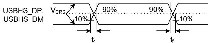
Figure 2.76 USBHS\_DP and USBHS\_DM output timing in low-speed mode
