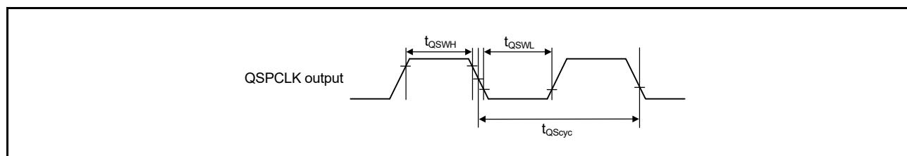
**Figure 2.52 QSPI clock timing**
