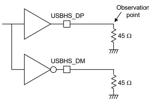
Figure 2.83 Test circuit in high-speed mode
