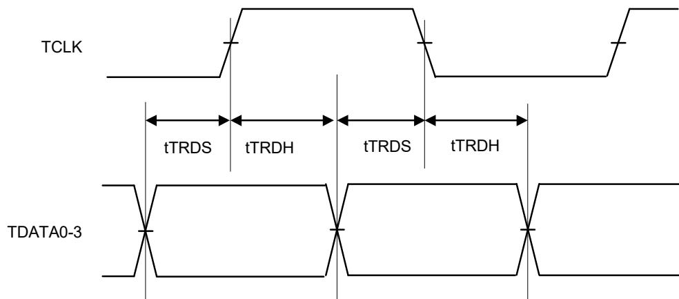
**Figure 2.104 ETM output timing**
