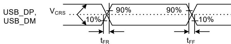
**Figure 2.86 USB\_DP and USB\_DM output timing in full-speed mode**
