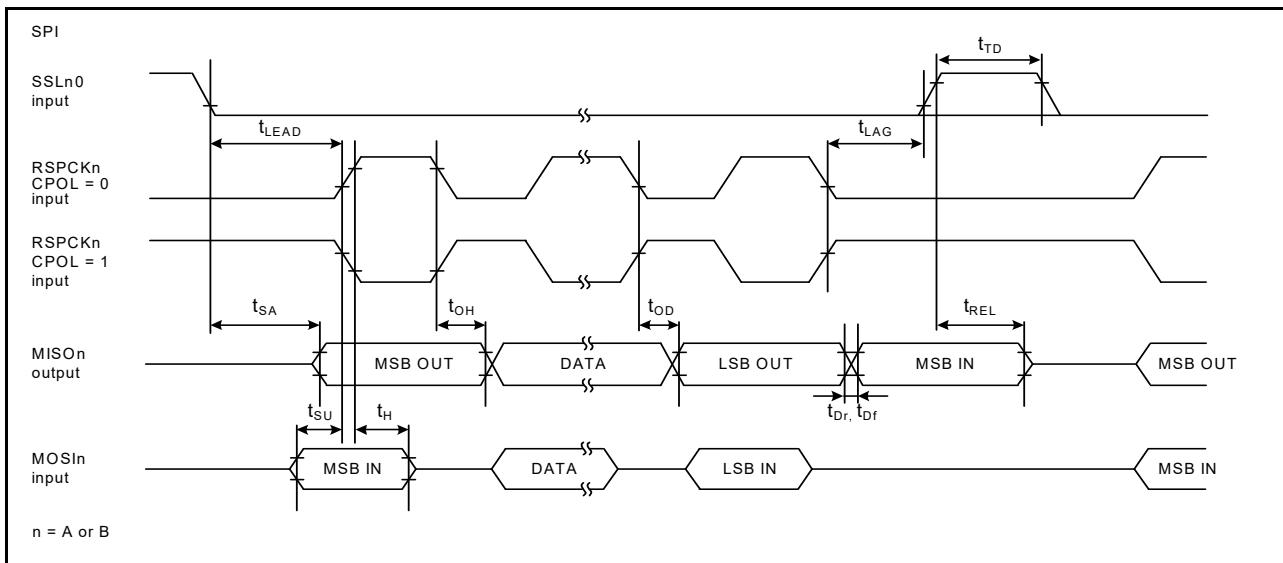
Figure 2.50 SPI timing for slave when CPHA = 0
