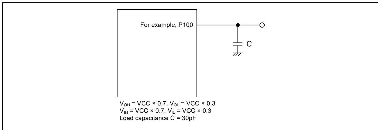
**Figure 2.1 Input or output timing measurement conditions**
