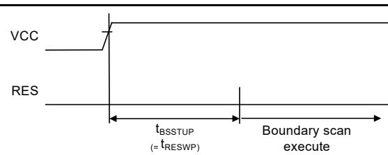
**Figure 2.98** Boundary scan circuit startup timing
