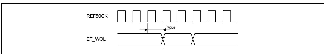
Figure 2.64 WOL output timing for RMII
