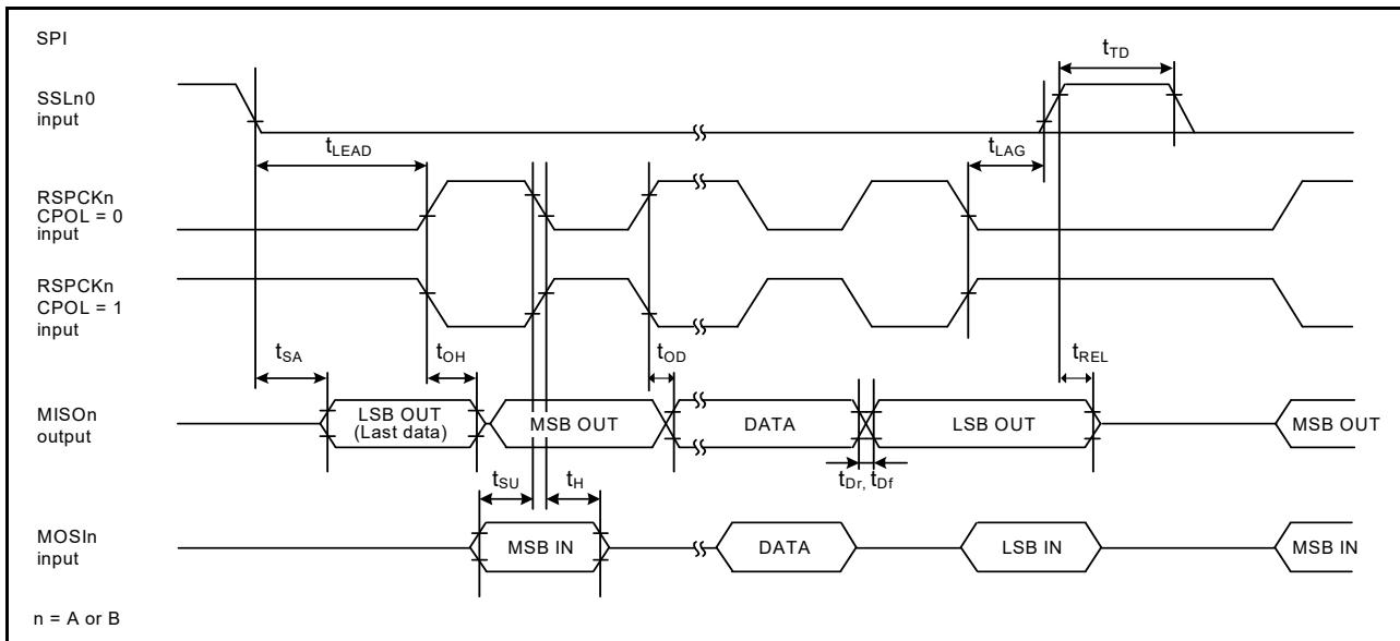
Figure 2.51 SPI timing for slave when CPHA = 1
