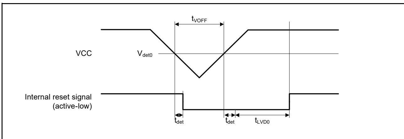
Figure 2.91 Voltage detection circuit timing ( $V_{det0}$ )
