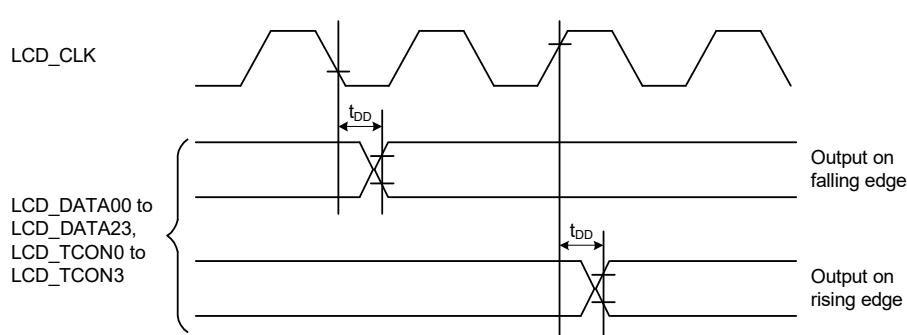
**Figure 2.75 Display output timing**
