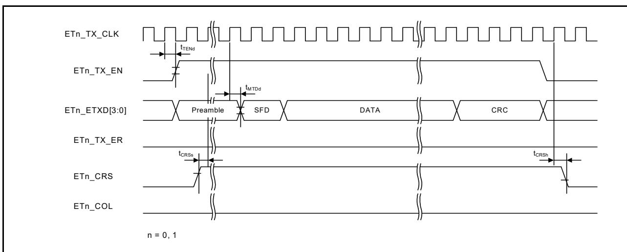
Figure 2.65 MII transmission timing in normal operation
