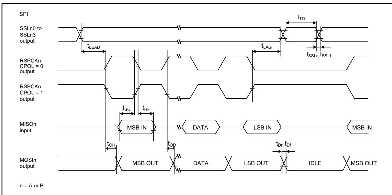
Figure 2.48 SPI timing for master when  $\text{CPHA} = 1$
