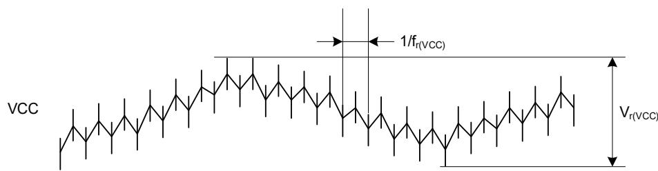
**Figure 2.2 Ripple waveform**
