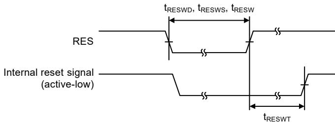
Figure 2.10 Reset input timing
