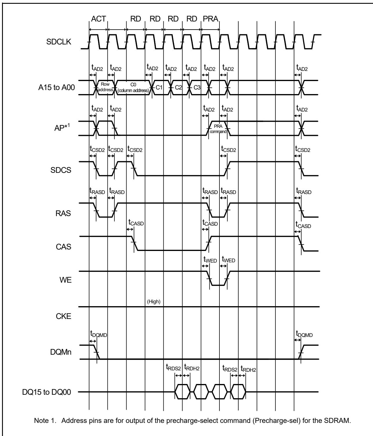
Figure 2.23 SDRAM multiple read timing
