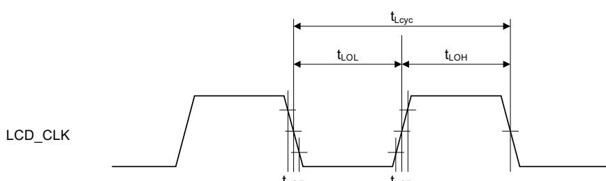
**Figure 2.74 LCD\_CLK clock output timing**
