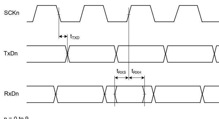
Figure 2.38 SCI input/output timing in clock synchronous mode
