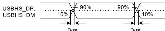
Figure 2.82 USBHS\_DP and USBHS\_DM output timing in high-speed mode
