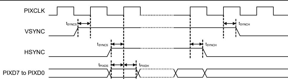
**Figure 2.72 PDC AC timing**
