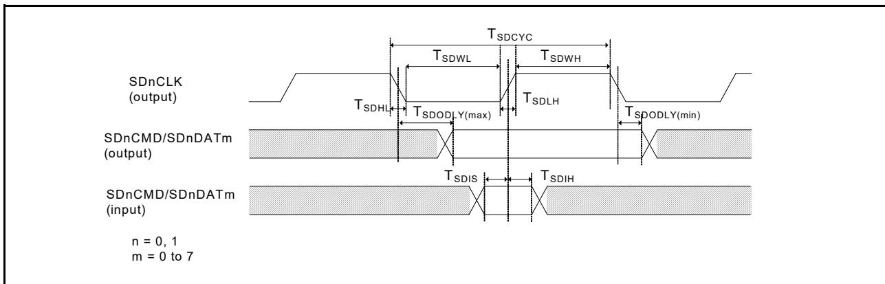
Figure 2.59 SD/MMC Host Interface signal timing
