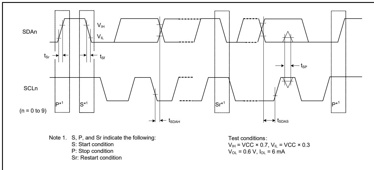
Figure 2.44 SCI simple IIC mode timing
