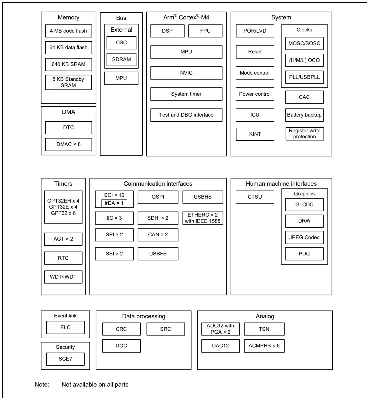
Figure 1.1 Block diagram
