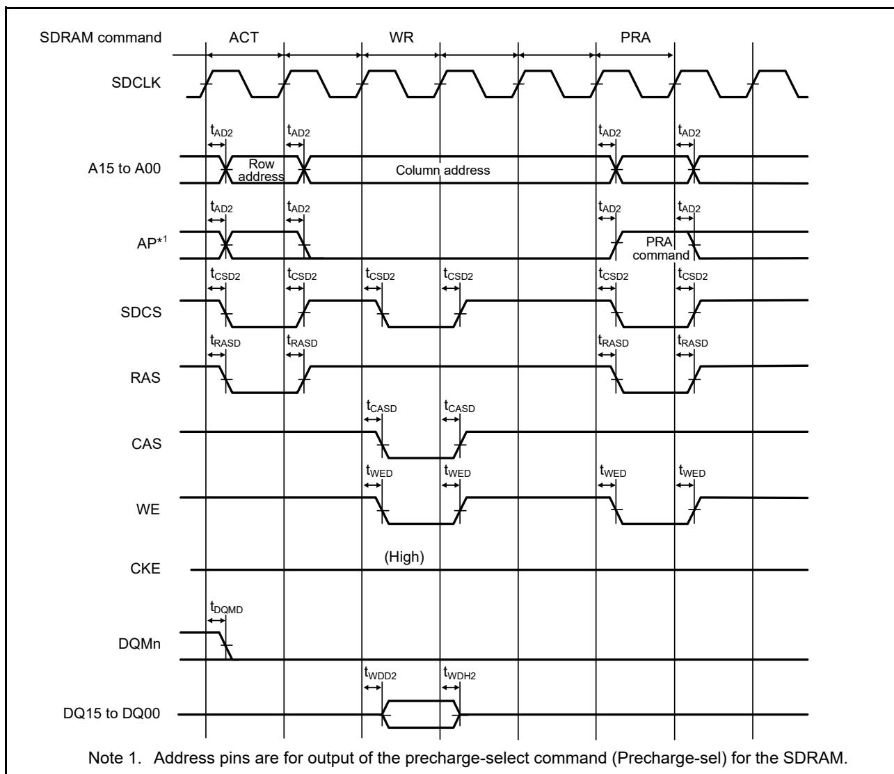
Figure 2.22 SDRAM single write timing
