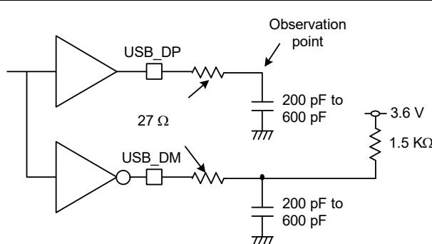
Figure 2.85 Test circuit in low-speed mode
