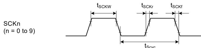
Figure 2.37 SCI clock input/output timing
