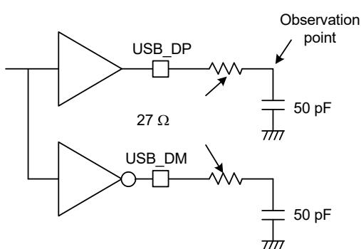
**Figure 2.87 Test circuit in full-speed mode**
