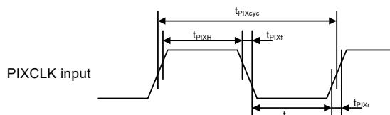
**Figure 2.70 PDC input clock timing**
