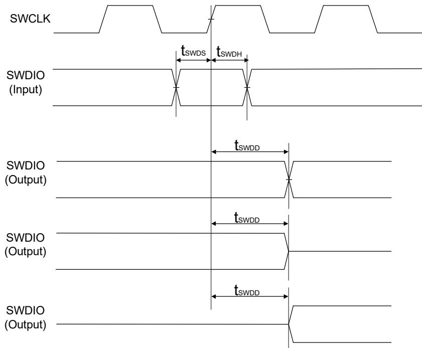
**Figure 2.102 SWD input/output timing**
