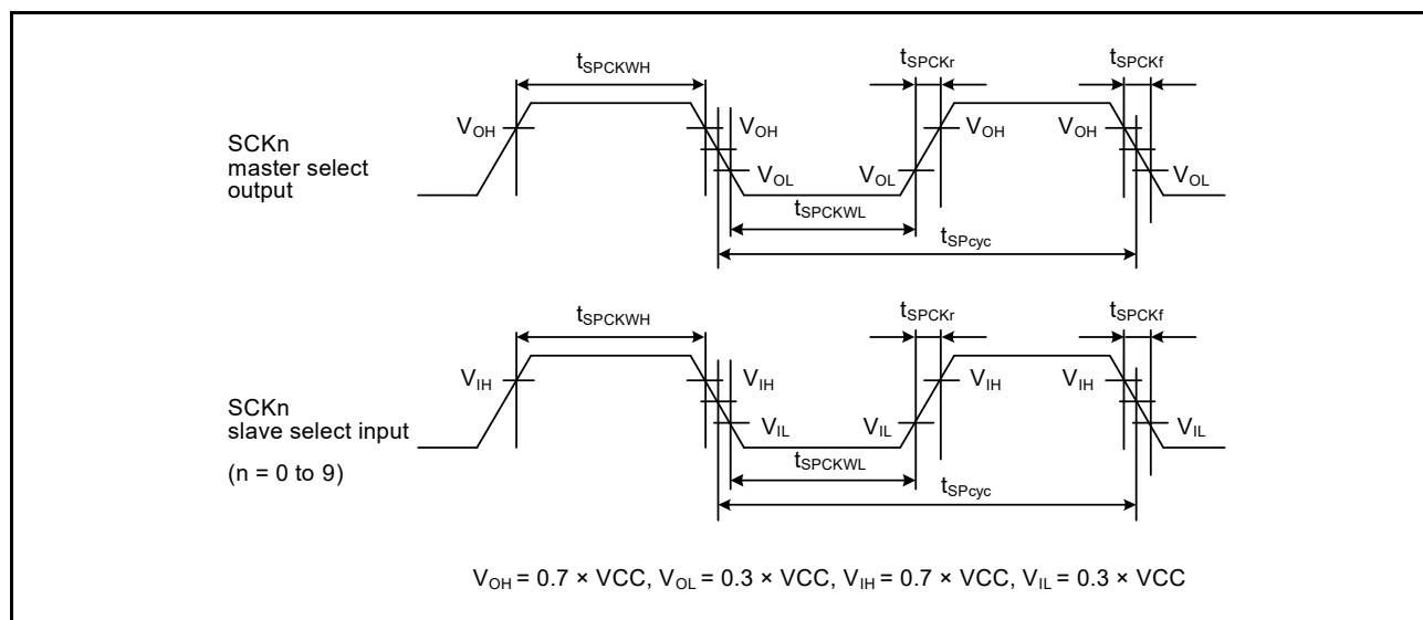
**Figure 2.39 SCI simple SPI mode clock timing**
