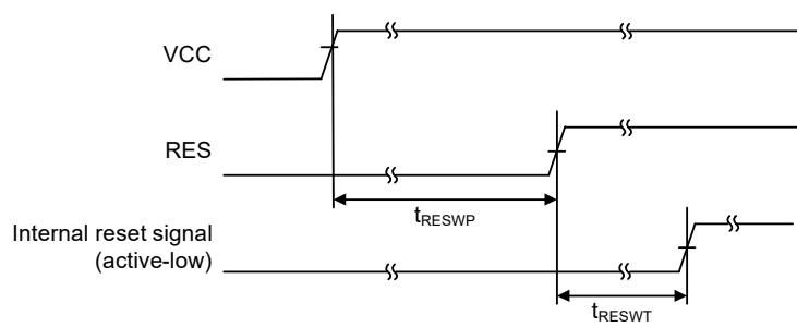
Figure 2.9 Power-on reset timing
