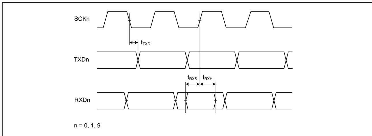
Figure 2.43 SCI input/output timing in clock synchronous mode
