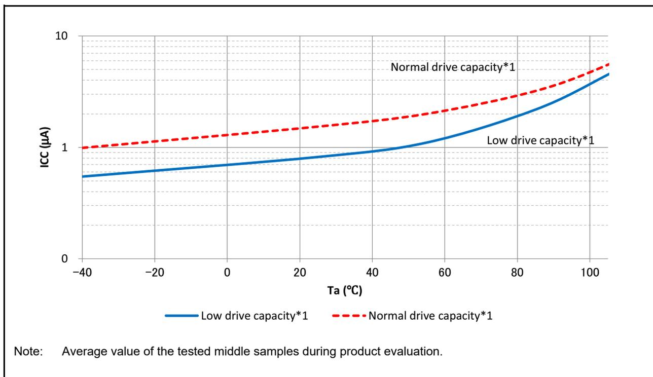
Figure 2.23 Temperature dependency of RTC operation (reference data)
