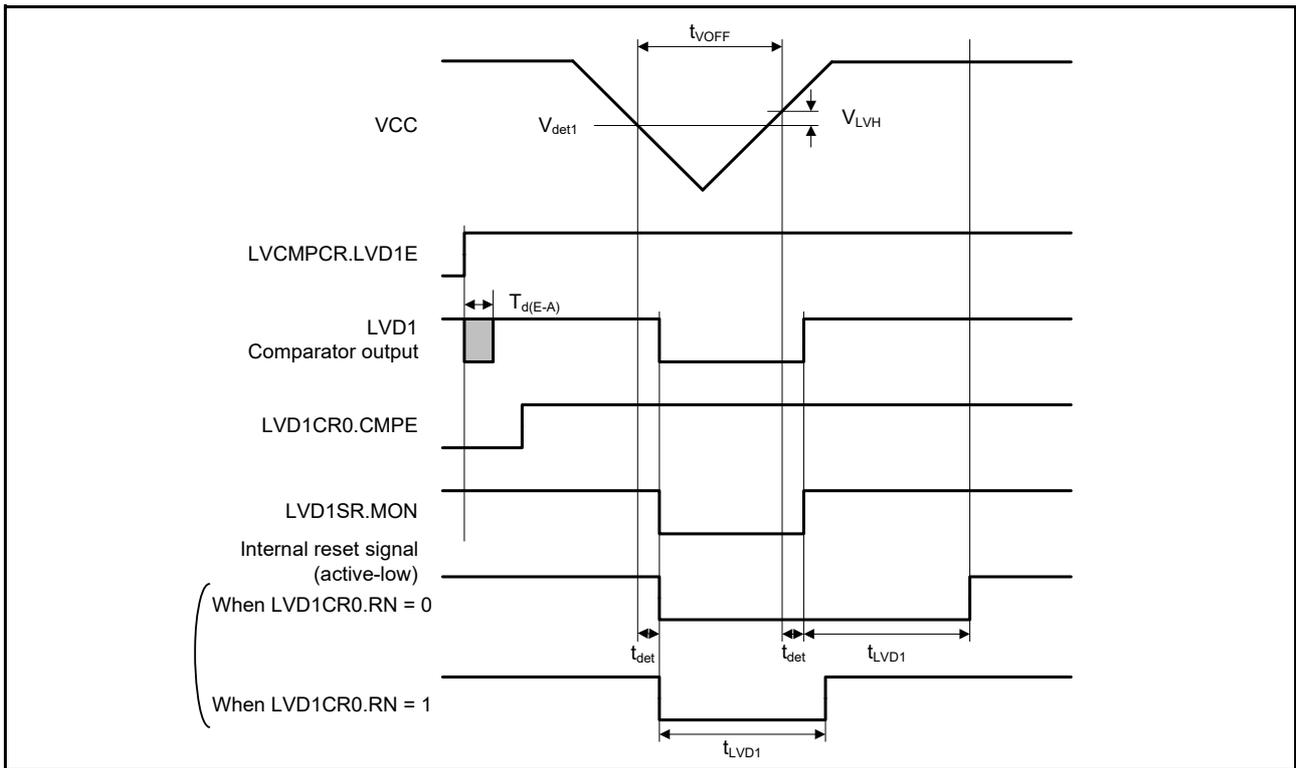
Figure 2.69 Voltage detection circuit timing (V<sub>det1</sub>)
