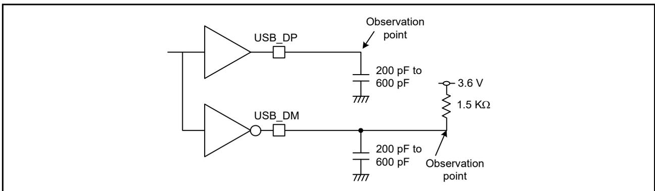
Figure 2.61 Test circuit for Low-Speed (LS) connection
