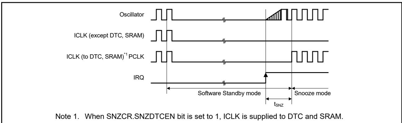
Figure 2.33 Recovery timing from Software Standby mode to Snooze mode
