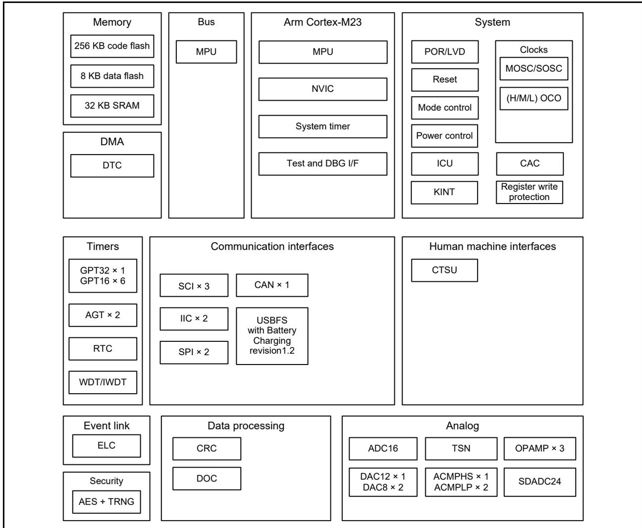
Figure 1.1 Block diagram
