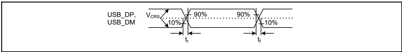
Figure 2.59 USB\_DP and USB\_DM output timing
