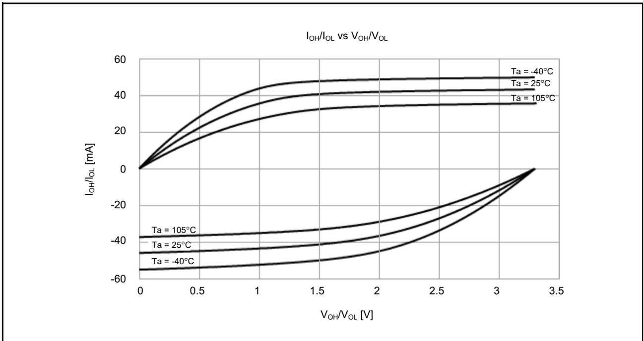
**Figure 2.10**  $V_{OH}/V_{OL}$  and  $I_{OH}/I_{OL}$  temperature characteristics at  $V_{CC} = 3.3$  V when middle drive output is selected (reference data, except for P914 and P915)
