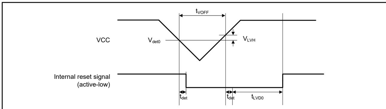
Figure 2.68 Voltage detection circuit timing ( $V_{det0}$ )
