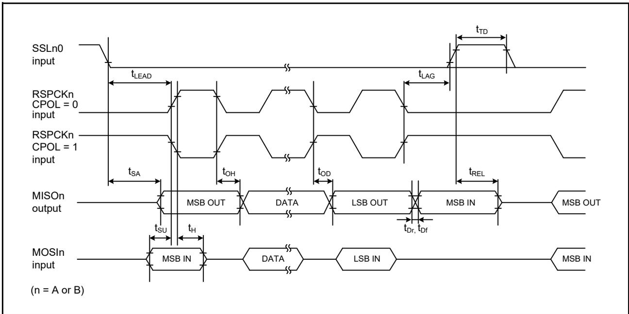
Figure 2.55 SPI timing (slave, CPHA = 0)
