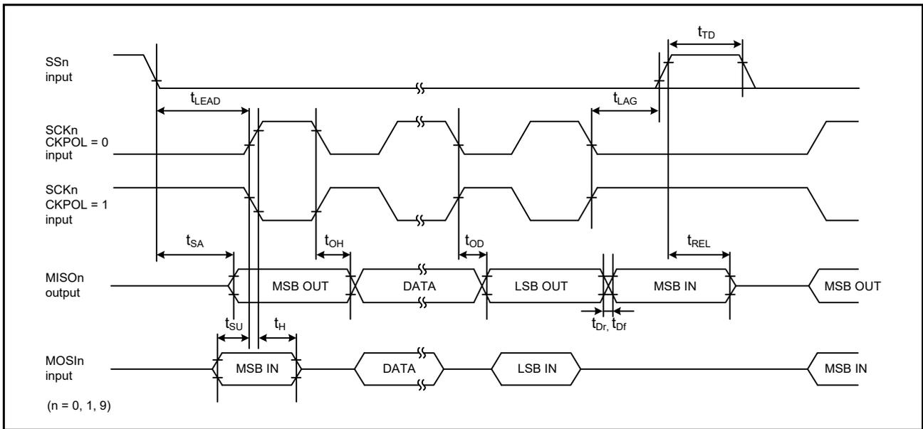
Figure 2.47 SCI simple SPI mode timing (slave, CKPH = 1)
