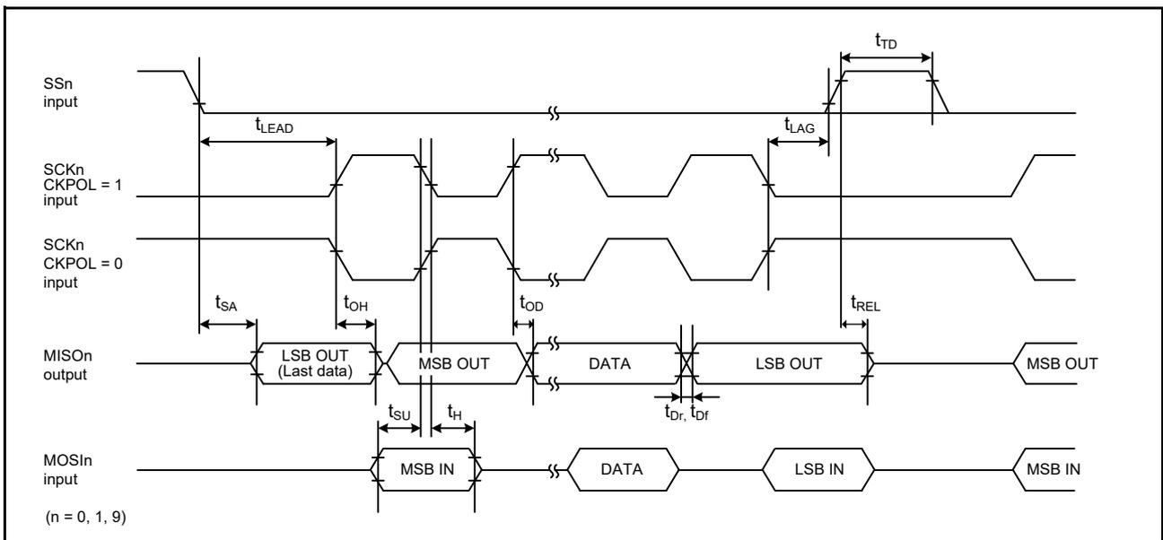
Figure 2.48 SCI simple SPI mode timing (slave, CKPH = 0)
