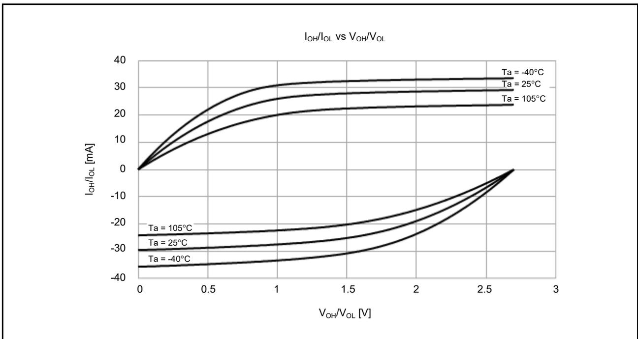
**Figure 2.9**  $V_{OH}/V_{OL}$  and  $I_{OH}/I_{OL}$  temperature characteristics at  $V_{CC} = 2.7$  V when middle drive output is selected (reference data, except for P914 and P915)
