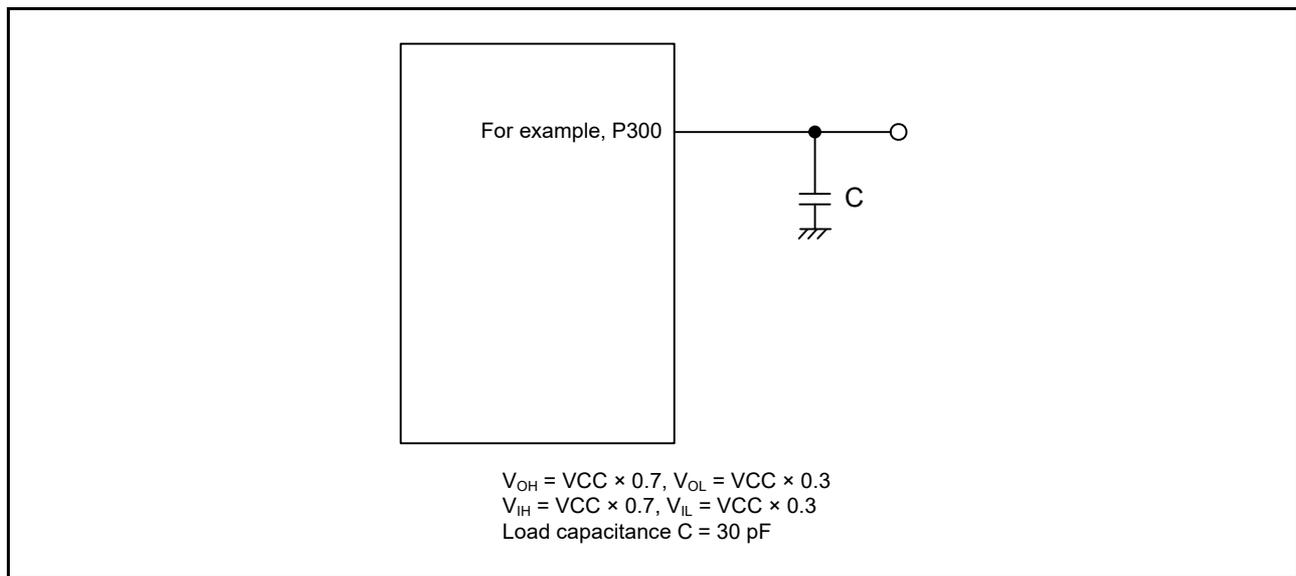
**Figure 2.1** Input or output timing measurement conditions
