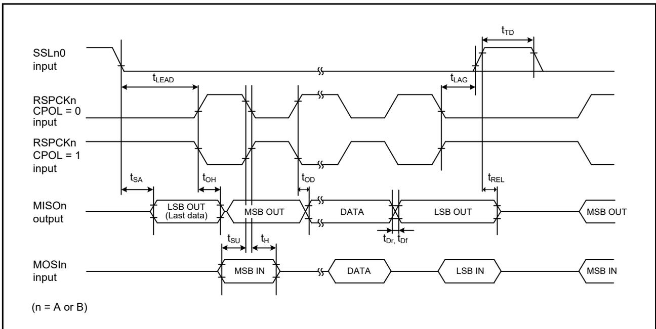
Figure 2.56 SPI timing (slave, CPHA = 1)
