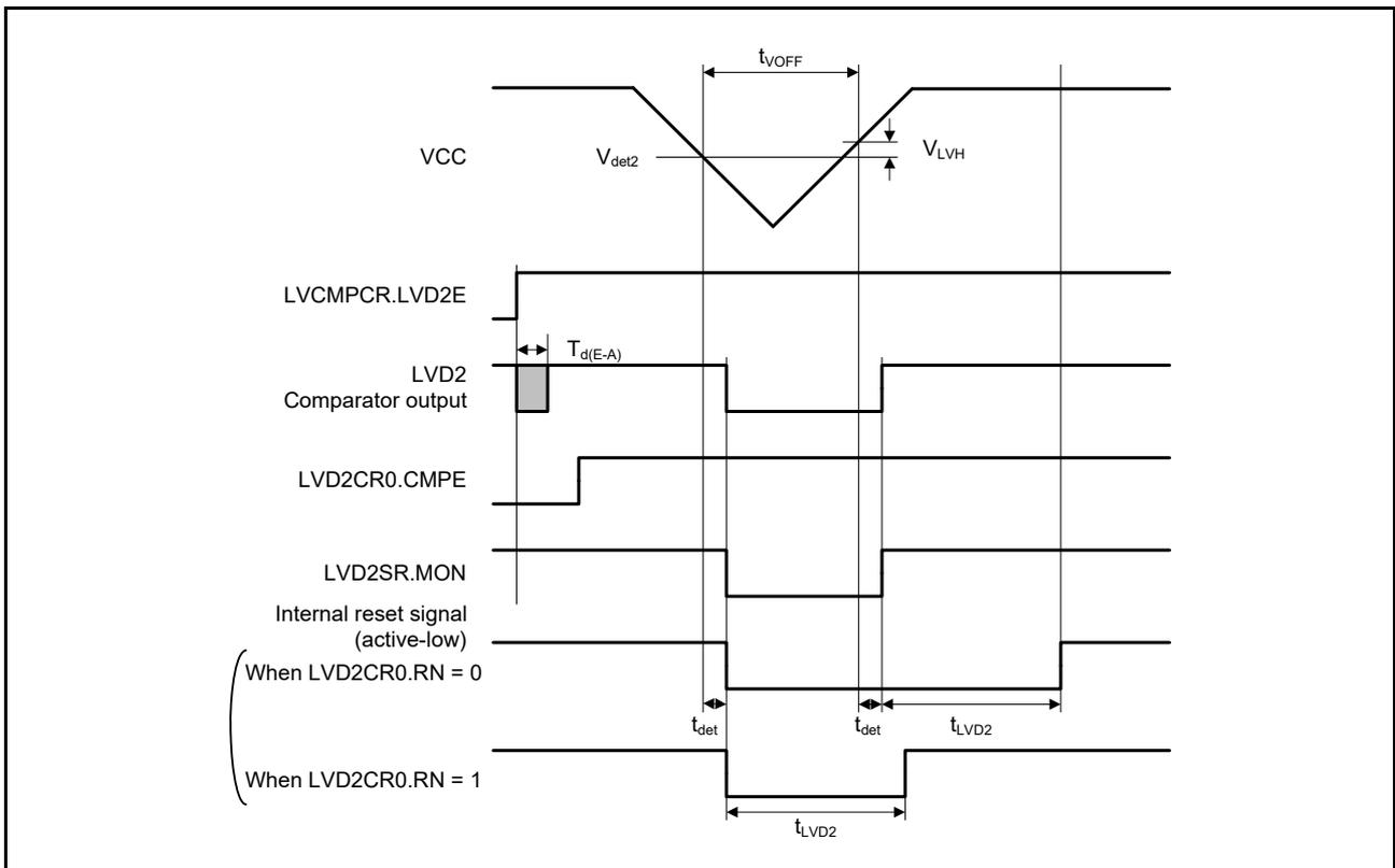
Figure 2.70 Voltage detection circuit timing (V<sub>det2</sub>)
