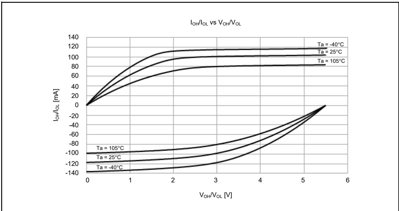
**Figure 2.11**  $V_{OH}/V_{OL}$  and  $I_{OH}/I_{OL}$  temperature characteristics at  $V_{CC} = 5.5$  V when middle drive output is selected (reference data, except for P914 and P915)
