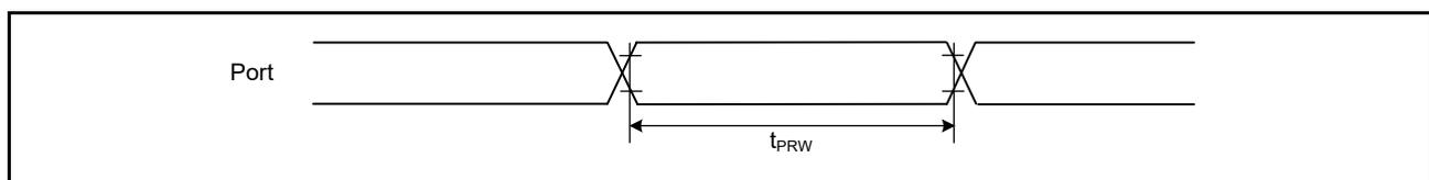
**Figure 2.36 I/O ports input timing**
