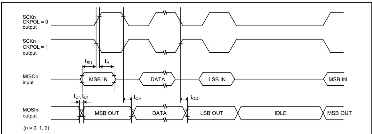
Figure 2.45 SCI simple SPI mode timing (master, CKPH = 1)
