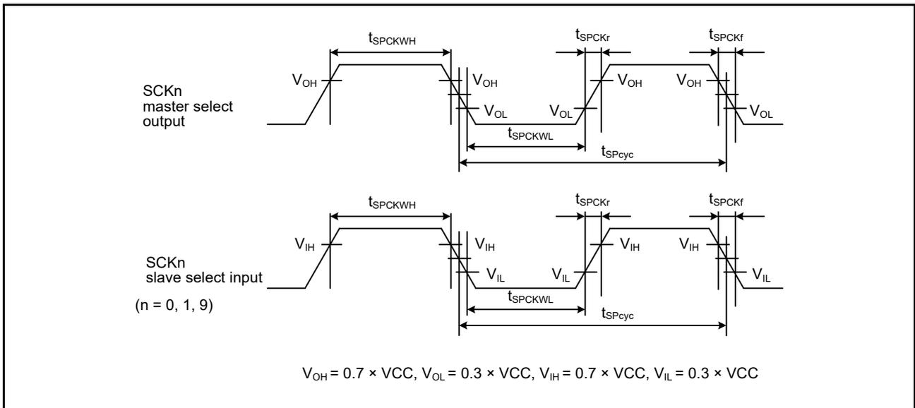
Figure 2.44 SCI simple SPI mode clock timing
