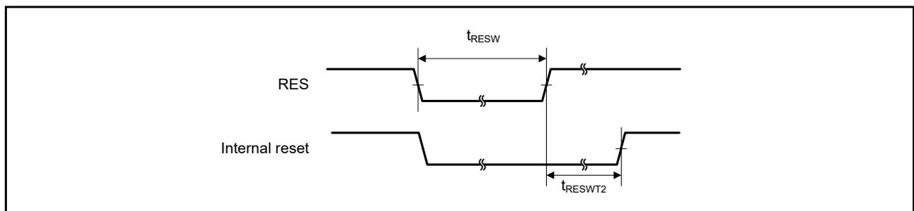
**Figure 2.30 Reset input timing (1)**
