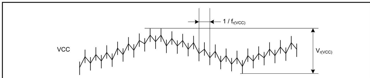
**Figure 2.24 Ripple waveform**
