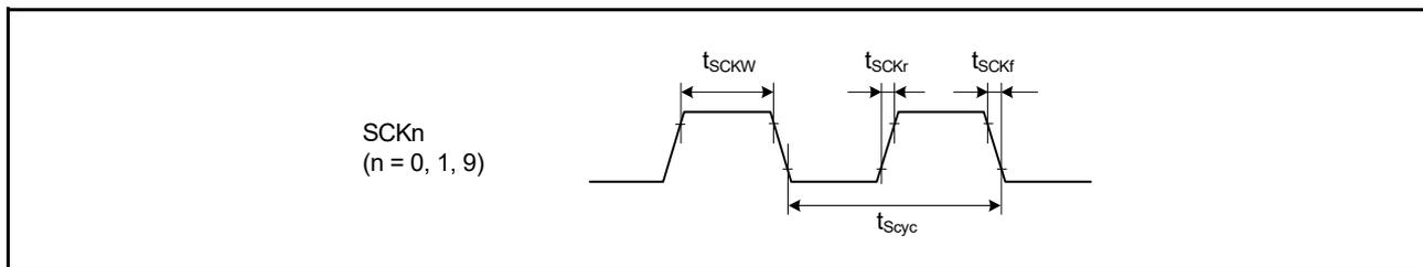
Figure 2.42 SCK clock input timing
