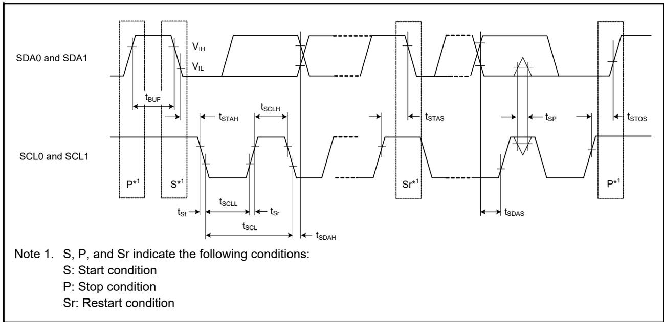
Figure 2.57 I<sup>2</sup>C bus interface input/output timing
