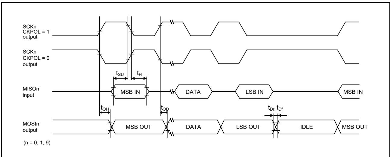
Figure 2.46 SCI simple SPI mode timing (master, CKPH = 0)
