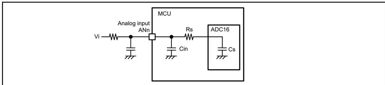
**Figure 2.62 Equivalent circuit for analog input**
