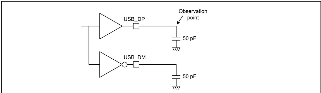
Figure 2.60 Test circuit for Full-Speed (FS) connection
