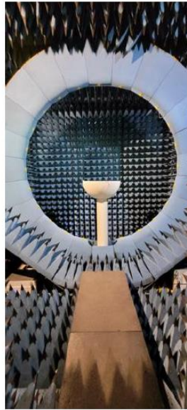
Figure 21. Satimo SG-23 6 GHz Stargate Antenna Test Chamber
